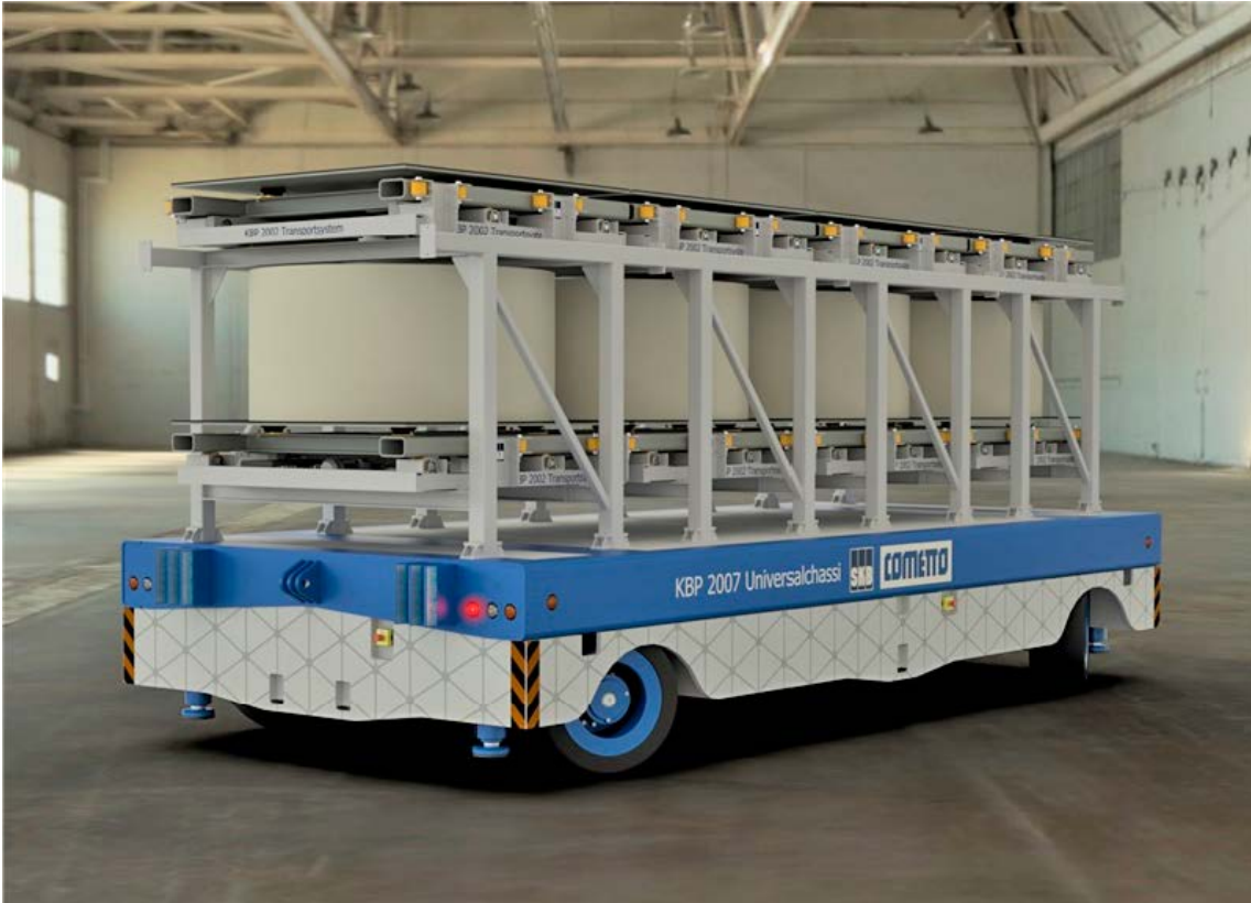
Figure 5-3. Conceptual design of the universal chassis, here it is configured as a material transporter.
