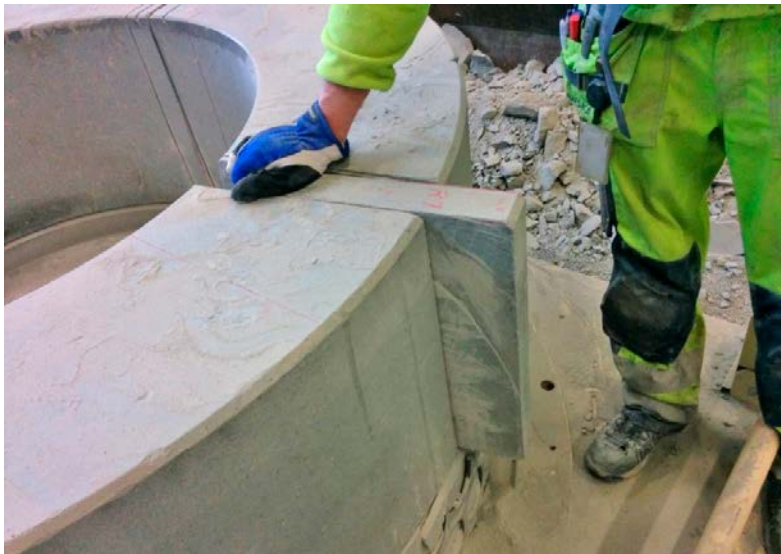
Figure 4-13. Taking samples from the buffer rings.
