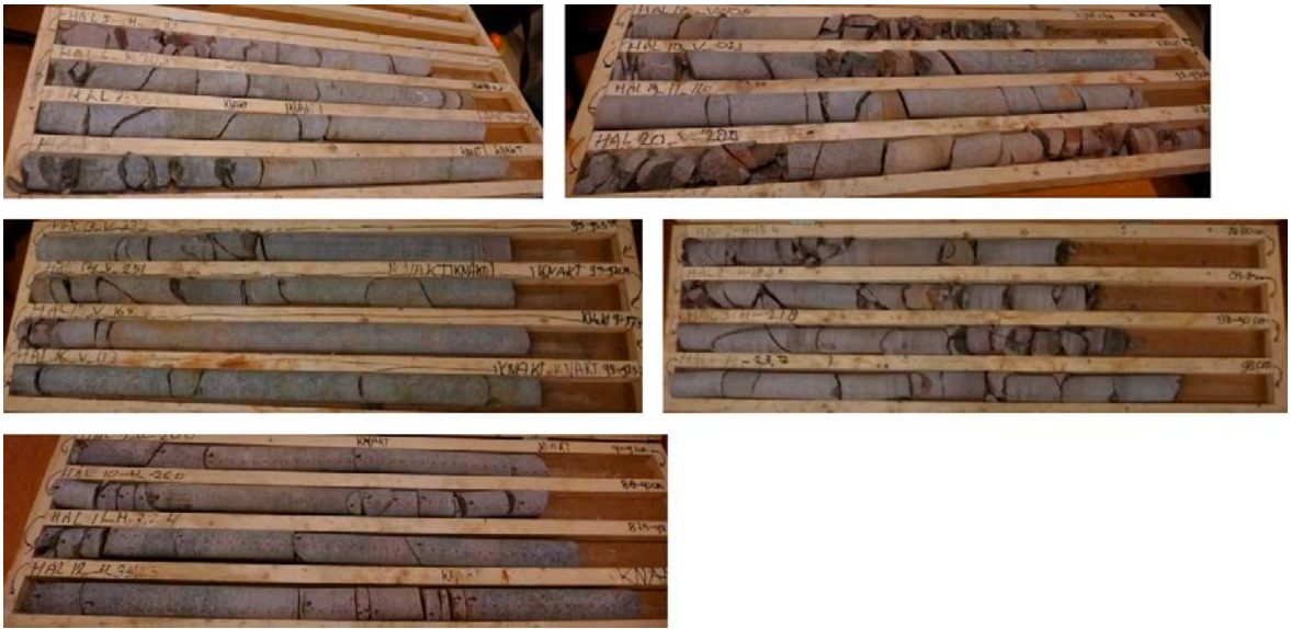
Figure 3-10. Core samples of EDZ investigation taken in TAS04.
