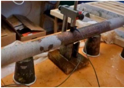
Figure 3-12. Diametric P-wave velocity measurements on TAS04 cores.
