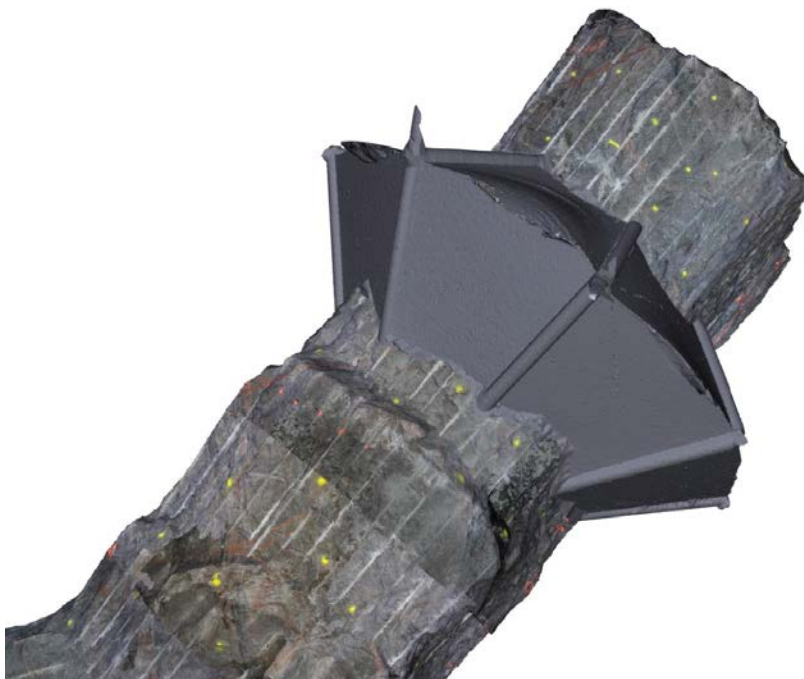
Figure 4-21. Illustrative model structured of data from laser scanning of TAS01 as well as of the excavated slot abutment (seen from above).
