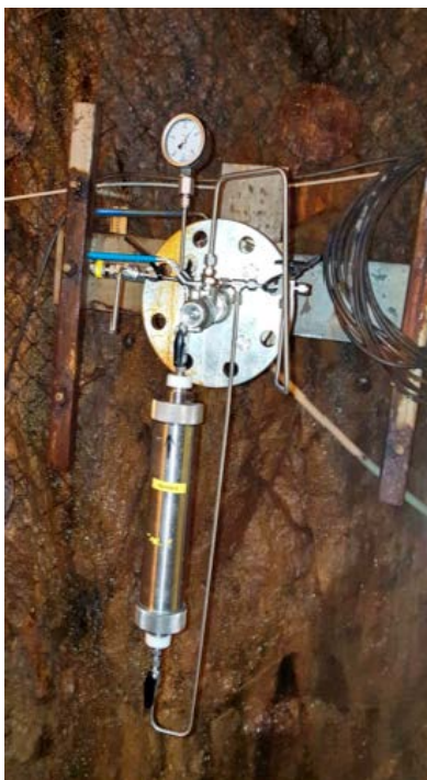
Figure 7-20. Test equipment to expose steel for different groundwater compositions in bedrock.
