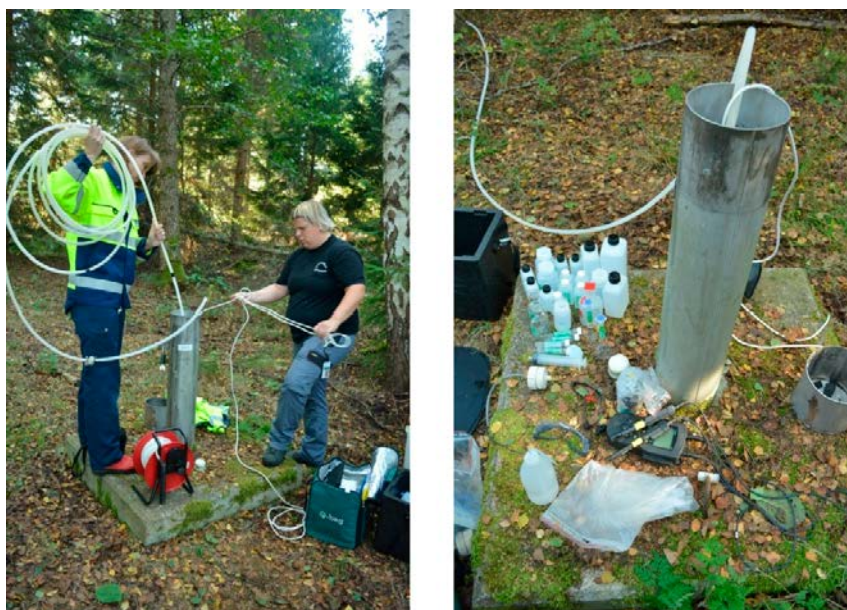
Figure 2-3. Ongoing sampling of shallow boreholes (soil tubes) (left figure), and the equipment such as field instrument and bottles for the extensive analyse program (right figure).
