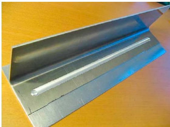
Figure 7-21. Stringer on sheet (aluminum).
