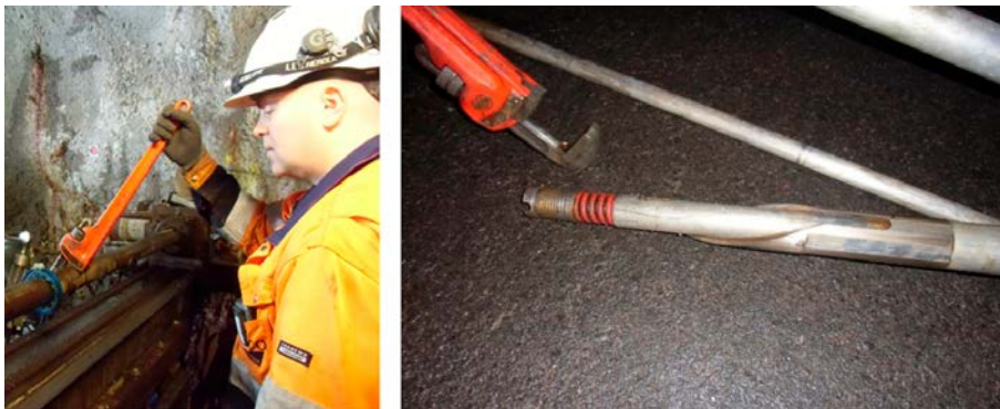
Figure 5-9. Orientation of the DeviDrill tool. The Pee-Wee instrument is mounted inside the DeviDrill when brought into to the bottom of the borehole. A reading is taken and the instrument is winched up and based on the reading may the drill string be rotated to the correct position. Then the inner tube with the Pee-Wee instrument is pumped back into the DeviDrill to check the setting before the steered drilling starts.
