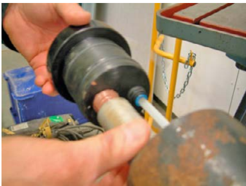
Figure 9-2. The plastic plug glued into the casing destroyed an N drillbit when drilling started. The reason was that the plastic material caulked the water channels, whereby the drillbit was overheated, resulting in melting of the alloy (iron-cobalt) with which the diamond chips are fastened to the drill bit body.
