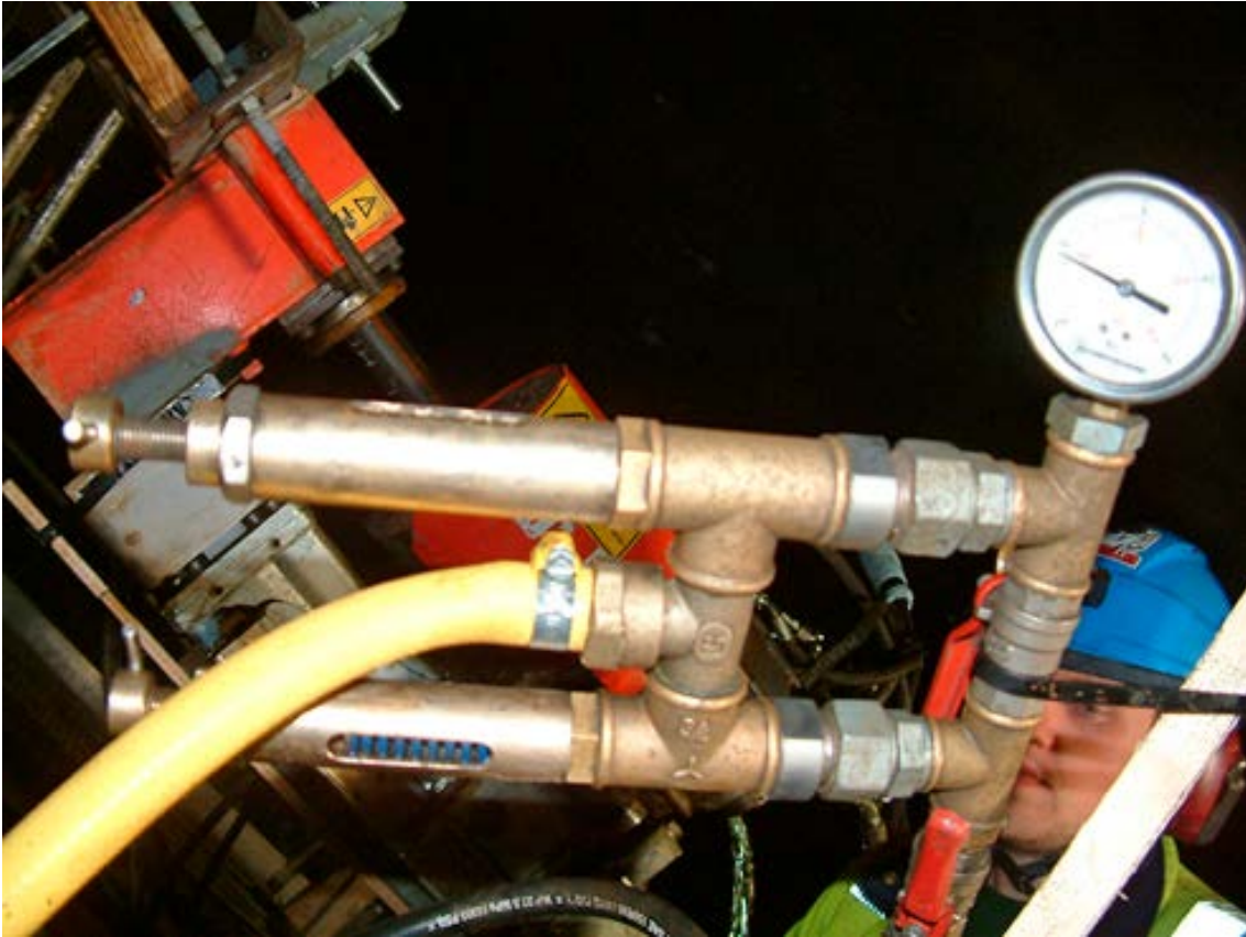
Figure 7-9. An adjustable reducing valve is mounted on the hose from the flush water pump preventing the water pressure to drop below 30 bars while the DeviDrill is in use.
