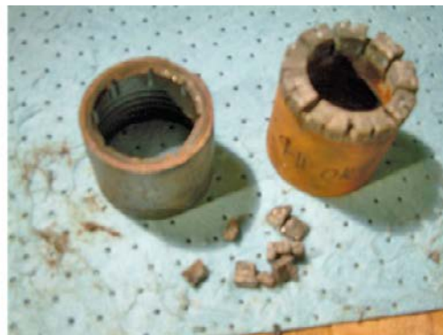
Figure 9-2. The plastic plug glued into the casing destroyed an N drillbit when drilling started. The reason was that the plastic material caulked the water channels, whereby the drillbit was overheated, resulting in melting of the alloy (iron-cobalt) with which the diamond chips are fastened to the drill bit body.
