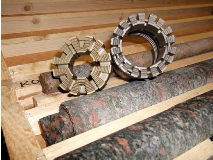
Figure 8-2. Display of drill bits and example core. Conventional triple-tube drilling 76 mm (N-size) gives a core diameter of 50.8 mm (right). When using the directional core barrel a core with 31.5 mm diameter is produced (left).
