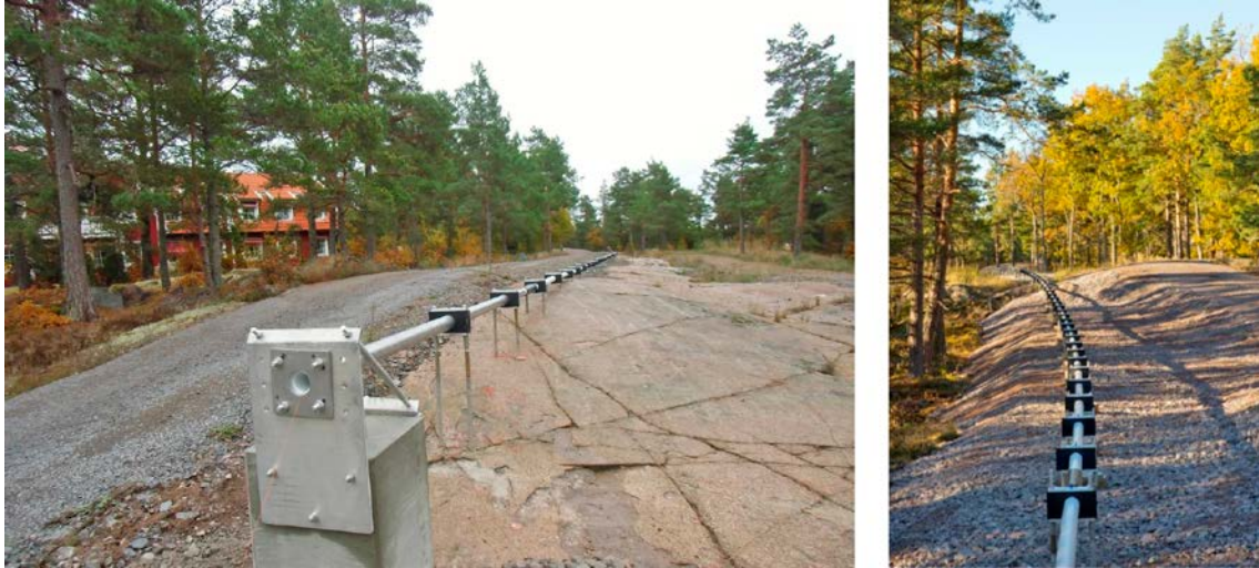
Figure 4-1. Äspö deviation control facility is a 300 m long plastic tube ( \text{Ø}75 mm) secured firmly to the ground with 151 fastening devices. All material used in the construction is non-magnetic such as plastic and aluminum.
