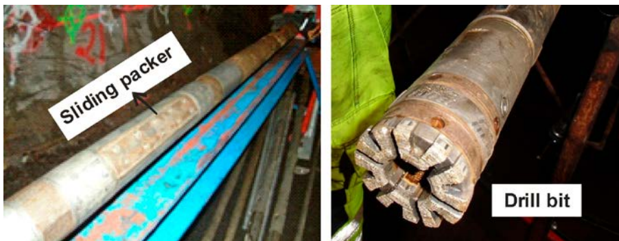
Figure 5-8. DeviDrill core barrel. Left: When water pressure increases (about 20 bars), the sliding packer expands and locks the barrel in its position. Right: The end of the DeviDrill. The drill bit gives a 31.5 mm core in sections where steering is applied.
