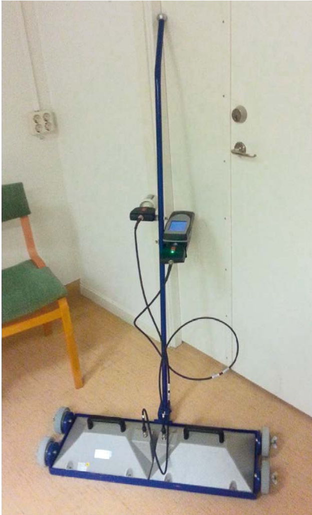
Figure B-5. Measurement device with room for two DP8 scintillation detectors installed for scanning measurement of floor surfaces. Measurement data from both probes are collected in a Colibri measurement data file.
