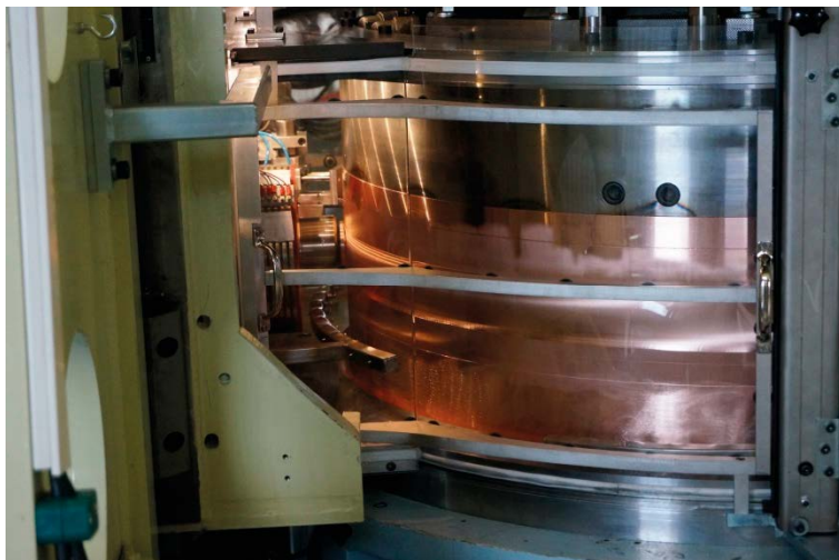
Figure 2-3. The gas shield during welding. To the right, the supporting bracket can be seen. The white lines on the upper and lower part of the PMMA panels are seals.
