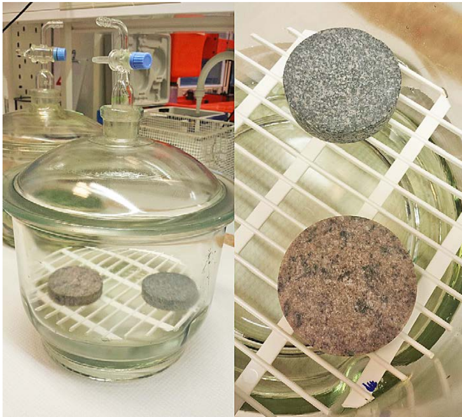
Figure 3-56. Excicator (with saturated salt solution) and two rock samples, B1 and A1.
