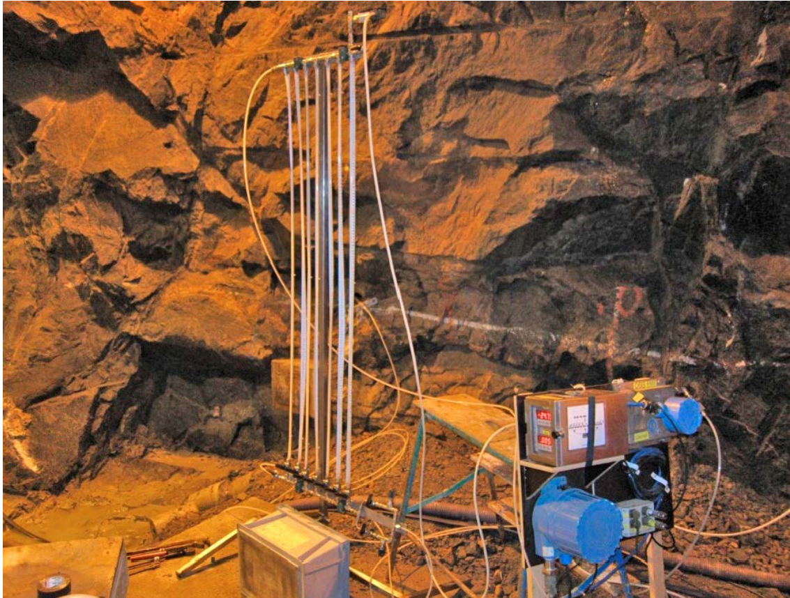
Figure 3-10. Photo of equipment referred to as a “flow organ” used for transient hydraulic tests. See also principal sketch in Figure 3-11. Using this equipment, water level drawdown in tubes could be read manually and based on this flow was calculated.
