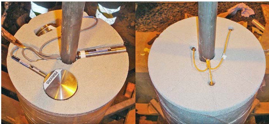
Figure 4-8. Instrumentation of blocks; left: block with pressures sensors; right: block with RH sensors.
