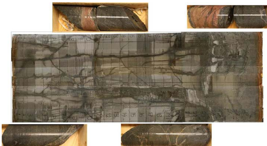
Figure 5-18. Comparison of some fractures in rock core and traces on bentonite for KO0018G01. The core is broken by the main water-bearing fracture.
