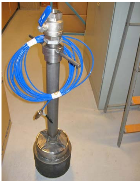
Figure 3-41. Single packer for hydraulic testing in 300 mm boreholes.
