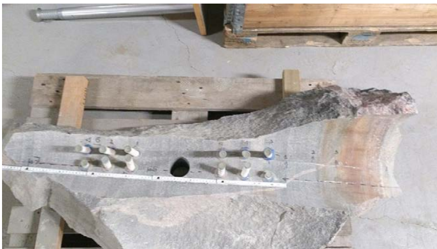
Figure 3-64. Rock blocks and monitoring of relative humidity (RH), KO0017G01 (upper part of rock block to the right). Locations referred to as DSL (Dry Section Lower) and F (closest to the Fracture). The figure also shows the location of the rock core for hydraulic tests. Samples 1:1 to 1:4 (hydraulic conductivity) originate from the core. Figure 5-25 shows location of measurements in rock in relation to the bentonite parcels.
