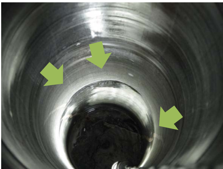
Figure 5-4. Location of main flows (green arrows) in main water-bearing fracture, KO0017G01. The arrows indicate the upper part of the fracture (opposite the dip-direction).
