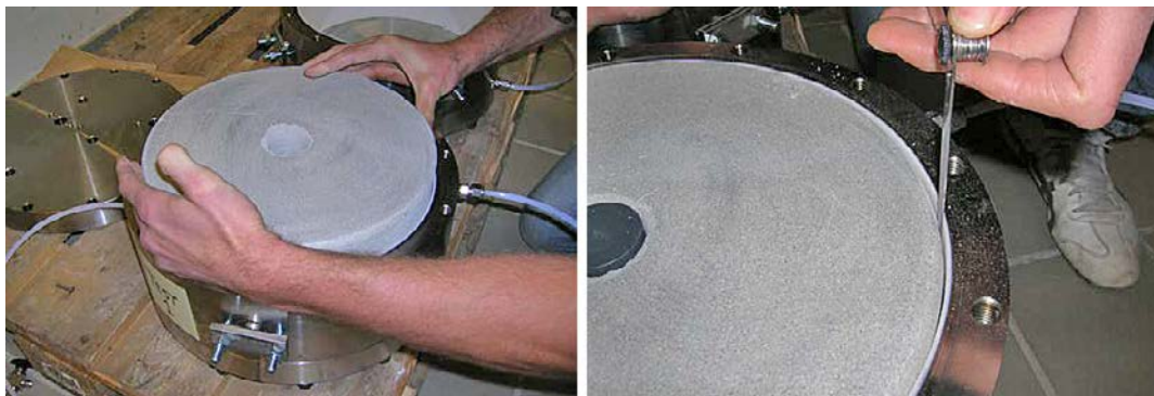
Figure F-6. Installation of block in cylinder (left). Centering of block (right). The PVC dummy representing the central tube is seen to the left of the right picture.
