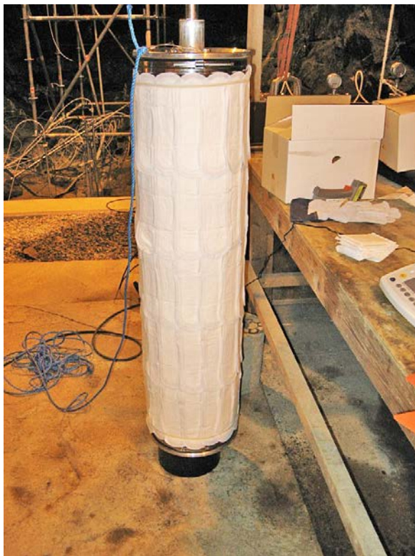
Figure 3-46. Equipment for borehole wall inflow measurements, also referred to as a “Nappy” test. The equipment consists of a cylinder of approximately 1 m length and 0.3 m diameter covered by rubber that can be inflated using gas pressure to fit the borehole. Nappies (15 around and 5 in height) were attached to the cylinder to measure the flow distribution over the borehole surface. Photo Christian Butron.
