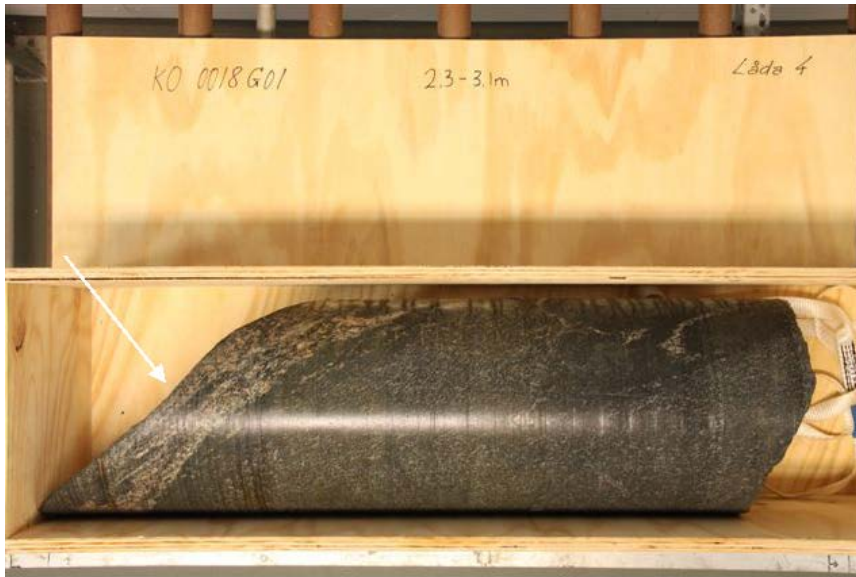
Figure 3-40. KO0018G01, 2.3–3.1 m, 300 mm. Main fracture of interest is indicated (deepest part of the core).
