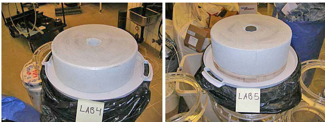
Figure F-3. Two bentonite blocks ready for installation.
