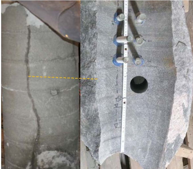
Figure 5-19. Dark trace on surface of Blocks 10–15 in KO0017G01 and corresponding fracture between rock blocks (image reversed). Note the main fracture of interest, and the trace from this, at the lower end of the photos.
