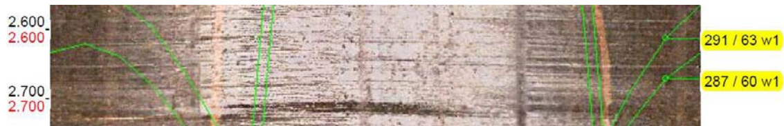
Figure A-10. KO0017G01, Strike/dip (bold style in Table A-3) relate to (one of the two) fracture(s) found from 2.6 m to 3.1 m.
