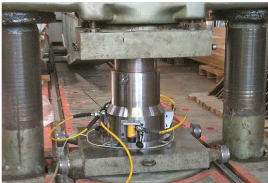
Figure F-2. Form for compaction of bentonite blocks.
