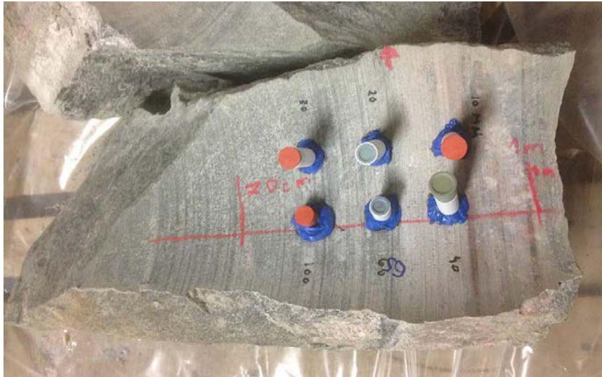
Figure 3-65. Rock block and monitoring of relative humidity (RH), KO0018G01, upper part of rock block to the right.
