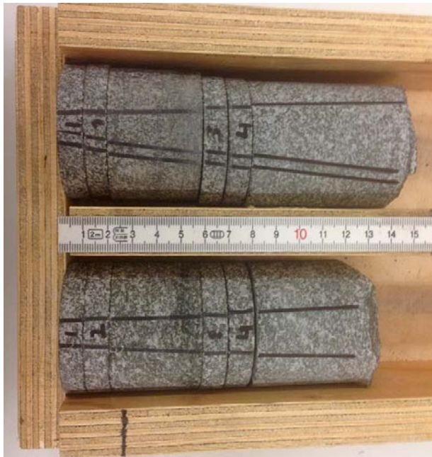
Figure 3-66. Boreholes perpendicular to KO0017G01, in rock blocks by the 300 mm borehole wall. Left (three lines) includes samples 2:1 to 2:4 (Dry Section Upper, 26.5 cm above fracture). Right (two lines) includes samples 1:1 to 1:4 (between Dry Section Lower, DSL and F). Samples 1:1 and 2:1 are found closest to the borehole wall. Approximate distance due to material lost during preparation of samples.
