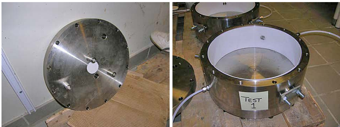
Figure F-4. Lid with holders for RH-sensors, and filter for gas pressure sensor (left). Cylinder with filter, water inlets and force transducers with pistons (right).
