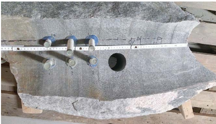
Figure 3-63. Rock block and monitoring of relative humidity (RH), KO0017G01 (upper part of rock block to the left, right hand of photo shows the upper part of main fracture). The figure also shows the location of the rock core for hydraulic tests. Location referred to as DSU (dry section upper). Samples 2:1 to 2:4 (hydraulic conductivity) originate from the core. Figure 5-24 shows location of measurements in rock in relation to the bentonite parcels.
