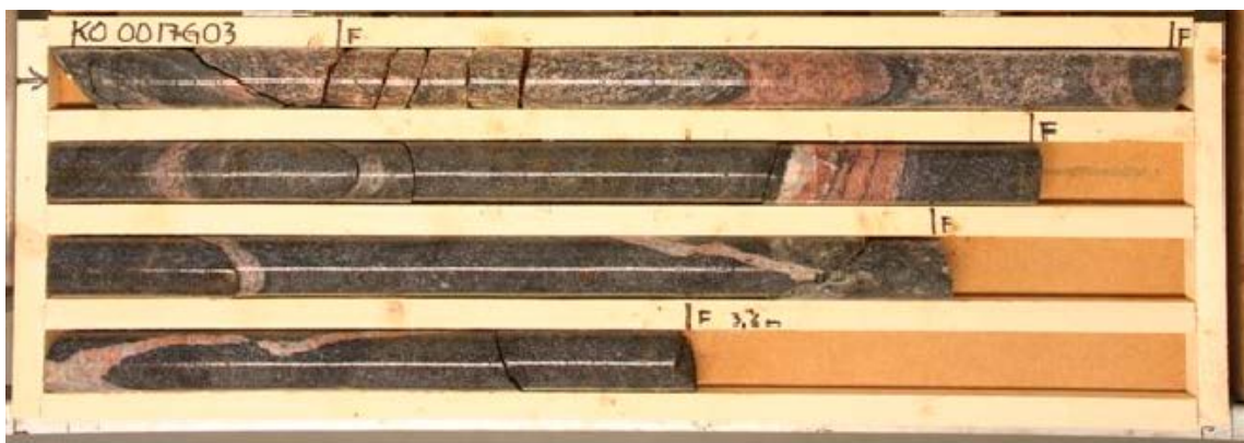
Figure 3-24. Core from borehole KO0017G03. Fracture of main interest in the lower part of the borehole identified with the pegmatite vein (that has been subjected to shearing).
