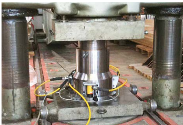
Figure 4-6. Form for compaction of bentonite blocks.
