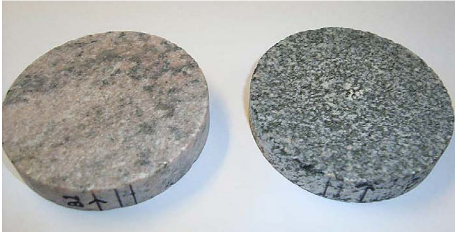
Figure 3-58. Samples B2 (fine-grained granite) and A2 (diorite), KO0020G01, diameter and thickness approximately 60 mm and 10 mm respectively.
