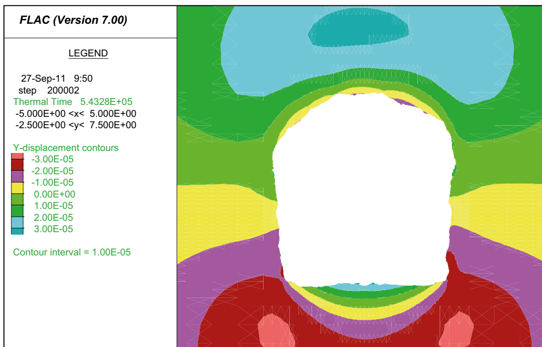
Figure A1-9. Magnitudes of elastic displacements in the y-direction due to 6 days of heating for the section 42 m.
