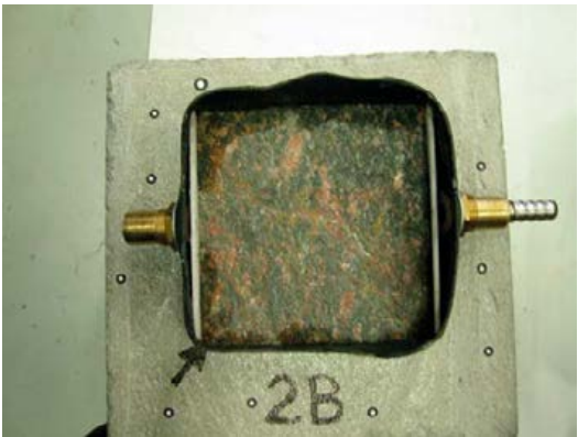
Figure 2-12. Sample, rubber tube, filters and quick joints for water inlet and outlet.
