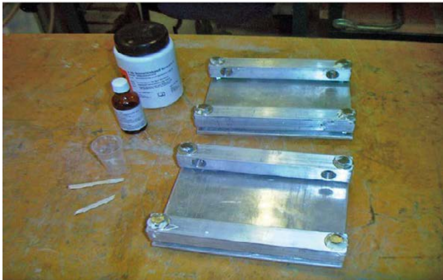
Figure 2-7. The fixation tools for mounting the LVDTs along the side of the samples.
