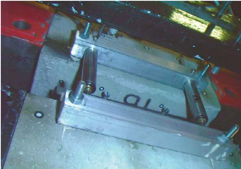
Figure 2-9. LVDTs mounted into the holders after the guide aluminium plate has been removed.
