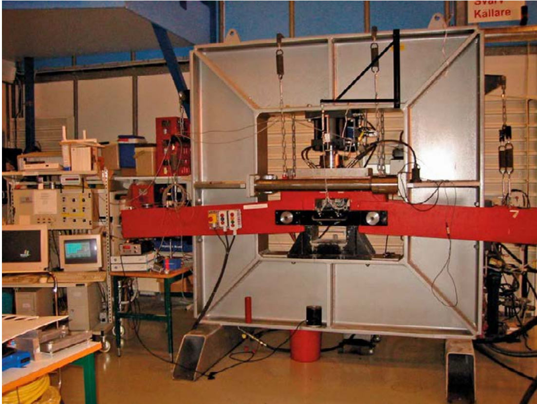
Figure 2-2. Shearing frame in grey with shearing system in red. Log system in the right of the picture.
