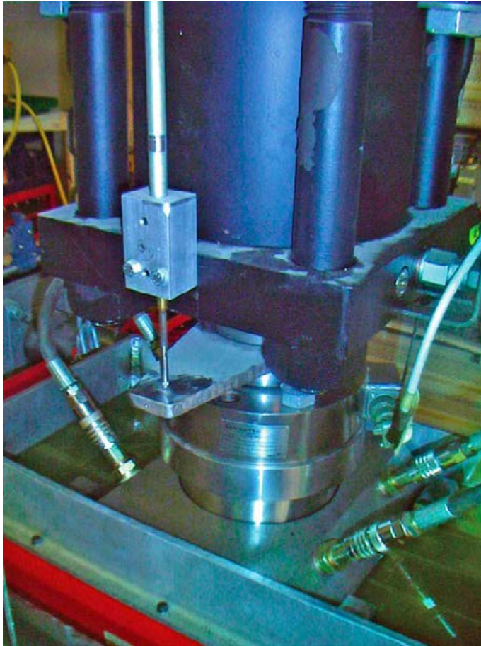
Figure 2-5. Normal force actuator and the system for distributing the force down on top of the sample.
