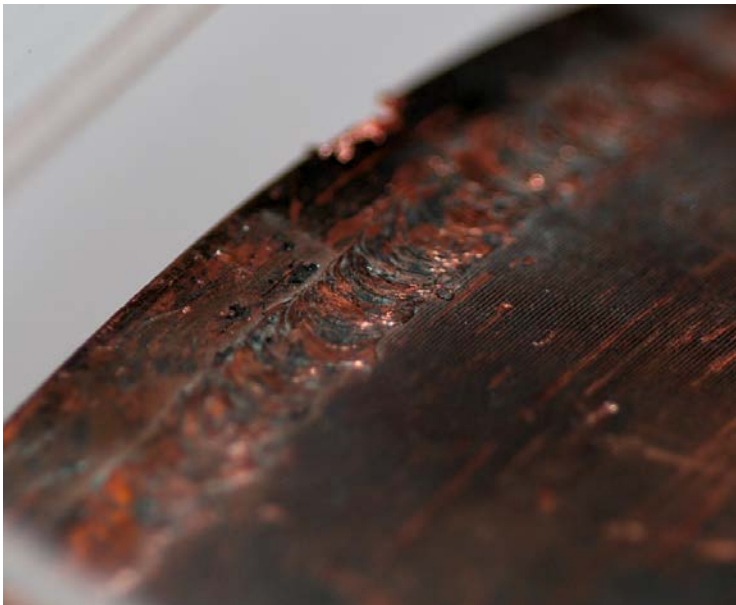
Figure 4-50. Top weld of copper canister sample M5 26:1.
