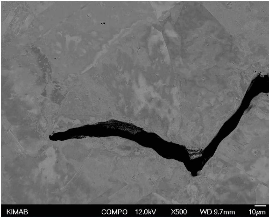
Figure A3-62. Crack tip of WOL sample M4 4:1.
