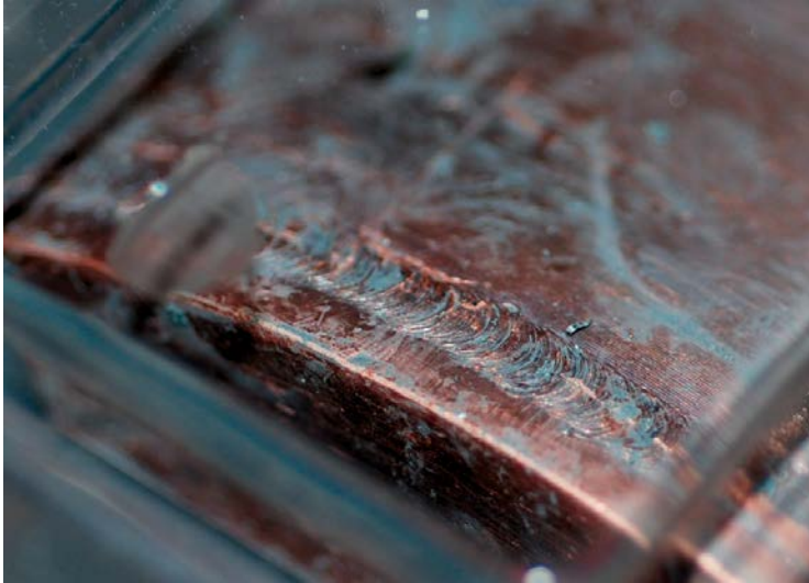
Figure 4-49. Top weld of copper canister sample M4 26:1.
