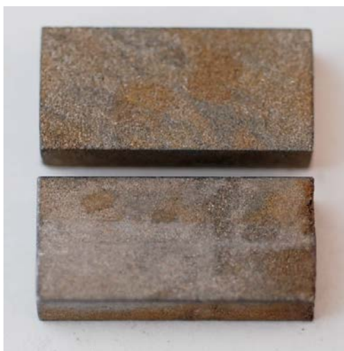
Figure 4-22. Iron mass loss samples M4 11:1 and M5 11:1 after pickling.
