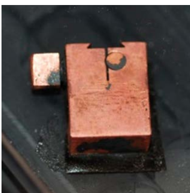
Figure A7-23. Sample M4 2:1 u-bend specimen, with fluorescence from cuprite.
