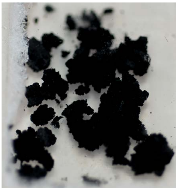
Figure 4-63. Sample M5 13:1 corrosion products from the iron part of the iron-copper sandwich.
