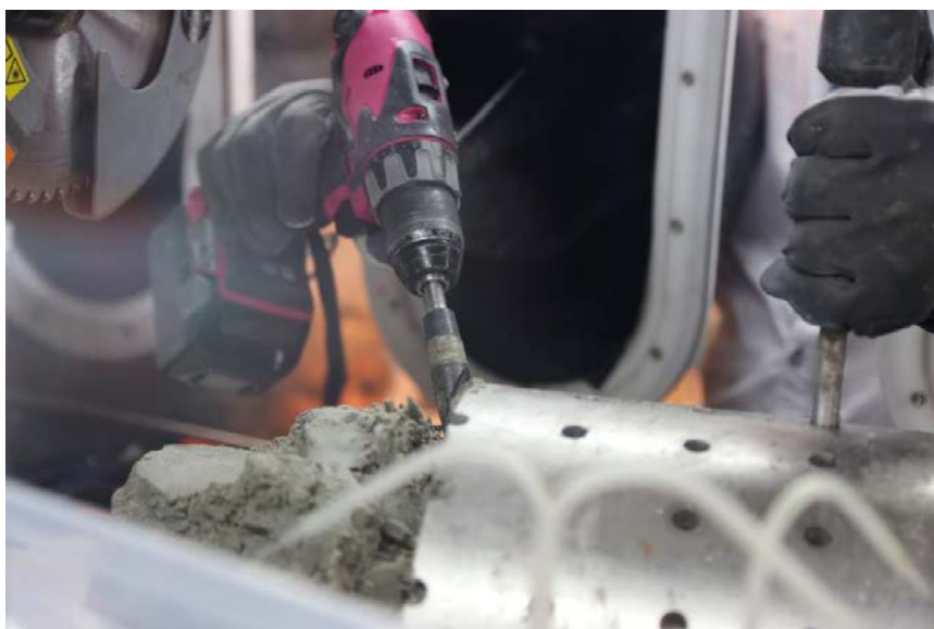
Figure 2-5. The stainless steel cage was cut open and the bentonite was removed as much as possible by use of hand tools.
