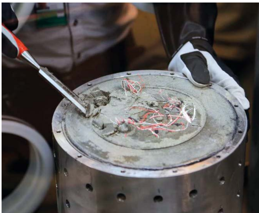
Figure 2-4. The high-density bentonite as seen upon opening the MiniCan 4 assembly.
