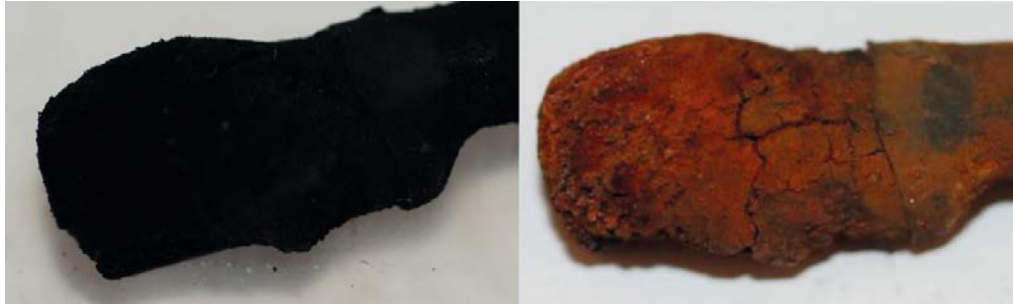
Figure 4-18. Sample M5 9:1 iron electrode before and after a few minutes of exposure to air after the sealed sample holder was opened.
