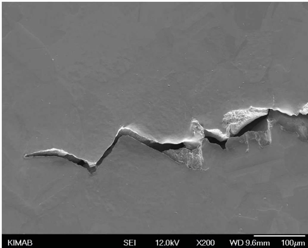
Figure A3-65. Secondary electron image (SEI) of forward part of pre-crack of WOL sample M4 4:1.
