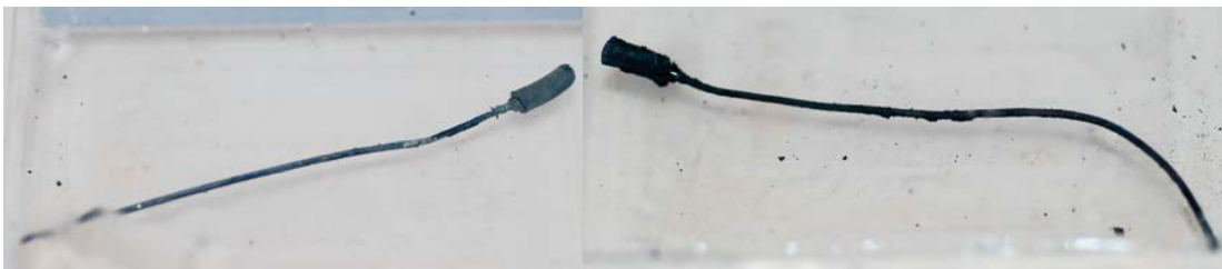
Figure 4-36. M5 16:1 and 17:1 Pt and Au electrodes.
