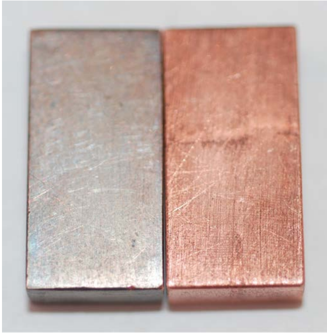
Figure A4-2. Copper mass loss sample M4 7:1 on the left hand side, and M5 7:1 on the right hand side, after pickling was completed. M4 7:1 was grey in colour after pickling.
