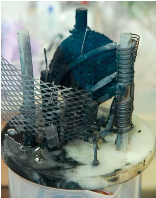
Figure 5-2. The support table upside down immediately after removal from MiniCan 5. The copper mass loss (left) and iron mass loss (right) samples can be seen in the foreground attached to the Pt/Ti net electrode by a nylon thread. The black surface deposit can be seen to be confined to the sandwich specimen and one half of the support rack.
