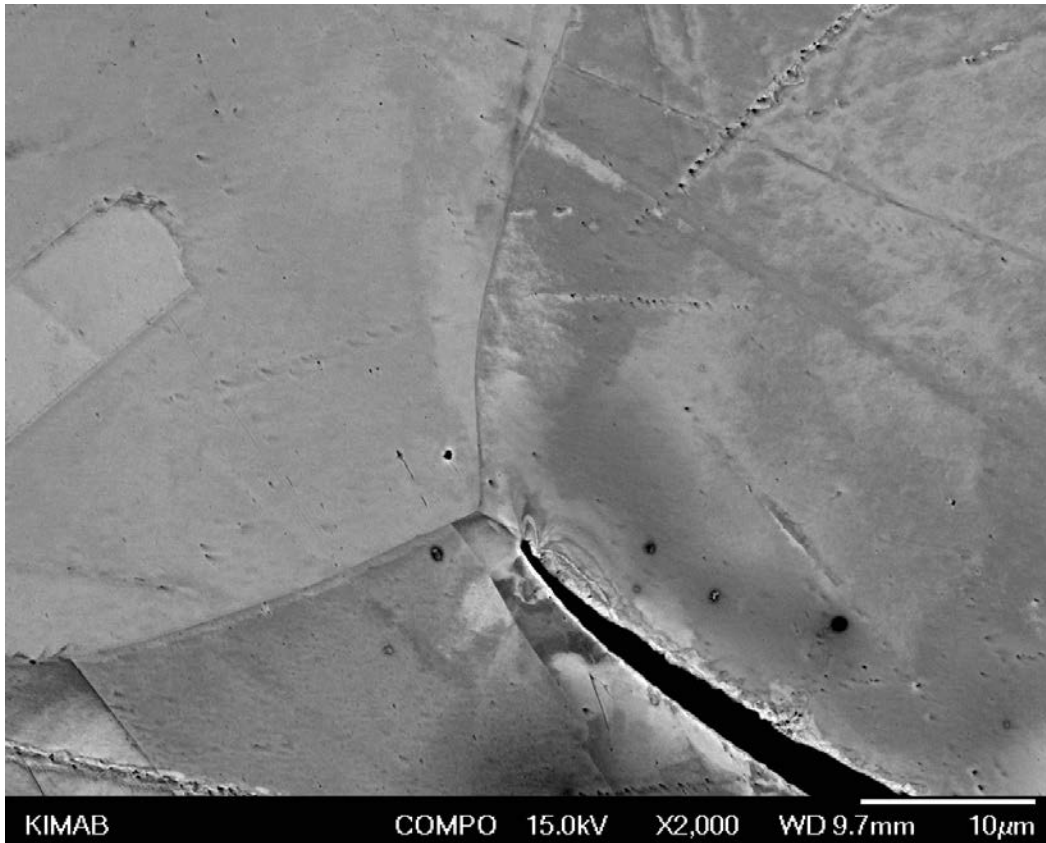
Figure A3-46. Detail of the crack tip of WOL sample M4 3:1.
