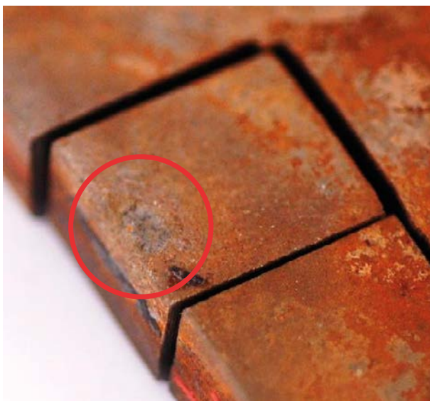
Figure 4-58. Cast iron insert sample M4 30:1 after removal from the sample holder and after further sampling had taken place to cut out the corroded area, encircled, for analysis.
