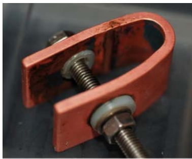
Figure A7-22. Sample M4 1:1 u-bend specimen.
