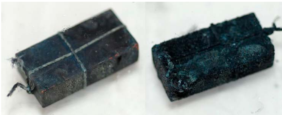
Figure 4-21. M5 7:1 and M5 11:1 copper (left) and iron (right) mass loss samples after removal from the MiniCan 5 experiment.
