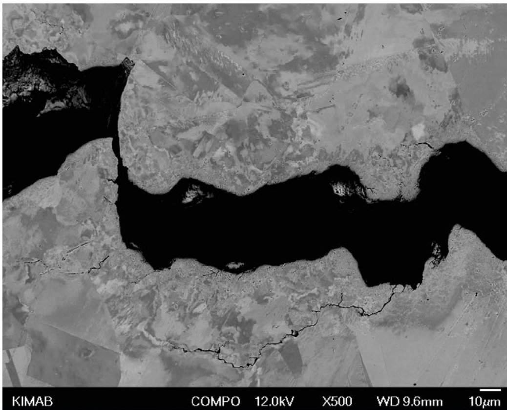
Figure A3-63. Detail of middle section of pre-crack of WOL sample M4 4:1, with smaller cracks emanating from the pre-crack into the cold deformed zone.
