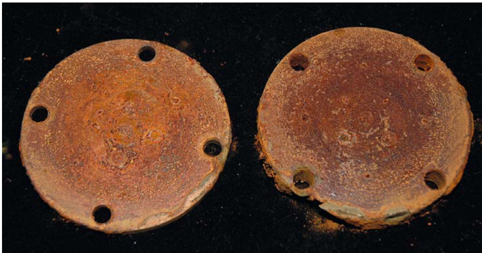
Figure 4-29. Inner surfaces of sample M5 14:1 sandwich specimen, copper on the left, iron on the right. The internal surfaces of the components were covered with iron corrosion products. The iron component had significant material loss as seen on the bottom left hand corner of the iron specimen to the right. The shiny area on the bottom right of the copper sample is the mating surface to the corroded area of the iron sample.
