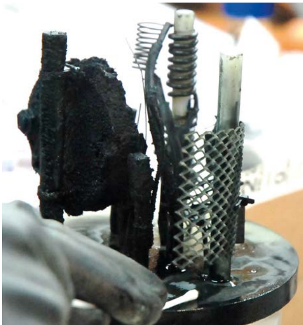
Figure 4-27. Copper-Iron sandwich sample M5 14:1 seen on the left hand side of the figure, directly after withdrawal from the MiniCan assembly. The outer surfaces are covered in a thick black deposit which also covers the adjacent areas of the support table.
