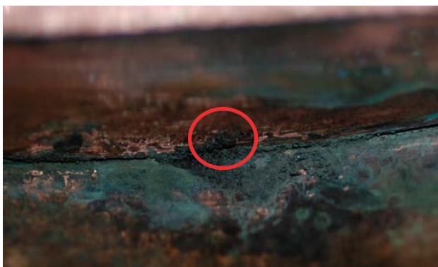
Figure 4-5. Sample M5 27:1 hole through copper canister at top of MiniCan 5.
