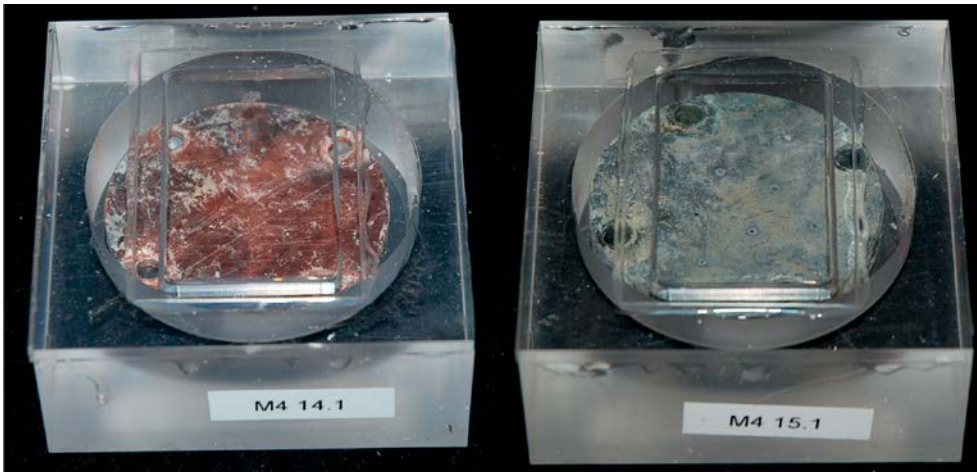
Figure 4-25. Copper (M4 14:1) and iron (M4 15:1) parts of the sandwich specimen after removal from MiniCan 4.
