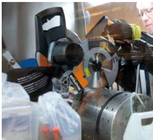
Figure 2-3. The modified circle saw assembly, with two saws installed on the customised base.
