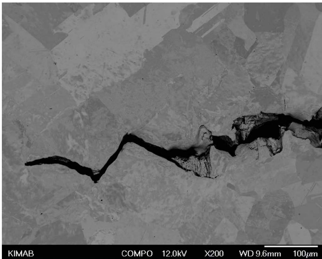
Figure A3-61. Forward part of the pre-crack of WOL sample M4 4:1.
