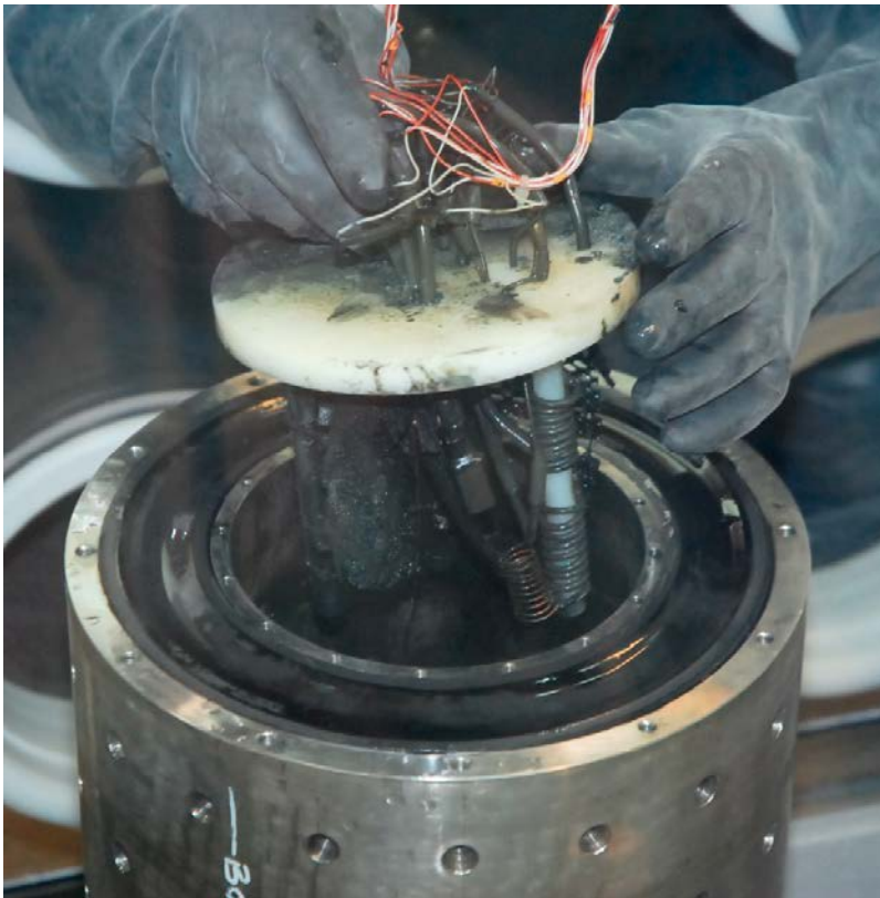
Figure 2-8. Removal of the "external" samples from inside the MiniCan 5 assembly.
