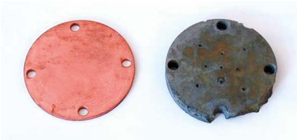
Figure 4-31. The inner surfaces of M5 14:1 sandwich specimen after pickling. The copper component is visibly uncorroded, whilst the iron component does not appear to be as corroded compared to the outer surface. The edges of the iron component are corroded however, and these correspond to contact points with the copper component when assembled.
