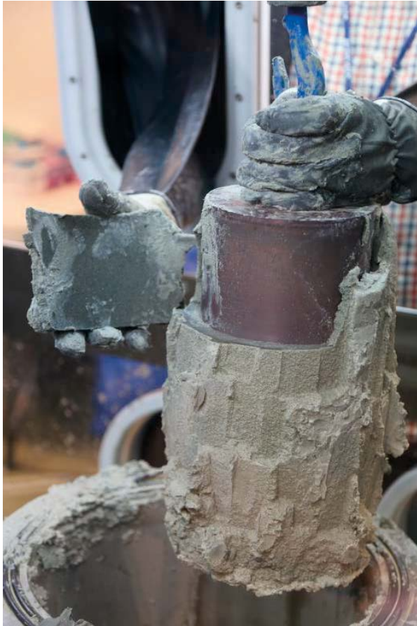
Figure 2-6. Removal of the final layers of bentonite surrounding MiniCan 4.
