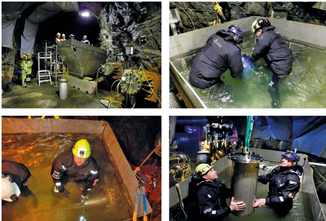
Figure 2-1. a) top-left: water-filler container connected to borehole; b) top-right: SKB personnel removing the MiniCan assembly; c) bottom-left: the MiniCan assembly remained under water at all times during removal; d) bottom-right: a sealed transfer flask was used to keep the MiniCan assembly oxygen-free until it was placed inside the glovebox.
