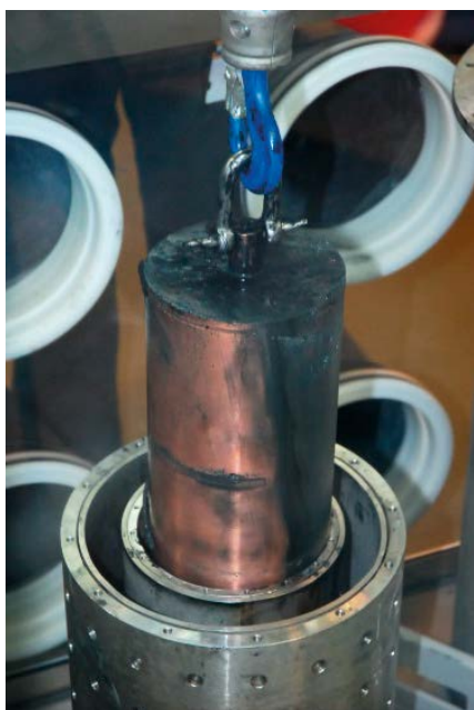
Figure 2-2. MiniCan 5 being lifted out of the stainless steel cage. The black deposit on the right hand side in the photograph was the bottom of the MiniCan, positioned downwards in the borehole.
