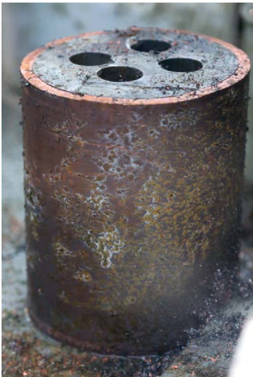
Figure A2-6. Bottom section of sectioned MiniCan 4, iron particles contaminated the surface during cutting and began to oxidise on the surface after the glovebox was opened.
