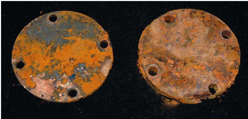
Figure 4-28. External surfaces of sample M5 14:1 sandwich specimen, copper on the left, iron on the right. The external surfaces of both components were covered with a thick deposit consisting mainly of iron corrosion products. The iron specimen had significant material loss after the exposure, seen here at the 6 o'clock and 10 o'clock positions.
