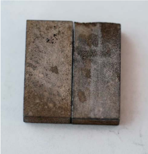
Figure A4-5. Iron mass loss samples, M4 11:1 to the left hand side, and M5 11:1 after pickling was completed.
