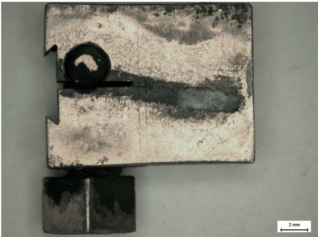
Figure A3-57. Microscope image of opposite side of WOL sample M4 4:1.
