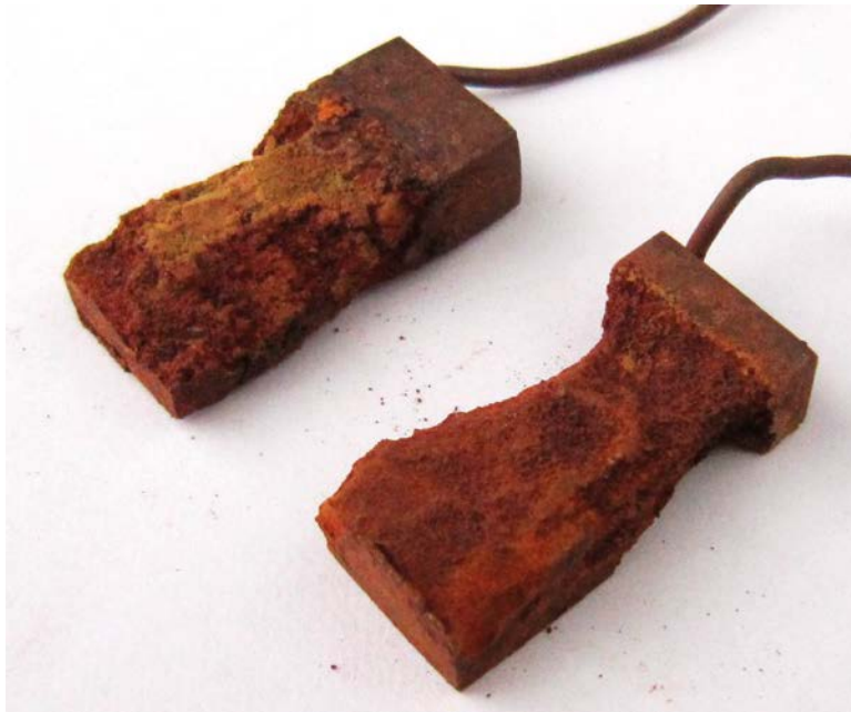
Figure 4-19. Appearance of iron electrodes M5 9:1 (left hand side) and M5 10:1 from MiniCan 5 after removal of loose corrosion products. The uncorroded areas near the electrical connection were protected by heat shrink during the exposure period.
