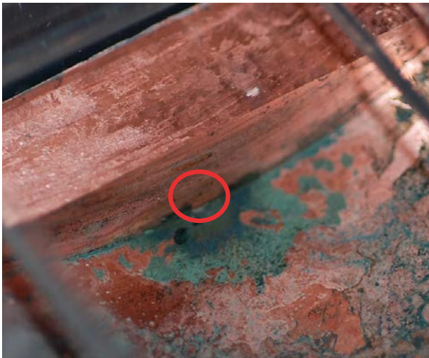
Figure 4-53. Sample M4 27:1 hole through copper canister, inner surface. The hole is located at edge between perpendicular surfaces as marked by the red circle.
