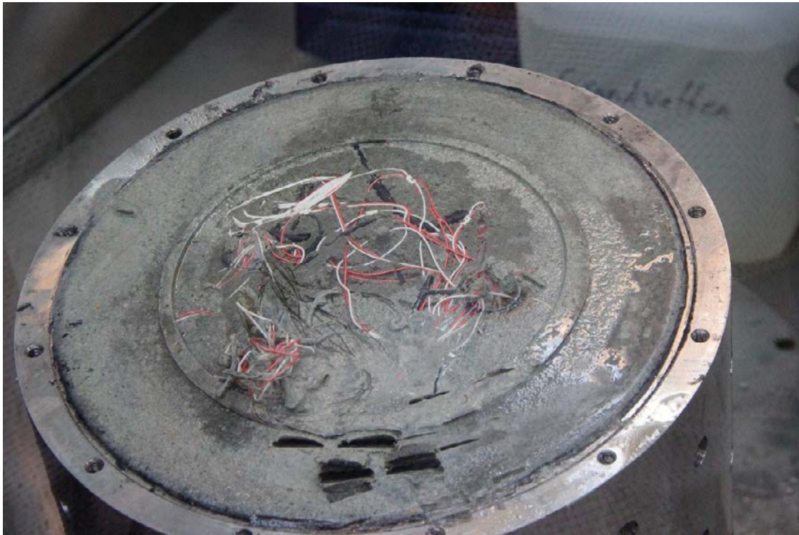
Figure 2-9. The top of the A05 support cage from MiniCan with fully compacted bentonite.
