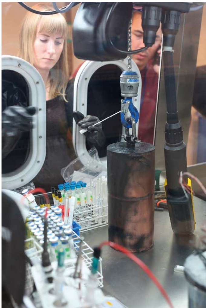
Figure 2-6. Sampling from the A06 copper canister from the MiniCan project, inside the glove box.
