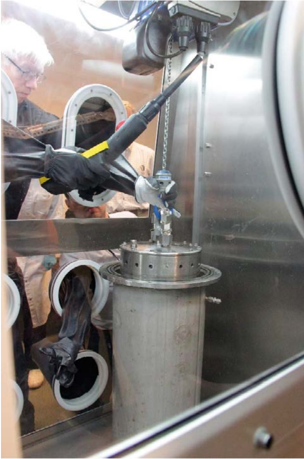
Figure 2-1. Transfer of the support cage of the MiniCan package A06, from the transport cylinder inside an anaerobic glovebox.
