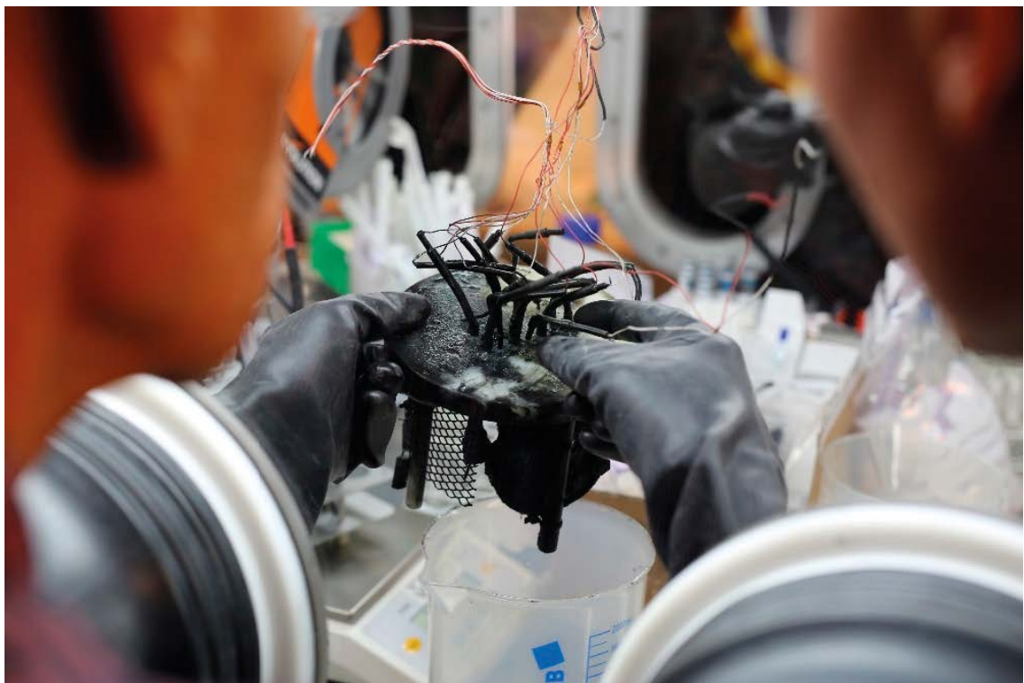
Figure 2-4. The nylon support rack and test specimens from the MiniCan package A06.
