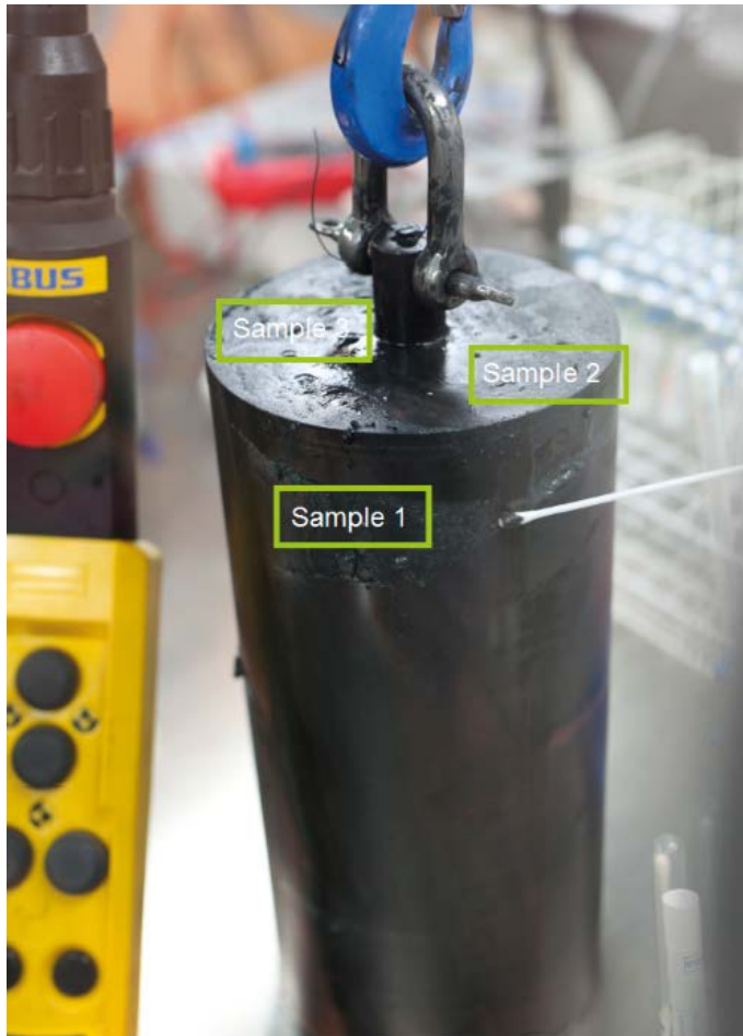
Figure 2-7. Sampling for microbiological analysis from the copper canister surface of the MiniCan package A06. The text squares show where the three canister samples were taken.
