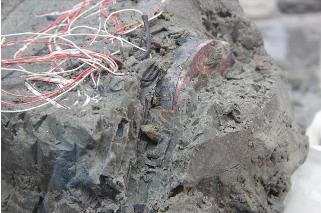
Figure 2-14. The sandwich specimen in compacted bentonite from the A05 package in MiniCan.
