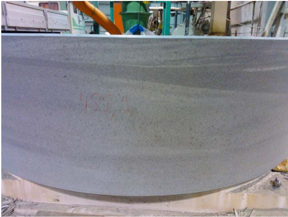
Figure 2-1. striping in compacted blocks.
