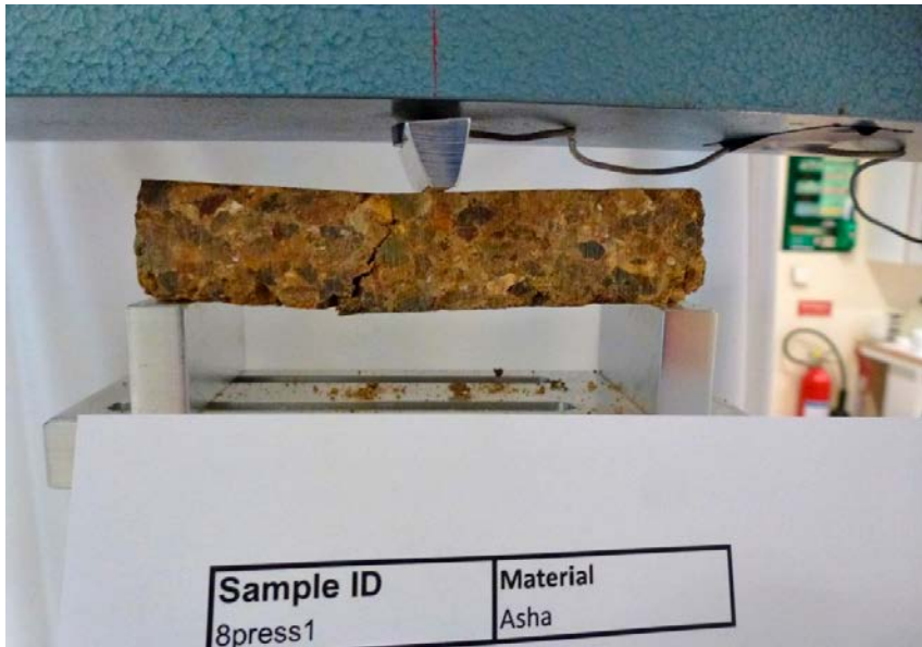
Figure 3-5. Example of a test sample with a coarse fraction. The failure surface is not in the centre and tend to follow the granule boundaries.
