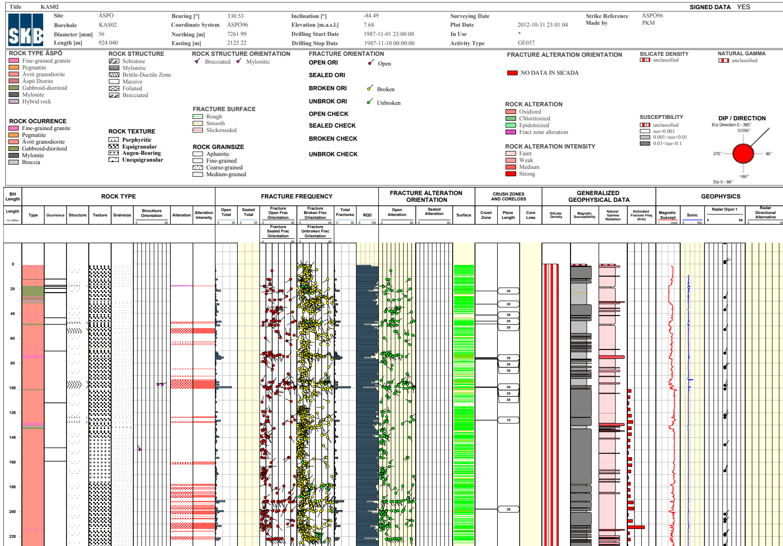
Figure 2-1. Example of WellCAD plot (from borehole KAS02 at Äspö) used as a basis for the geological single-hole interpretation.
