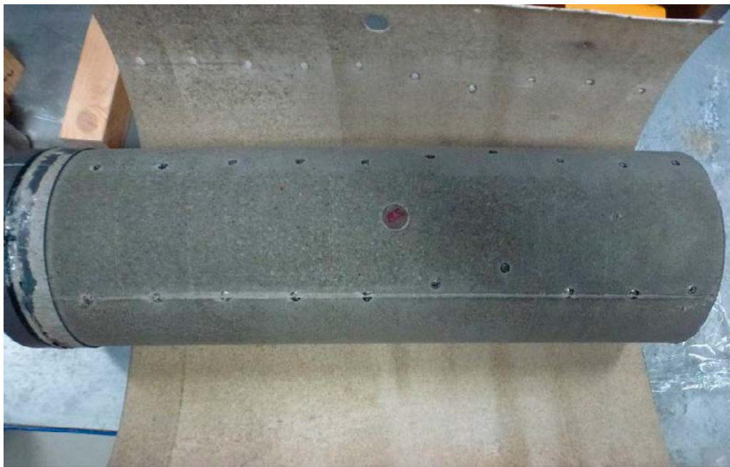
Figure 5-12. TZH. The plastic filter has been removed. Note the two rows of feet used to centralize the blocks. The circular point at the middle marked red is where the piston from the radial pressure measurement 1:B was located.
