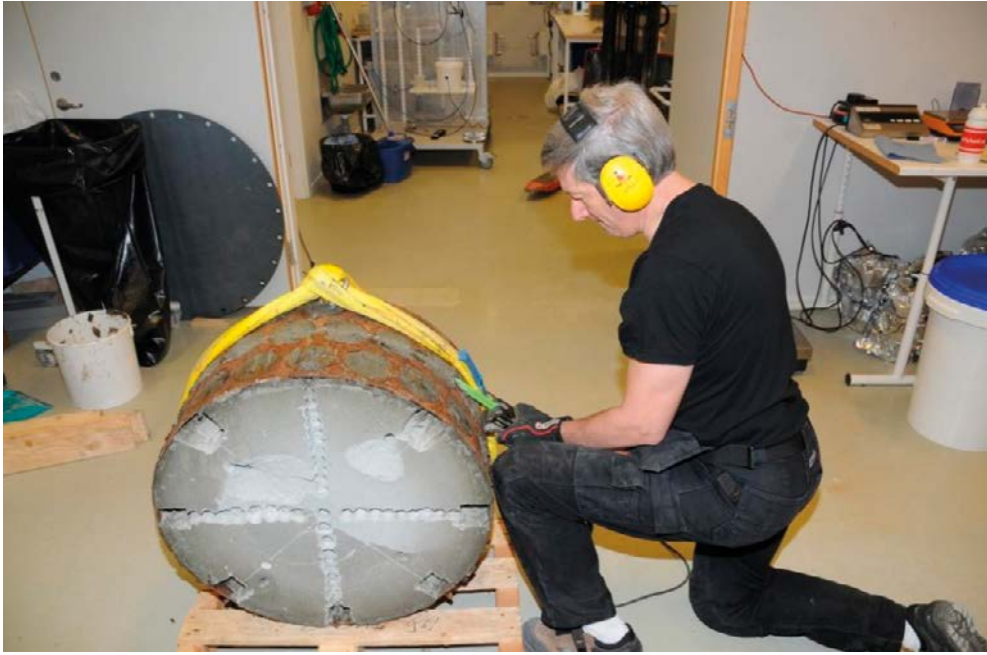
Figure 4-21. BB IV, cross section B. In order to uncover the bentonite in cross section B parts of the SC shell was cut off.
