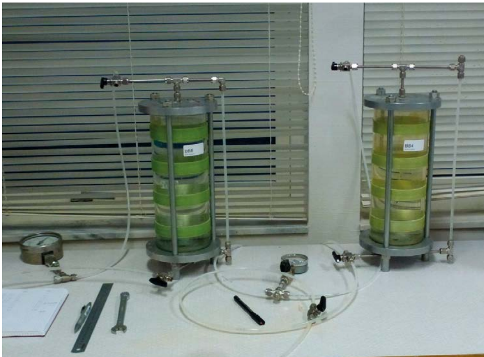
Figure 4-7. BB IV. Cells used to apply pressurized water to the filters in the test.
