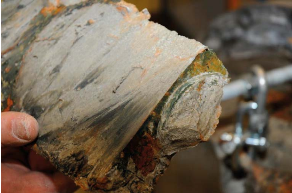
Figure 4-29. BB IV, cross section C. Photo showing a bentonite piece sampled from the SC-rock gap. The protrusion which can be seen on the surface facing right is material which has swelled into one of the feet.
