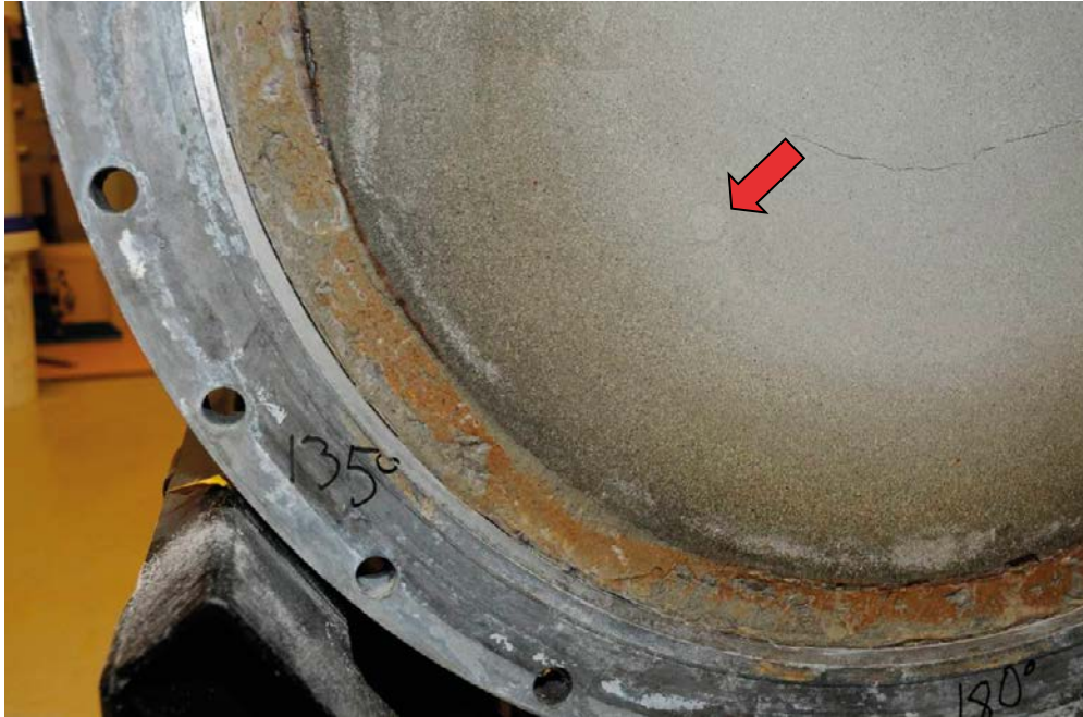
Figure 4-16. BB IV, cross section D. Close-up of cross-section D showing the position where the piston measuring the axial pressure (A1, 135 °) has been in contact with the bentonite.
