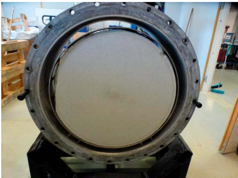
Figure 4-3. BB IV. The SC is installed and adjusted in the test cell. A part of the bentonite block has fallen off at the left side.
