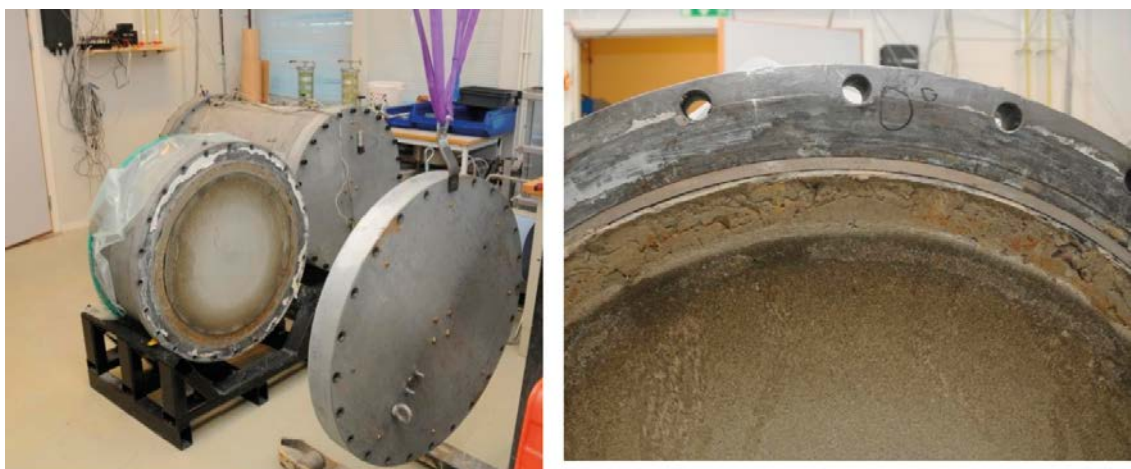
Figure 4-15. BB IV, cross section D. LEFT: The bentonite surface just inside the steel lid in section D is uncovered. RIGHT: Close up showing the bentonite filled SC-rock gap. The gap seems to have been filled up completely by the swelling bentonite.
