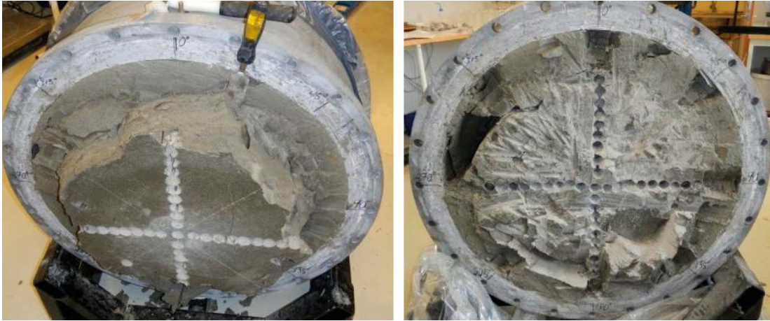
Figure 3-8. BB III, cross section B. LEFT: Uncovering of cross section B. RIGHT: Cross section B after complete sampling.
