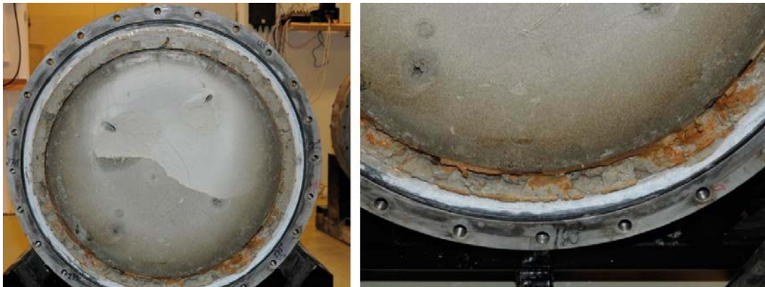
Figure 4-12. BB IV, cross section A. LEFT: The bentonite surface just inside the steel lid in cross section A. RIGHT: Close up showing the bentonite filled SC-rock gap. The space inside the feet has also been filled up with bentonite gel.
