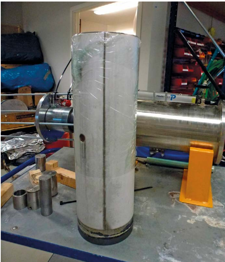
Figure 5-8. TZH. The distance block section (block side) has been removed. The bentonite is still covered with the plastic filter and a protective layer of thin plastic has been wrapped around to prevent drying.
