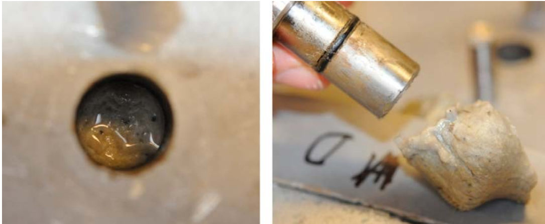
Figure 4-27. BB IV, cross section C. LEFT: Photo showing the uncovered bentonite surface inside the piston of radial pressure measurement C1 before sampling. RIGHT: the sample taken from just inside the piston of the radial pressure measurement C1.
