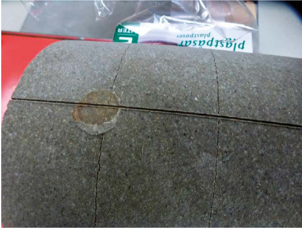
Figure 5-13. TZH. View of the top side and the position of pressure measurement 1:A. Note the cracks from the earlier block boundaries.
