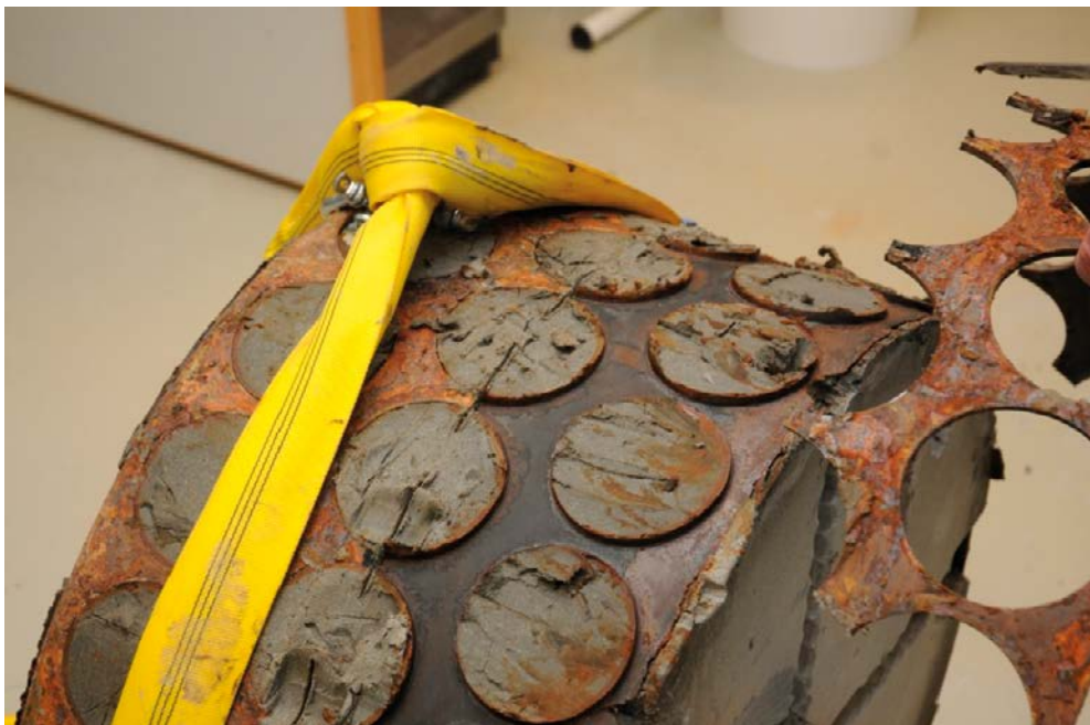
Figure 4-22. BB IV, cross section B. Photo showing the uncovered bentonite block surface after removal of a SC shell part
