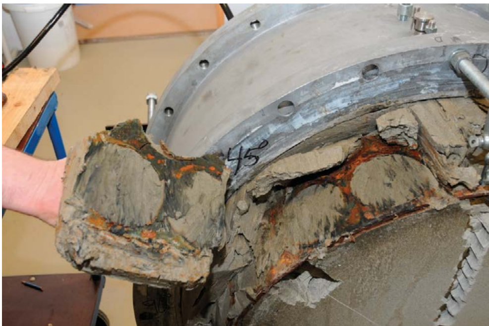
Figure 4-28. BB IV, cross section C. A bentonite piece has come loose from the SC surface. As shown in the photo there are no empty voids present in the SC-rock gap. The gap is completely filled with bentonite.
