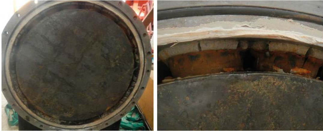
Figure 2-7. BB II, cross section A. LEFT: cross section directly after the lid was removed. RIGHT: close up of the “muffins”.
