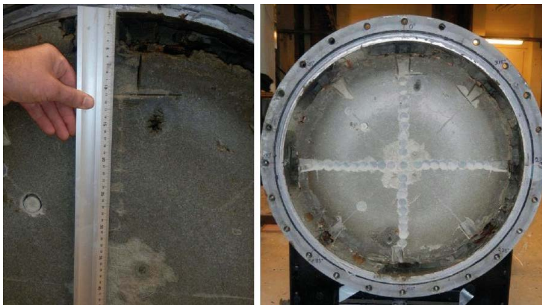
Figure 2-9. BB II, cross section F. LEFT: marking out the sample pattern inside the SC. RIGHT: overview of cross section F after the sampling.
