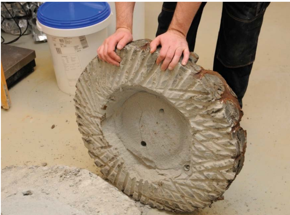
Figure 4-34. BB IV, cross section C. Photo showing the block part that was removed in order to uncover cross-section C.
