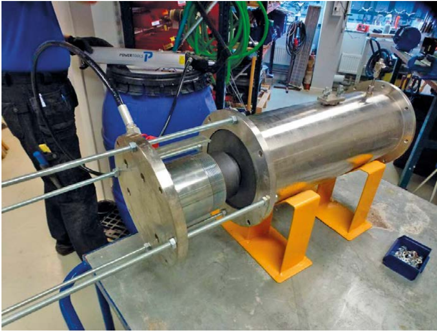
Figure 5-7. TZH. The bentonite in each of the test cell halves was pushed out using a hydraulic piston.
