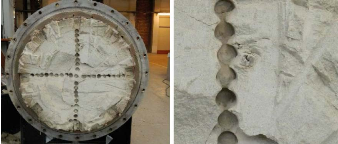
Figure 2-12. BB II, cross section D. LEFT: cross section D after complete sampling. RIGHT: one of the holes used for lifting the blocks was located nearby the sampling profile.
