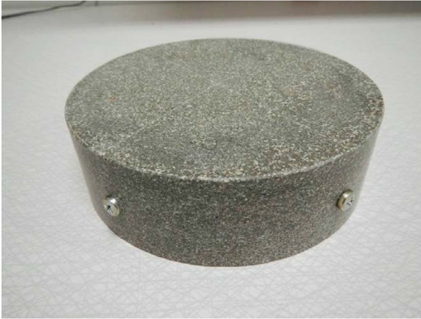
Figure 5-2. TZH. Photo of a bentonite block. The screws used to simulate the feet can be seen at the mid-height of the block periphery.
