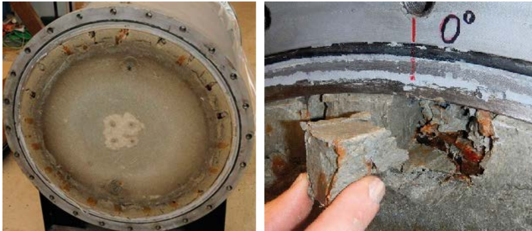
Figure 2-8. BB II, cross section F. LEFT: cross section directly after the lid was removed. RIGHT: sampling of the SC-rock gap.
