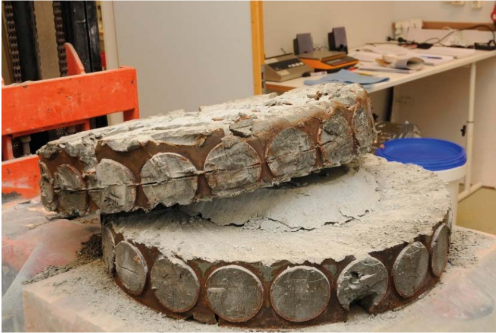
Figure 4-33. BB IV, cross section C. Uncovering cross-section C. Note that there is an obvious fracturing separating the outer parts and the central part.
