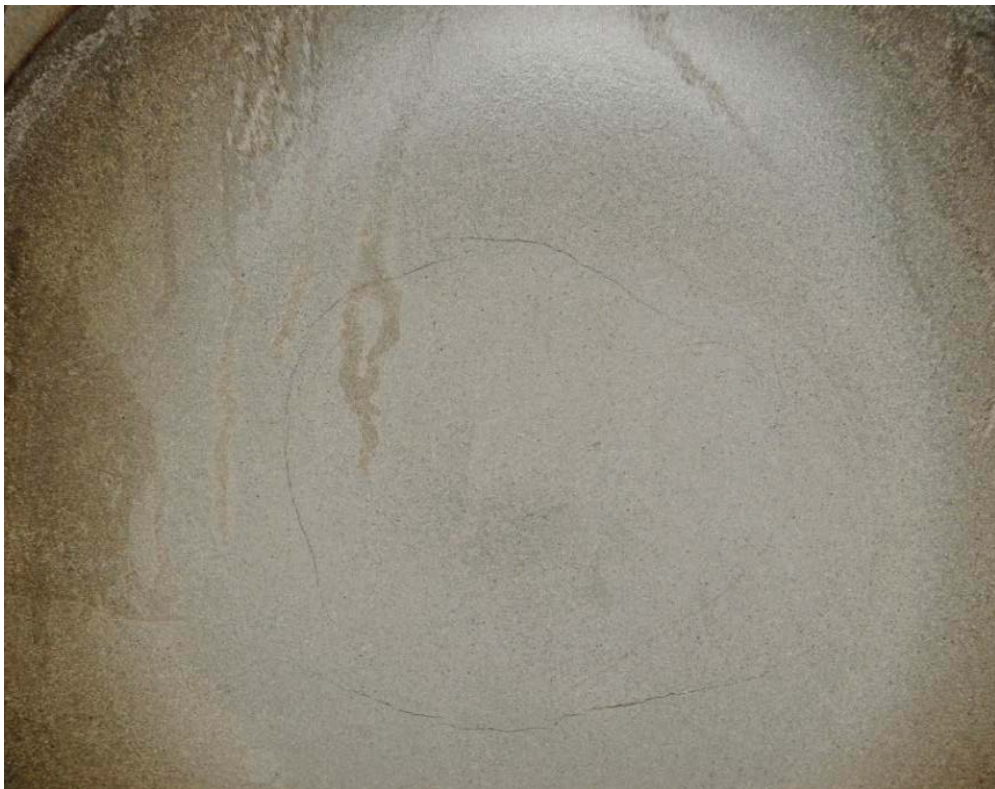
Figure 4-17. BB IV, cross section D. Close up showing the central parts of cross section D. There is a very clear fracture separating the innermost part from the rest of the block. The fracture was found to be present through the whole block.
