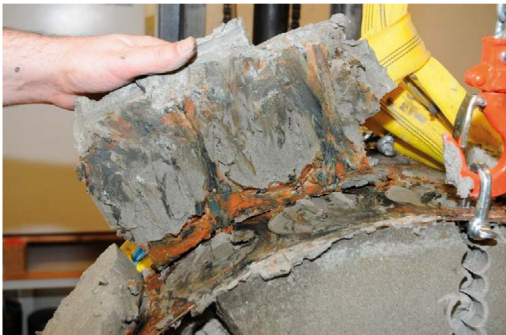
Figure 4-20. BB IV, cross section B. Close up showing a bentonite piece in section A–B. (Specimen S2, see Section 10.4.2).
