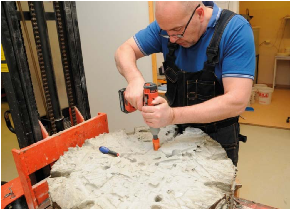
Figure 4-26. BB IV, cross section B. After having uncovered cross section B completely the sampling of the bentonite started. The sampling was made by use of a small core drill.
