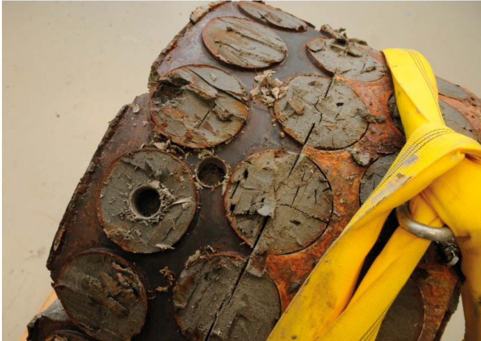
Figure 4-23. BB IV, cross section B. Close up showing some extra sampling performed. One sample was drilled out from the middle of a perforated hole and one from the area between three holes (Specimen S8, see Section 10.4.2)
