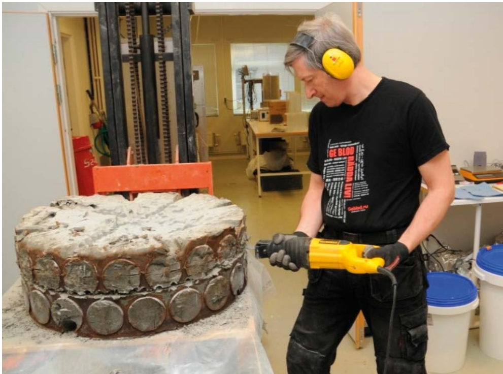
Figure 4-32. BB IV, cross section C. Sawing off the material left between the drilled boreholes.
