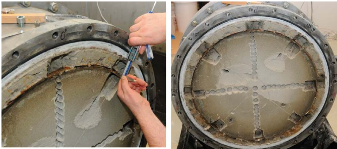
Figure 4-14. BB IV, cross section A. LEFT: Measuring the distance between SC and the inner test cell wall. RIGHT: Overview of cross-section A after having finished the sampling.
