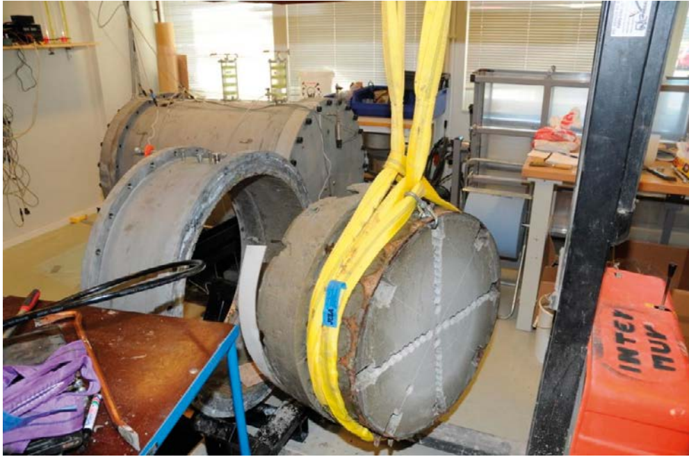
Figure 4-19. BB IV, cross section B. After having finished the sampling of the SC-rock gap in cross section C, the rest of the SC including the swollen bentonite was lifted out from the test cell.
