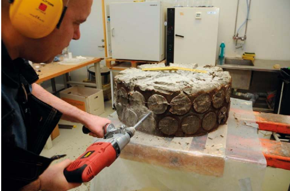
Figure 4-31. BB IV, cross section C. Seam drilling to uncover cross section C.
