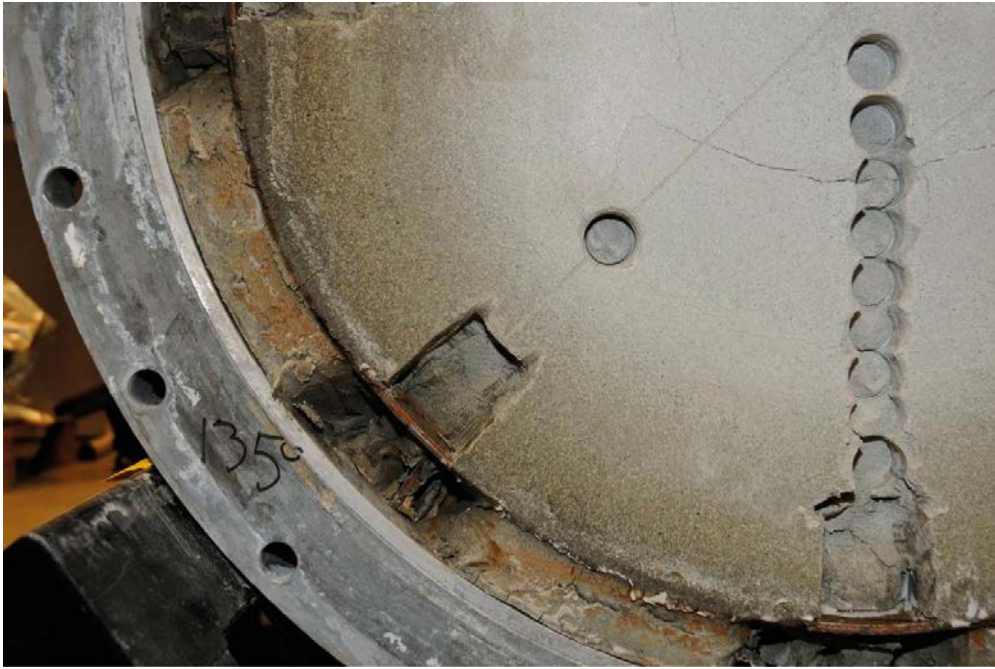
Figure 4-18. BB IV, cross section D. Close-up of cross section D, directions 135° to 180° after having finished the sampling.
