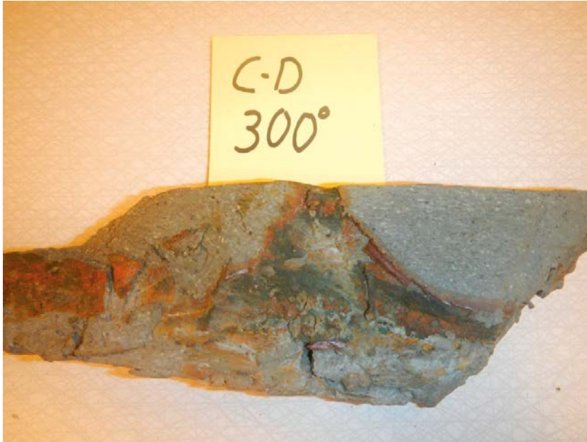
Figure D-26. BB IV. Photo showing specimen S7. The central, discolored area, has been beneath the SC shell.
