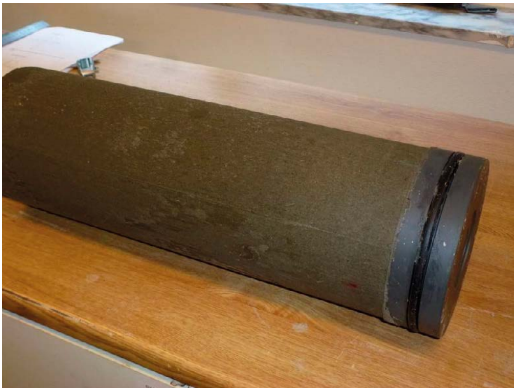
Figure 5-14. TZH. The transition zone section containing both pellets and blocks is ready for sampling (former pellet section is to the right and outside is the PVC piston with a central O-ring mounted). No evident block boundaries could be seen before the sampling started on this half, but some appeared at the left part i.e. at the block side, after start cutting.
