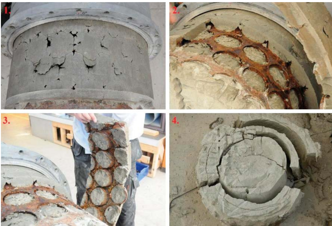
Figure 2-13. BB II, cross section C. (1) Muffin-shaped protrusions with empty volumes between some of the muffins. (2) Cut through the material within the SC-rock gap. (3) The bentonite within the SC-rock gap still held together when removed from the SC surface. (4) During the dismantling/sampling a protruding block part fell off in one piece.
