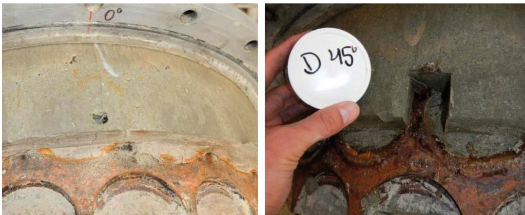
Figure 2-11. BB II, cross section D. LEFT: the hole from the sampling in the radial total pressure measurement position. RIGHT: the relative position between the sample taken at 45° and the perforation pattern is clearly seen.
