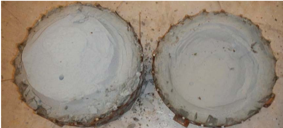
Figure 2-15. BB II, cross section B. The block fell apart and the inner samples had to be taken from the left piece while the outermost samples had to be taken from the right piece.
