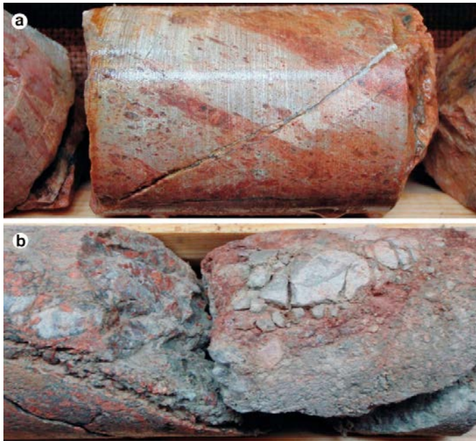
Figure 3-9. Photographs of selected drill core sections from the zone core of DZ2 in KAS12 showing (a) the intense brittle-ductile deformation and (b) strong argillic alteration.
