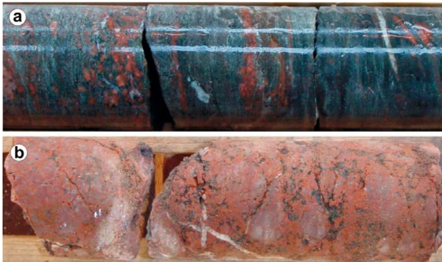
Figure 3-5. Photographs of selected drill core sections of DZ2 in KAS09. (a) Mylonitized section at 137.85–138.02 m. (b) Weakly argillized section with partly open fractures at 77.03 – 77.20 m.
