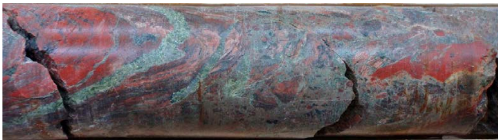
Figure 3-10. Photograph of a brecciated drill core section from the deformation zone core at 300.6–305.5 m of DZ3 in KAS12.
