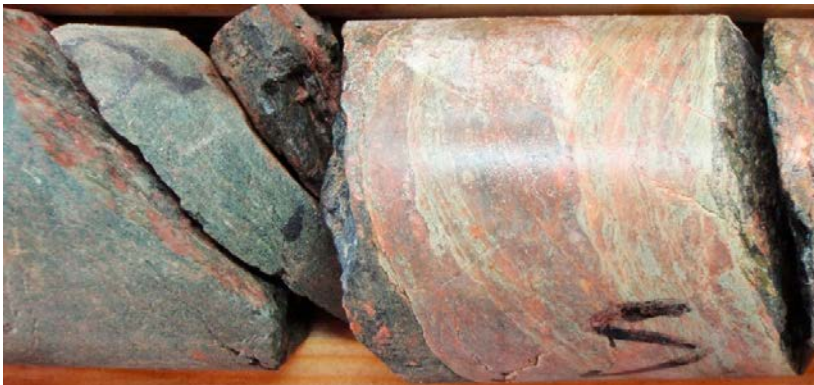
Figure 3-12. Photograph of the intense brittle-ductile deformation at approximately 59.2 m length in KAS13.
