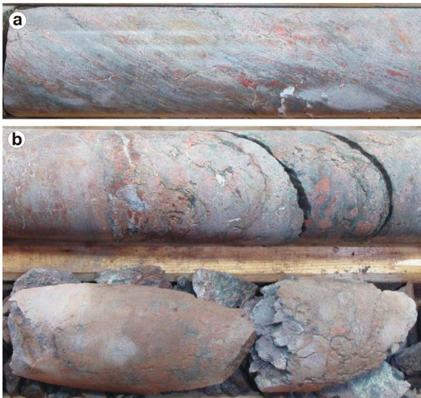
Figure 3-3. Photographs of selected drill core sections from the deformation zone core of DZ2 in KAS05. (a) Intense brittle-ductile deformation at 327.75–327.92 m. (b) Sections affected by argillization of weak (327.11–327.28 m) and strong (328.00–328.17 m) intensity.
