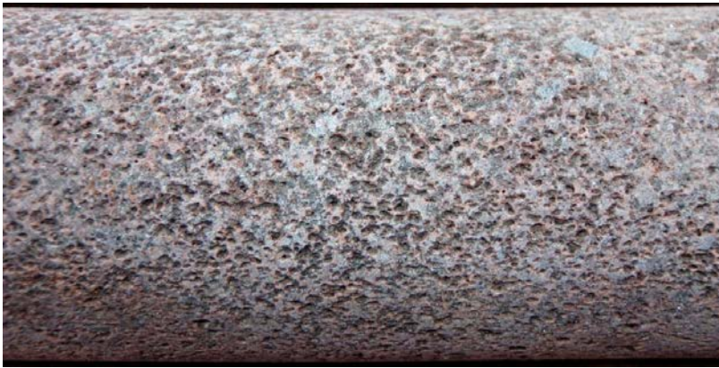
Figure 3-15. Photograph of a 1 dm core section of porous granite or episyenite from the interval 448.1–454.0 m in KAS16.
