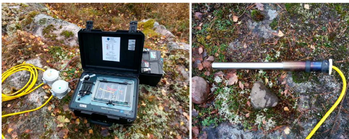
Figure 2-1. Photos of the data logger, external connection boxes and cables (left) and the sensor assembly with the added 2 kg lead weight (right).
