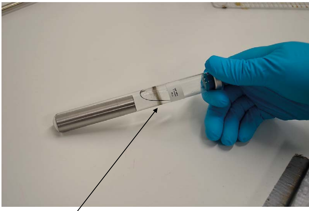
Figure 3-5. Black coloured precipitate on the tube glass in a tube containing a steel rod immersed in natural groundwater.
