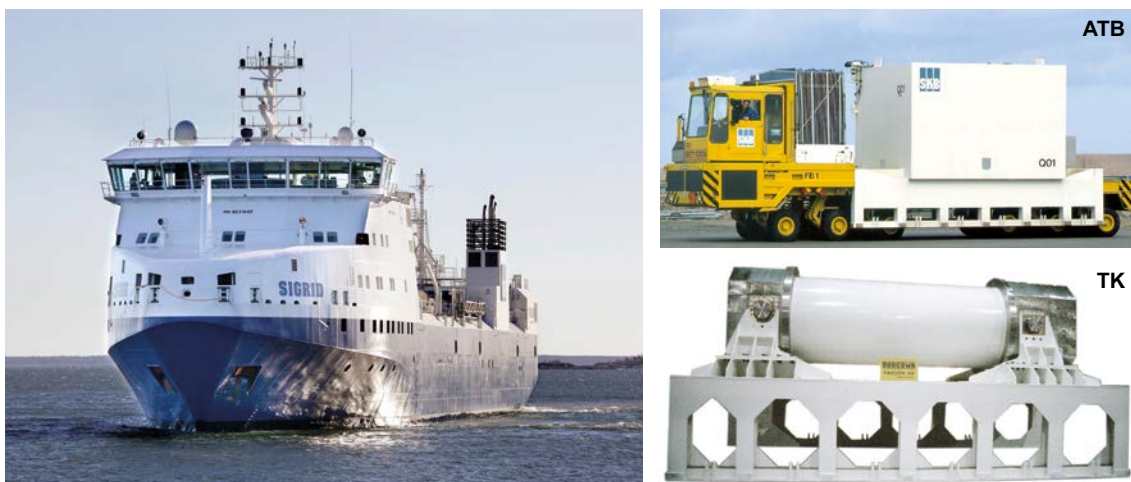
Figure 2-9. M/s Sigrid and transport container for short-lived radioactive waste (ATB) and transport cask for core components (TK).
