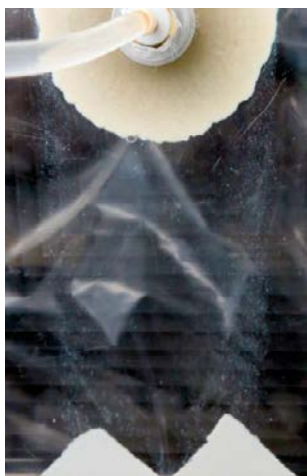
Figure 3-6. Artificial fracture test with calcium montmorillonite sample using deionized water flowing at \sim 0.09 ml/min; fracture aperture was 1 mm and fracture slope angle was 90^\circ . Image taken 644 h after start of test. Part of Figure 3-10 in Schatz and Akhanoba (2016).
