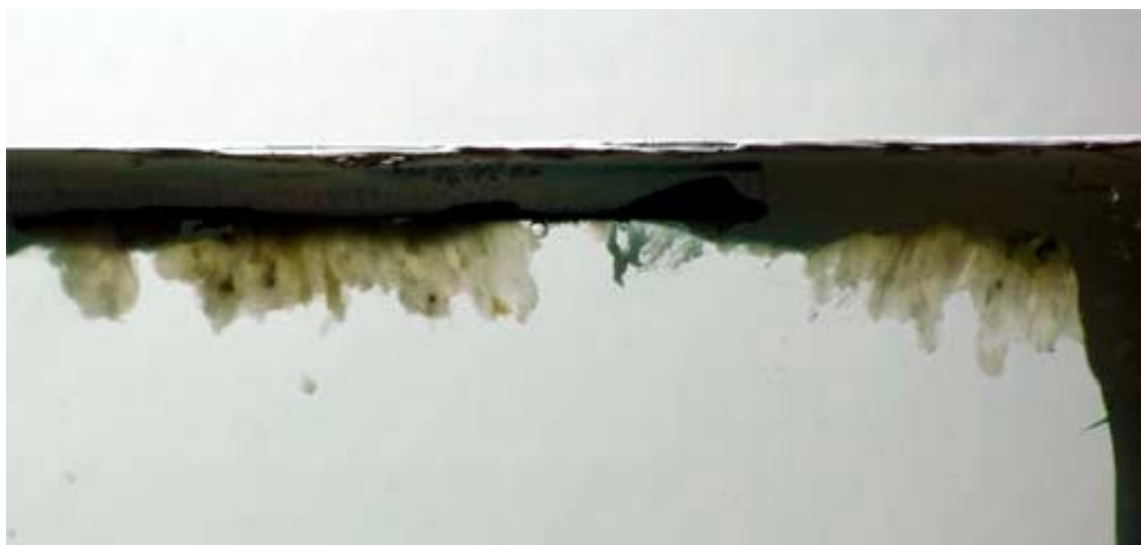
Figure A3-2. Enlargement of the upside down turned slit 24 hours later. Gel is slowly pulled downward by gravity. Small gel blobs are released and very slowly move downward. The whole picture is about 4 cm high.
