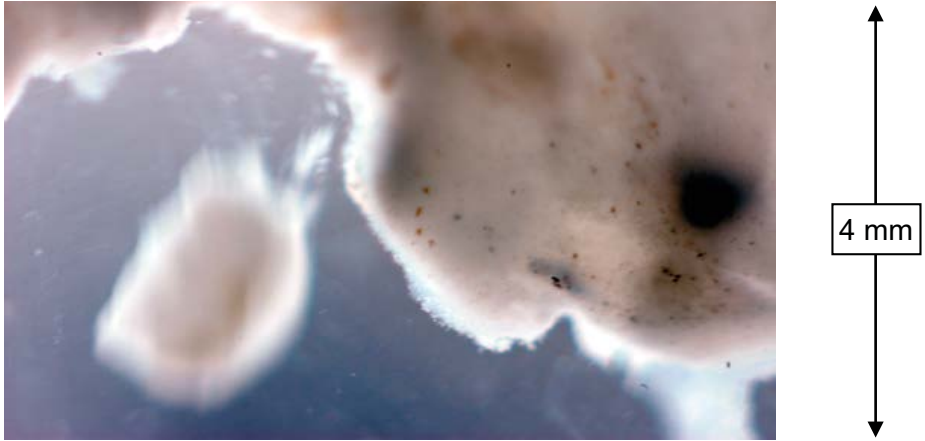
Figure A3-3. An enlarged detail of the hanging gel. The whole picture is 4 mm high. Large and small black particles are clearly seen.
