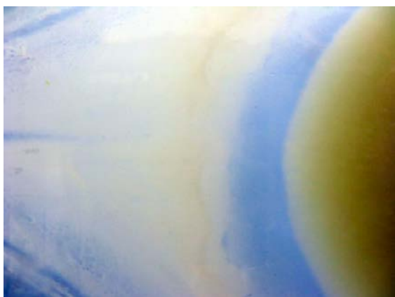
Figure A3-9. Close-up picture of down-stream region from a 50/50 mix of Ca and Na smectite in de-ionised water. Flow is from right to left. Figure 45 in Schatz et al. (2013).
