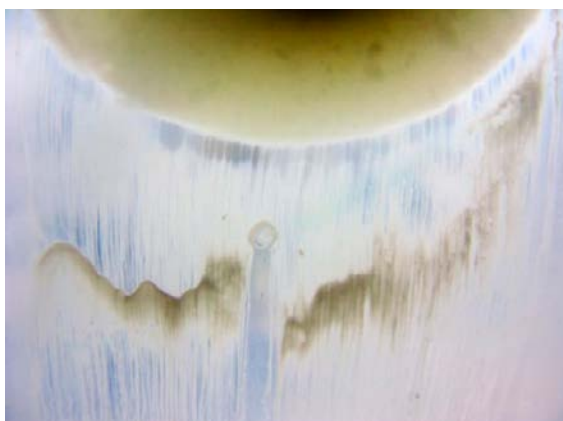
Figure A3-8. Close-up picture of sedimenting agglomerates in de-ionised water. The cylindrical region is 2 cm in diameter. Figure 59 in Schatz et al. (2013).
