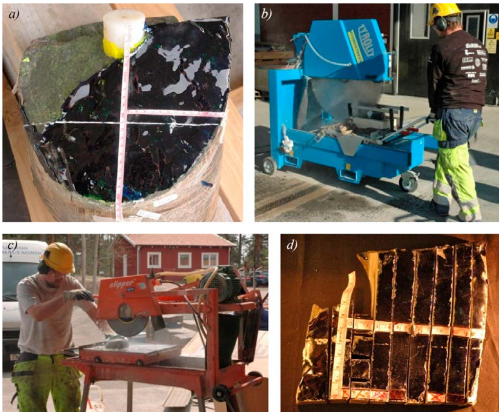
Figure 5-1. a) KXTT3, core piece 15 with reinforced surface and measurement tapes added as reference lines before cutting. b) First cut of core pieces moulded in boxes using a larger cutter. c) Second cut into slices and rods using a smaller cutter. d) Slices and rods of core piece 15 from KXTT3.
