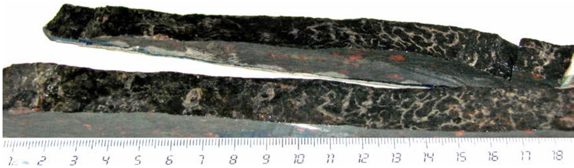
Figure 5-18. Photograph of the fracture surface of sample 8-III-7 (no coverage of reinforced epoxy on the left side).
