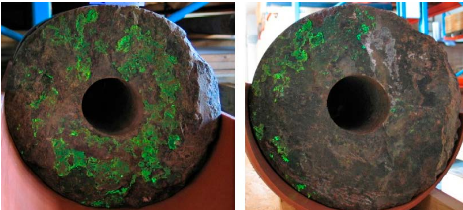
Figure 4-5. KXTT3, fracture at c. 13.1 m, core piece 2 (to the left) and 3 (to the right) in UV-lighting.
