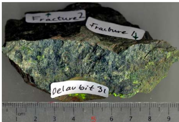
Figure 5-14. Fracture surface of Fracture 1 from piece 31 from KXTT3, coated by chlorite and clay minerals, and in parts, epoxy (e.g. to the far right). From Hakami et al. (2014).
