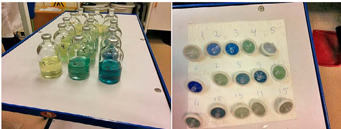
Figure 3-1. MB-II. No control of oxygen and filtration after addition of reagents show montmorillonite traces. Ibeco BF bentonite used.
