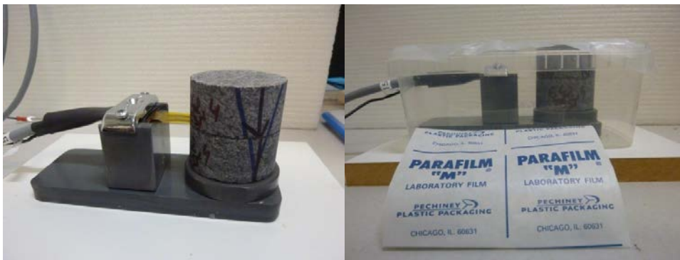
Figure 3 Specimens and TPS sensor (left) and moisture tight container (right).
