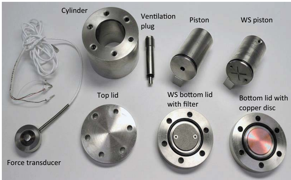
Figure 2-1. View of all parts included in a test cell. All parts in contact with the bentonites were made of titanium. See text for details. WS = water saturation.
