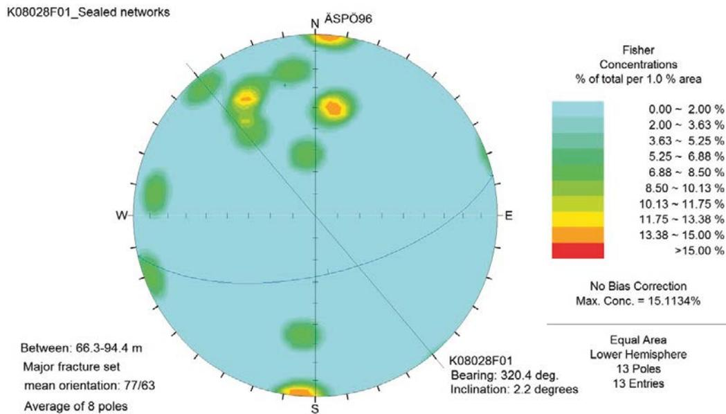
**Figure 5-4.** Stereogram (strike/dip poles) showing data from fracture measurements in Boremap, in terms of upper contacts of sealed networks between 66.3–94.4 m in borehole K08028F01. The coordinate system is Åspö96. Bearing of borehole K08028F01 marked as a line. The diagrams have not been adjusted for borehole orientation bias.
