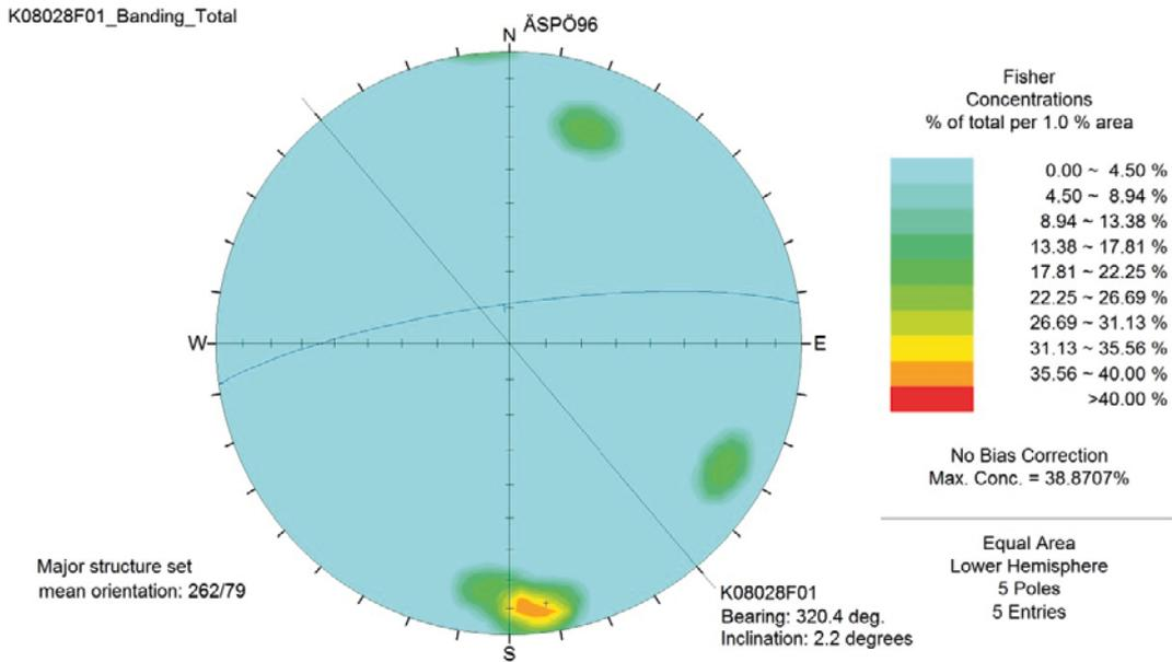
**Figure A1-7.** Data from structural measurements in Boremap of banding in borehole K08028F01. The coordinate system is Äspö96. Bearing of borehole K08028F01 marked as a line. Stereogram (strike/dip poles). The diagrams have not been adjusted for borehole orientation bias.
