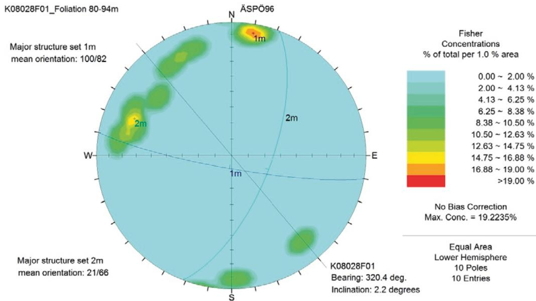
**Figure A1-10.** Data from structural measurements in Boremap of foliations in borehole K08028F01 between 80–94 m. The coordinate system is Äspö96. Bearing of borehole K08028F01 marked as a line. Stereogram (strike/dip poles). The diagrams have not been adjusted for borehole orientation bias.
