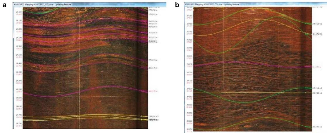
**Figure 5-9.** OPTV-images of good quality from borehole K08028F01, screen dump from the Boremap software. a) 12.452–13.103 m adjusted length (red numbers), showing both faint foliation at approximately 12.5 m and medium intensity banding at approximately 12.6 m. b) 27.627–28.376 m adjusted length (red numbers), showing medium intensity banding at approximately 28 m.
