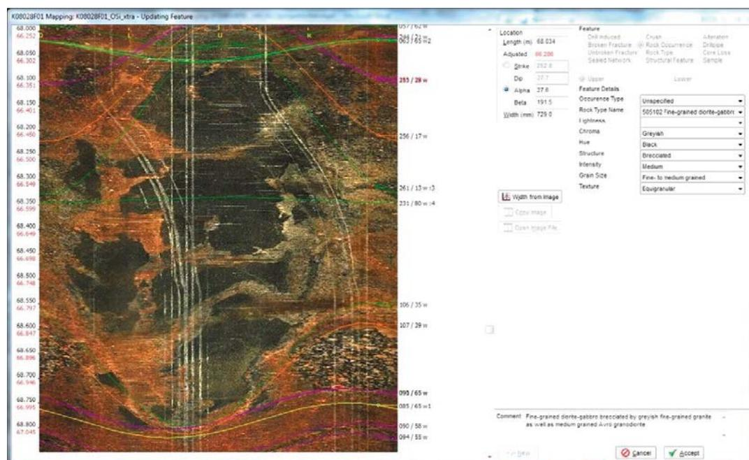
**Figure 5-8.** An OPTV-image of good quality from borehole K08028F01, screen dump from the Boremap software. An unspecified fine-grained diorite-gabbro brecciated by a greyish fine-grained granite and some medium grained Ävrö granodiorite occur between 66.252–67.045 m adjusted length (red numbers),
