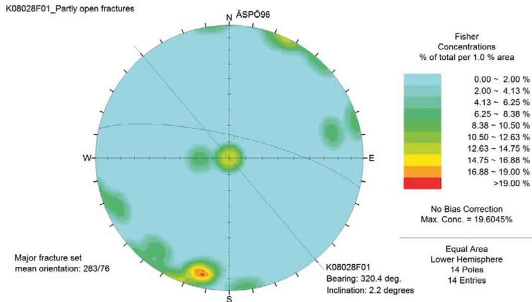
**Figure A1-4.** Data from Boremap mapping of all partly open fractures in borehole K08028F01. The coordinate system is Äspö96. Bearing of borehole K08028F01 marked as a line. Stereogram (strike/dip poles). Two fractures do not cut the core and therefore have the designated strike/dip 0/0. The diagrams have not been adjusted for borehole orientation bias.
