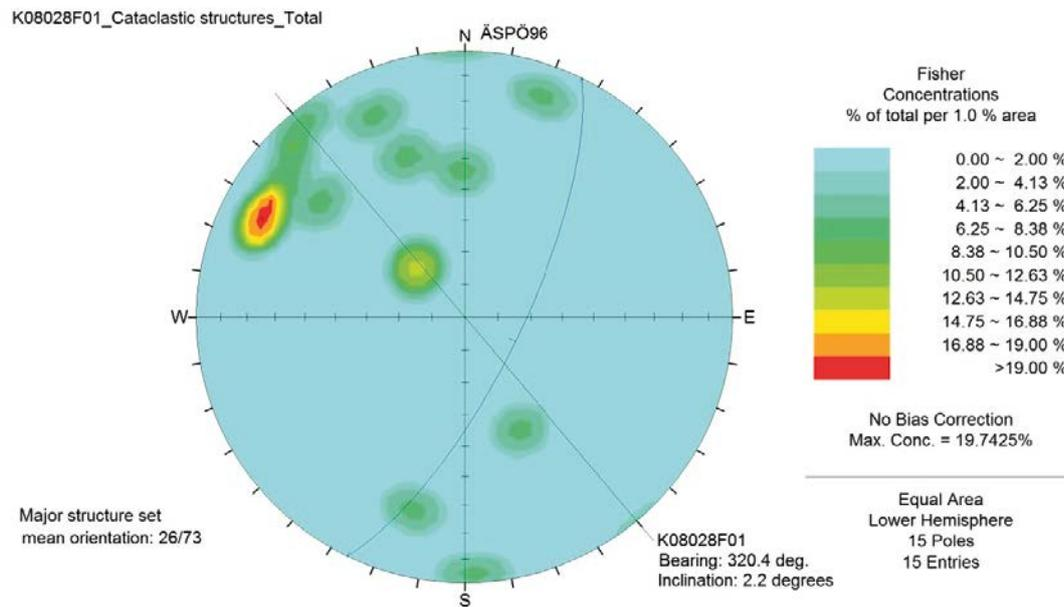
**Figure A1-6.** Data from structural measurements in Boremap showing cataclastic structures in borehole K08028F01. The coordinate system is Äspö96. Bearing of borehole K08028F01 marked as a line. Stereogram (strike/dip poles). The diagrams have not been adjusted for borehole orientation bias.
