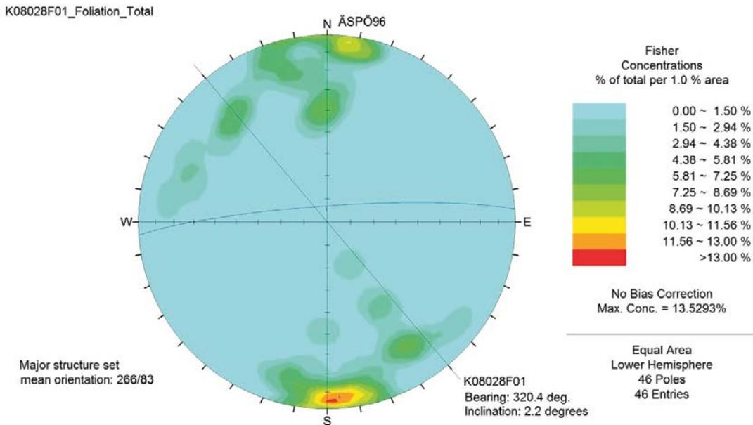
**Figure A1-8.** Data from structural measurements in Boremap of foliations in borehole K08028F01. The coordinate system is Äspö96. Bearing of borehole K08028F01 marked as a line. Stereogram (strike/dip poles). The diagrams have not been adjusted for borehole orientation bias.
