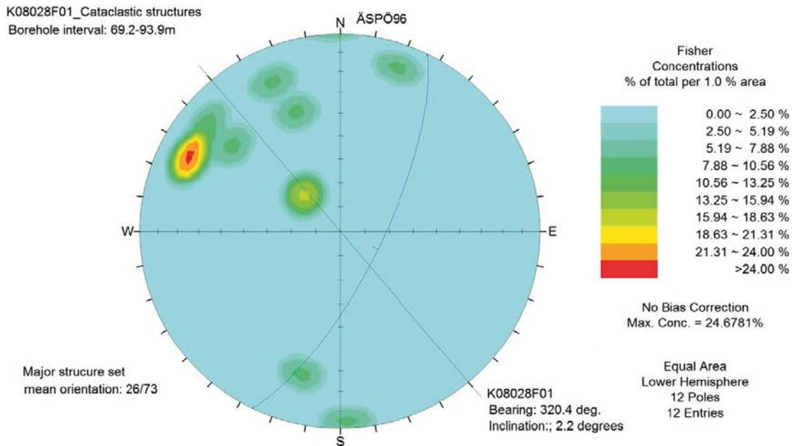
**Figure 5-6.** Stereogram (strike/dip poles) showing data from structural measurements in Boremap. Upper contacts of cataclastic structures between 69.2–93.9 m in borehole K08028F01. The coordinate system is Äspö96. The bearing of borehole K08028F01 is marked as a line. The diagram is not adjusted for borehole orientation bias.
