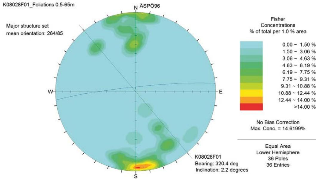
**Figure A1-9.** Data from structural measurements in Boremap of foliations in borehole K08028F01 between 0.5–65 m. The coordinate system is Äspö96. Bearing of borehole K08028F01 marked as a line. Stereogram (strike/dip poles). The diagrams have not been adjusted for borehole orientation bias.
