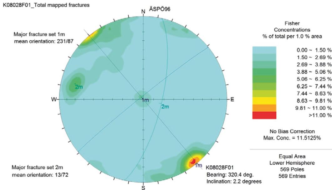
**Figure A1-1.** Data from Boremap mapping of all logged fractures in borehole K08028F01. The coordinate system is Åspö96. Bearing of borehole K08028F01 marked as a line. Stereogram (strike/dip poles). Fourteen fractures do not cut the core and therefore have the designated strike/dip 0/0. The diagrams have not been adjusted for borehole orientation bias.
