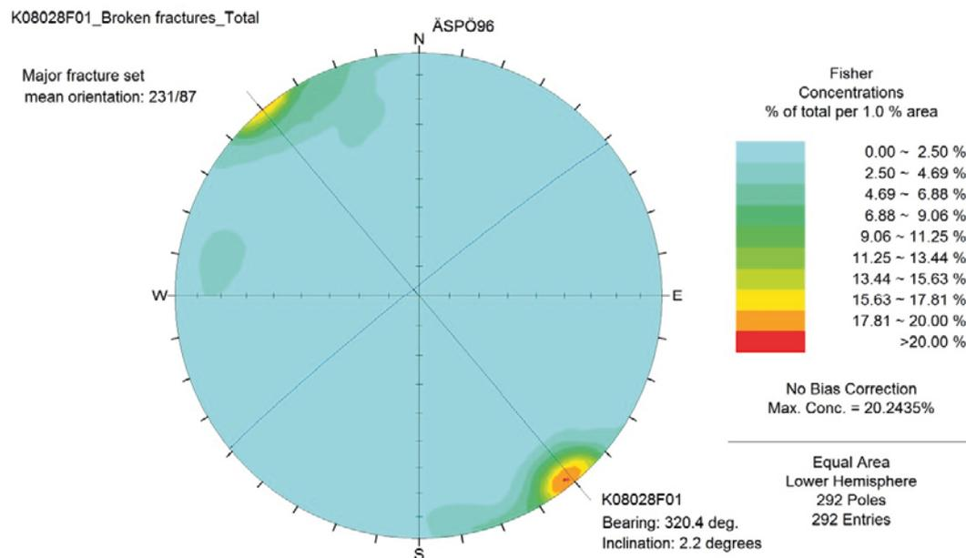
**Figure A1-2.** Data from Boremap mapping of all broken fractures in borehole K08028F01. The coordinate system is Åspö96. Bearing of borehole K08028F01 marked as a line. Stereogram (strike/dip poles). One fracture does not cut the core and therefore has the designated strike/dip 0/0. The diagrams have not been adjusted for borehole orientation bias.
