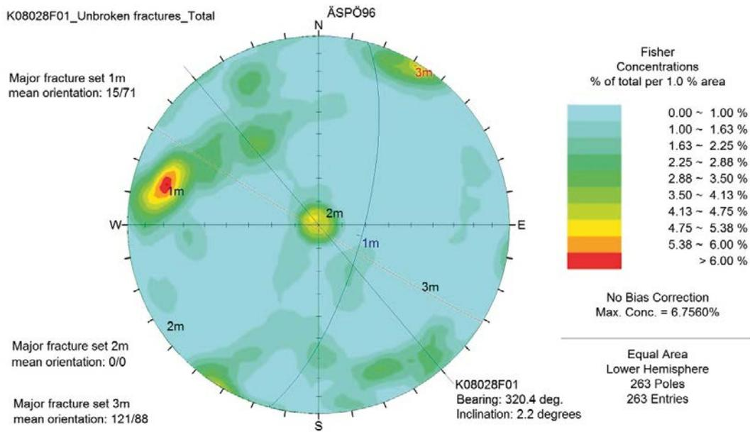
**Figure A1-3.** Data from Boremap mapping of all unbroken fractures in borehole K08028F01. The coordinate system is Äspö96. Bearing of borehole K08028F01 marked as a line. Stereogram (strike/dip poles). Eleven fractures do not cut the core and therefore have the designated strike/dip 0/0. The diagrams have not been adjusted for borehole orientation bias.
