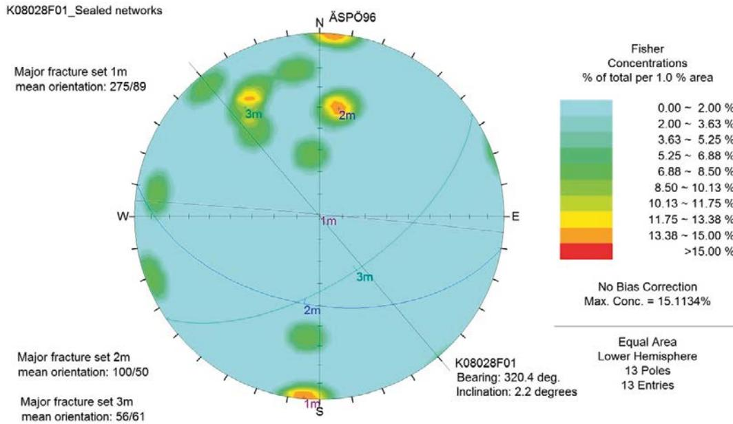
**Figure A1-5.** Data from measurements in Boremap showing upper contacts of sealed networks in borehole K08028F01. The coordinate system is Äspö96. Bearing of borehole K08028F01 marked as a line. Stereogram (strike/dip poles). The diagrams have not been adjusted for borehole orientation bias.
