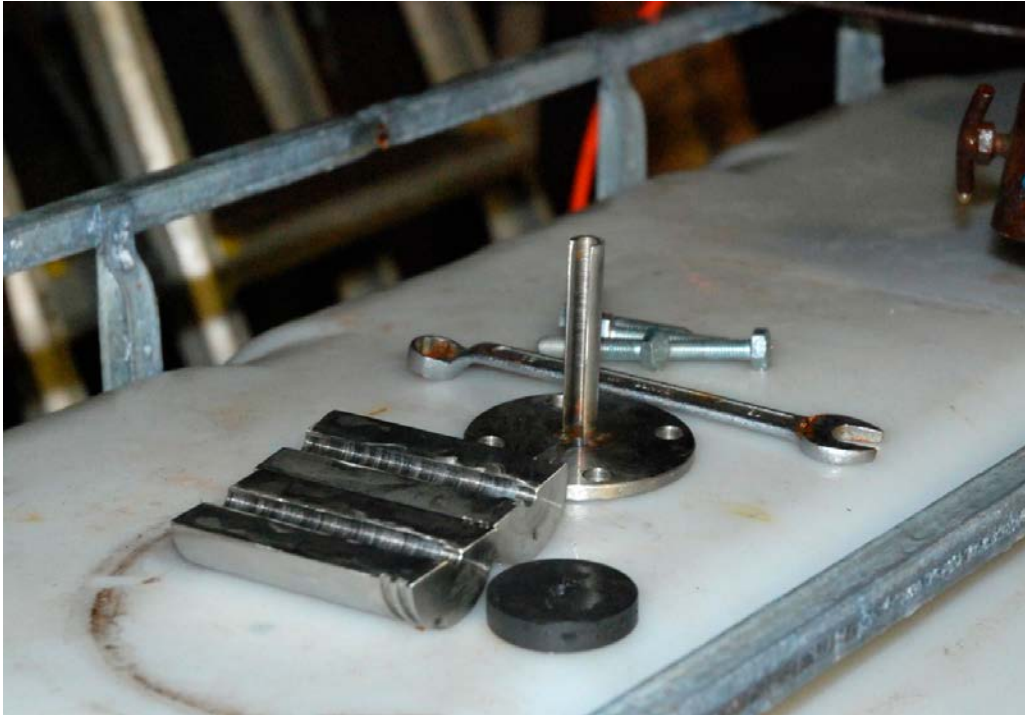
Figure 3-2. The outermost part of the sealing device opened up on the work bench.
