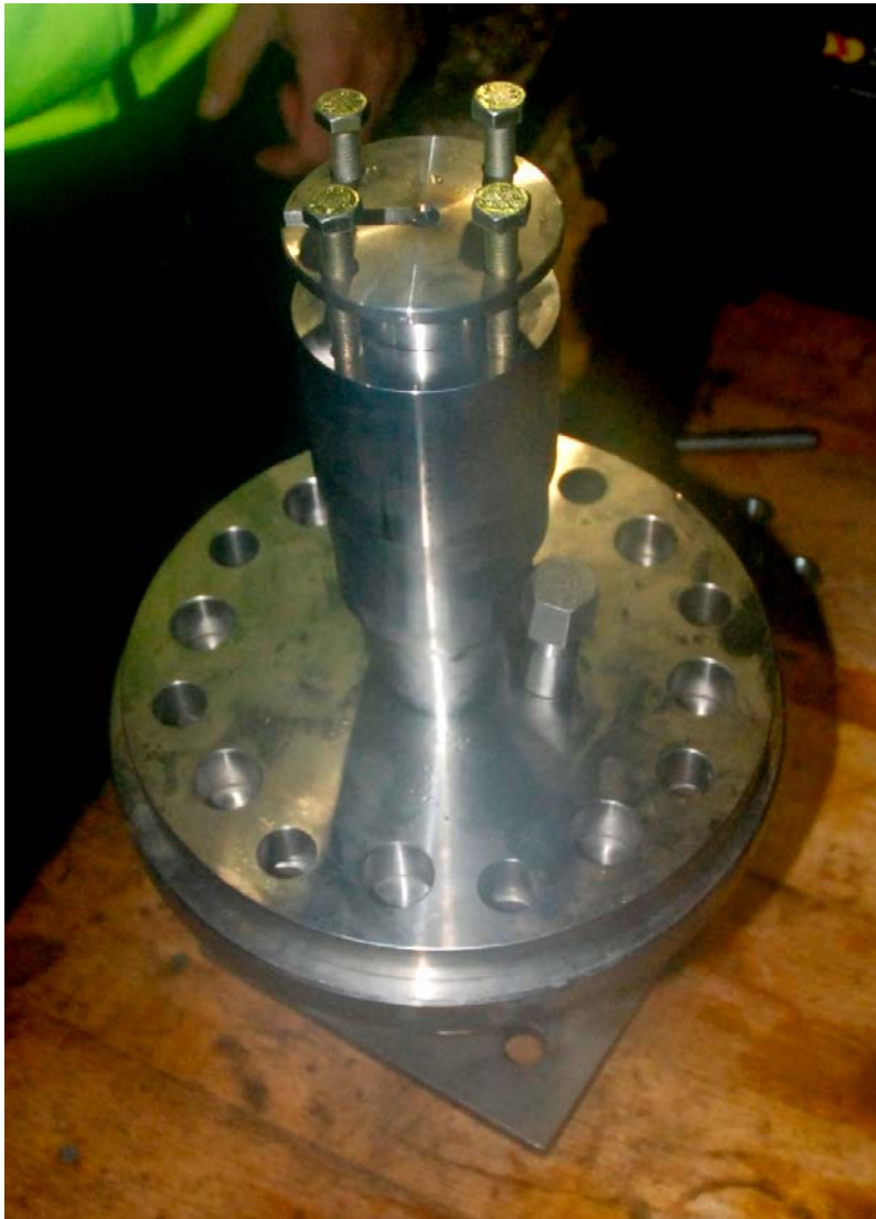
Figure 3-1. The sealing device. The wide part is fastened onto the borehole bushing. The outermost part is fastened after removing the push rods and the air hose. The logging cable runs through the whole device.
