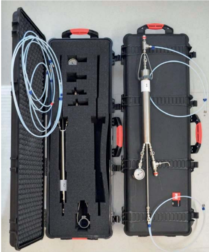
Figure 2-2. Left: Flow-through sampler for dissolved gas dismantled for transport. Right: A mounted sampler with the piston in a position corresponding to a full sample (400 mL) with pressure reducers, manometer, valves and connectors.
