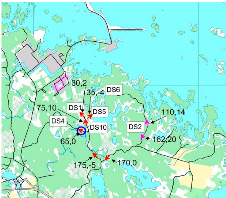
Figure 6-7. Measured DC currents in wires of the grounding grid that connects the drill sites (redrawn from Nissen et al. 2005). Numbers are given in mA with values before commas representing a situation with Fenno-Skan transferring 480 MW and the values after the commas representing Fenno-Skan out of operation. Magenta arrows indicate inferred current directions.
