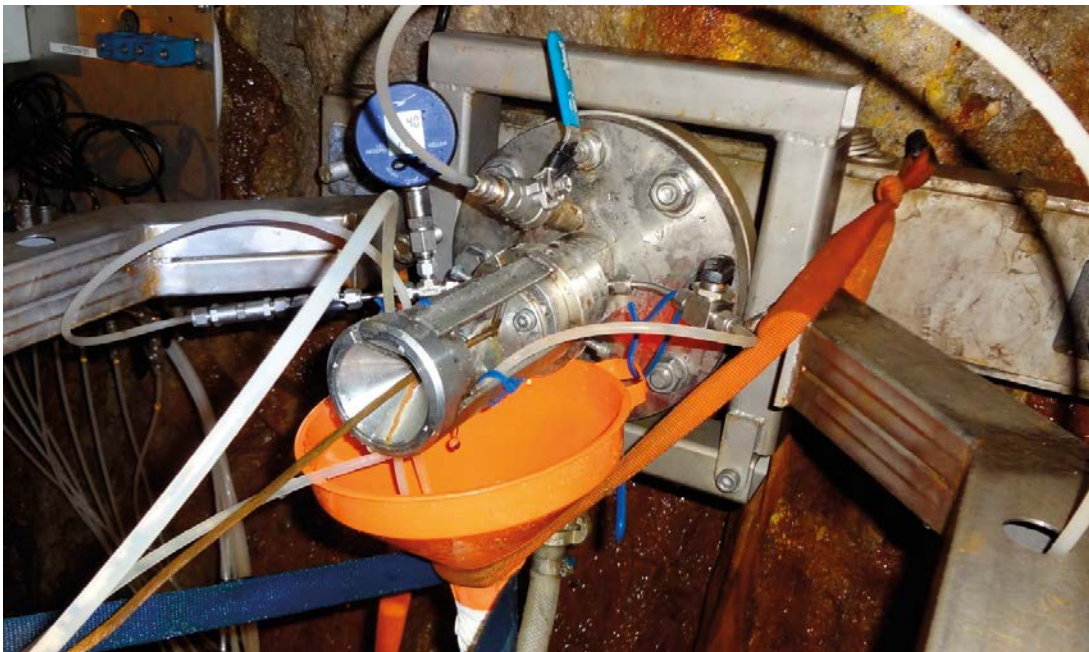
Figure 5-7. Sealing mechanism during the measurement.
