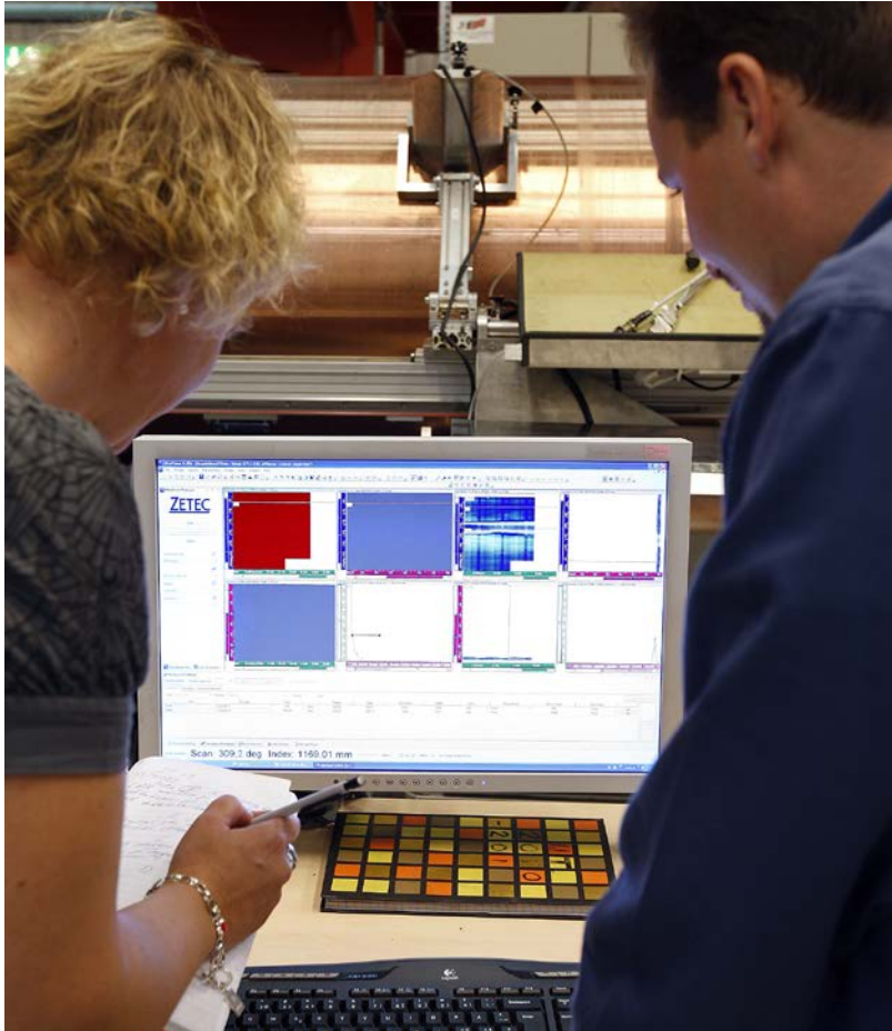
Figure 8-4. Ultrasonic technique is one of several techniques for non-destructive testing.
