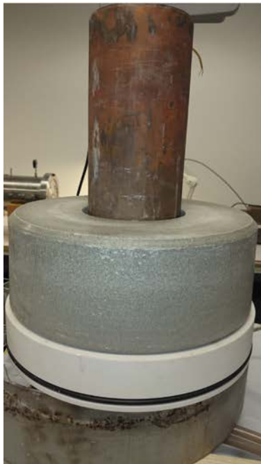
Figure 10-8. Upper left: Schematic illustration of the experimental set-up. Upper right: The heater (copper tube) and the bottom plate. Bottom left: One bentonite ring installed. Bottom right: Three bentonite rings and the massive upper block installed. The entire set-up is mounted on a scale (Birgersson and Goudarzi 2016).
