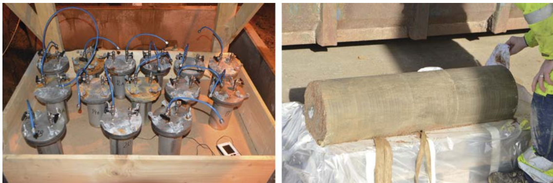
Figure 9-1. Steel containers containing material samples, groundwater from the Äspö HRL and crushed cement (left-hand picture) and a concrete cylinder with material samples (right-hand picture).
