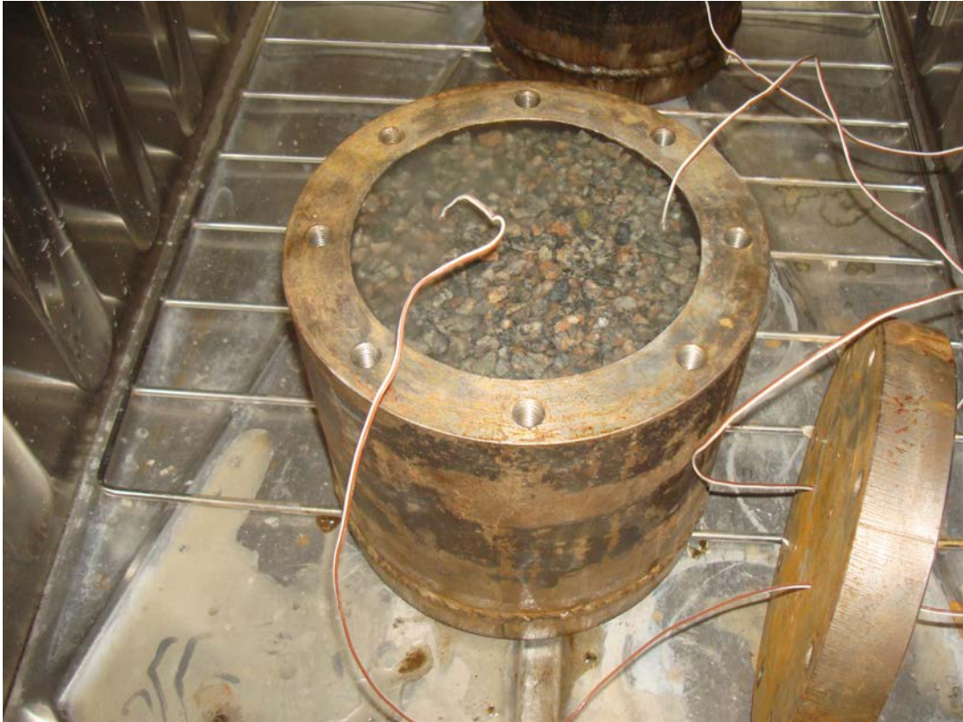
Figure 9-4. Experimental set-up used by Pålbrink and Rydman (2013). The strong steel container contains a water-saturated gravel bed in which a concrete cylinder has been installed. The steel cylinder corresponds here to the bedrock while the gravel bed and concrete cylinder correspond to the backfill and concrete structure in 1BMA. Note the cylinder lid with inlets for cords from temperature gauges attached to the sample.
