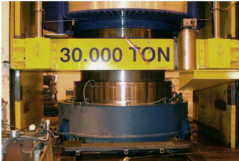
Figure 10-16. Uniaxial press for fabrication of buffer blocks.
