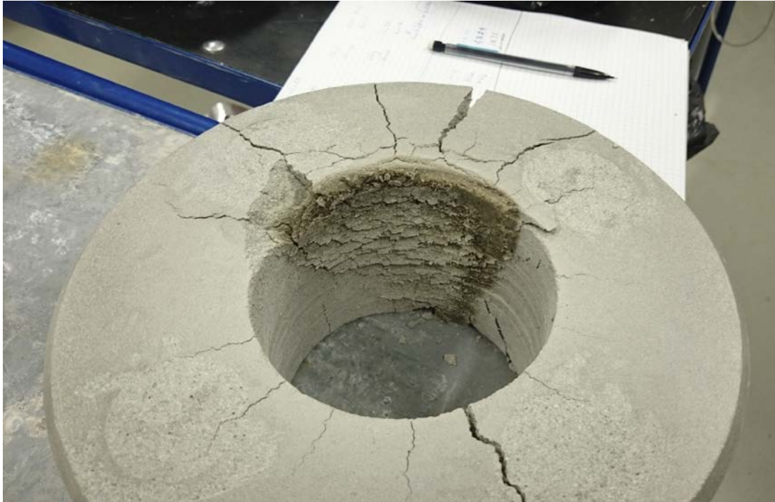
Figure 10-9. Example of a block with a forming condensation zone and the fractures caused by it.
