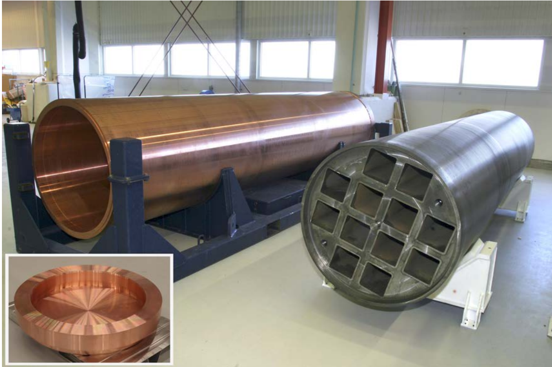
Figure 2-7. Copper shell and nodular iron insert (the inset photo shows the copper lid).
