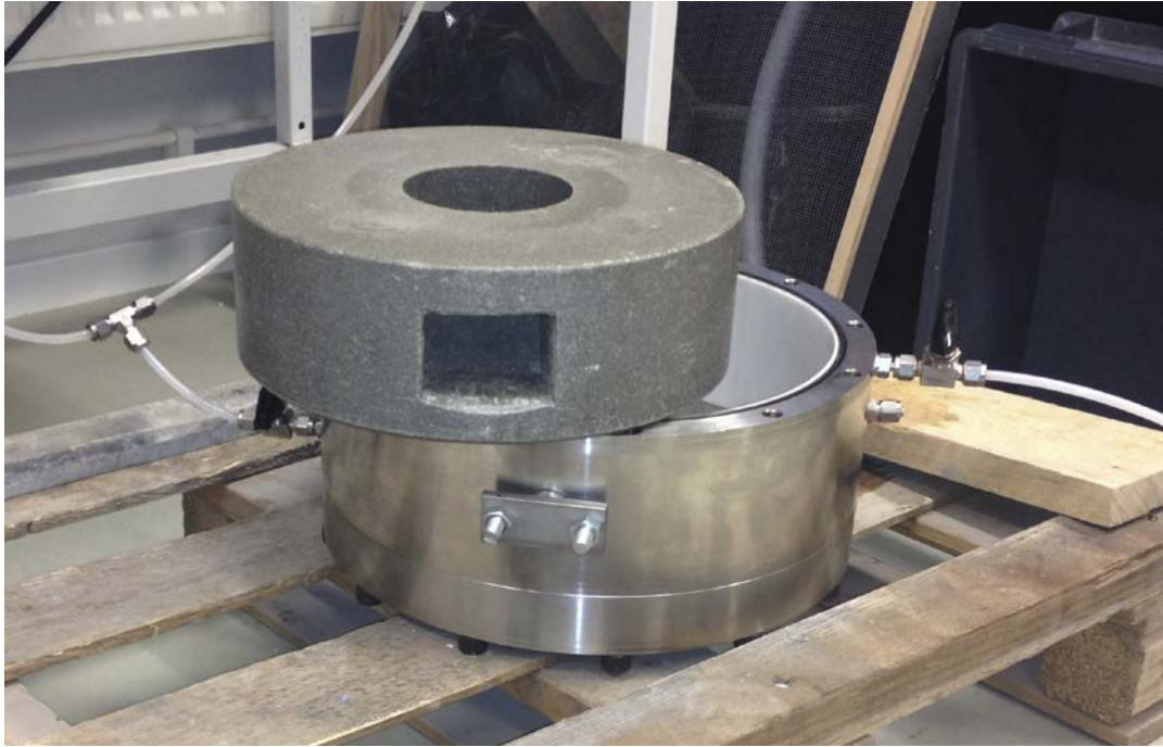
Figure 10-6. Sawn-out hole in the side of a bentonite block. This experiment is used as a modelling task in Task Force EBS.
