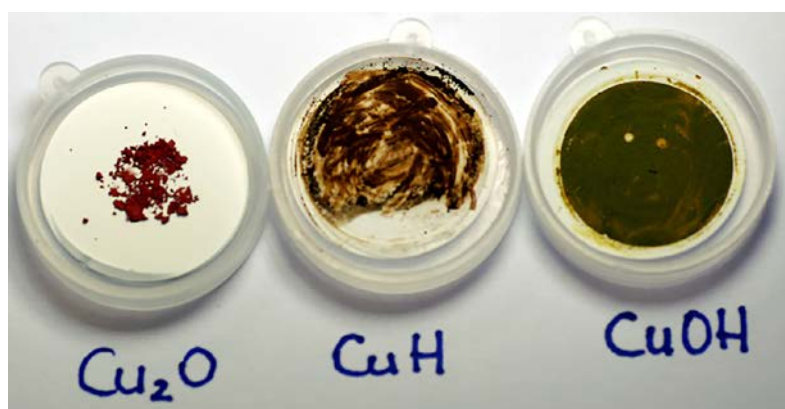
Figure 2-7. Powders of \text{Cu(I)} compounds with oxygen and hydrogen. \text{Cu}_2\text{O} is industrially produced, \text{CuH} and \text{CuOH} are synthesized in the nuclear chemistry lab at KTH.
