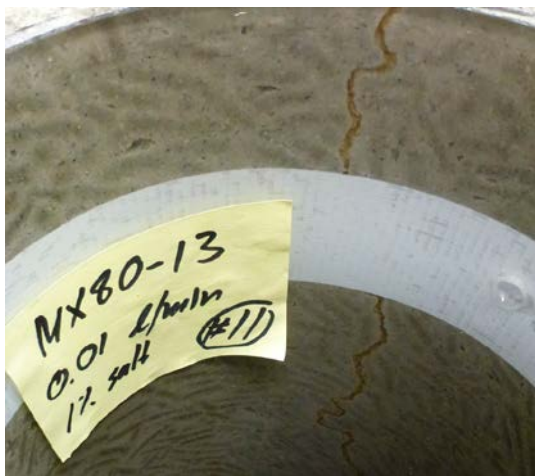
Figure 3-104. Test 3 at dismantling. A thin channel was found inside the slot on test dismantling.
