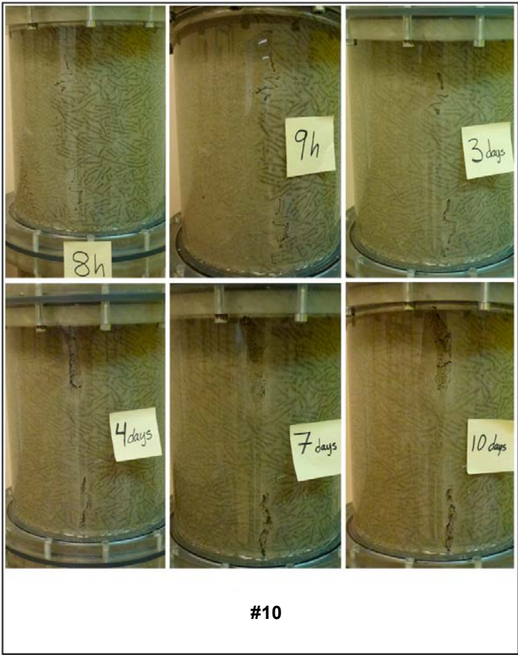
Figure 3-43. Section 3 of Test SB10. After eight hours, a disturbance is seen towards the Plexiglas surface at the left side of the tube and by day three this is healed. The channel widens around day four and remains unchanged for the remainder of the test.
