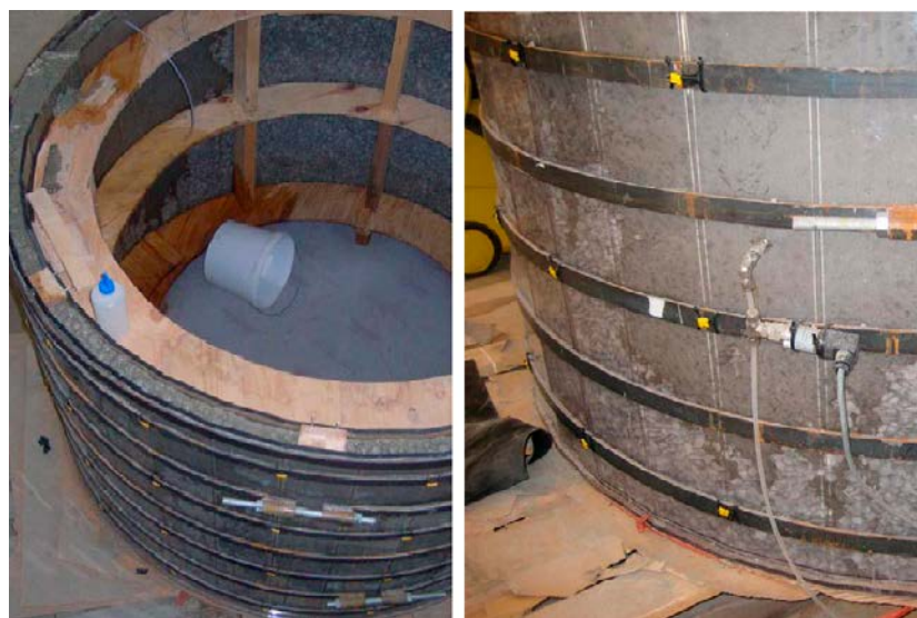
Figure 3-76. Artificial pellet slot in a deposition hole.
