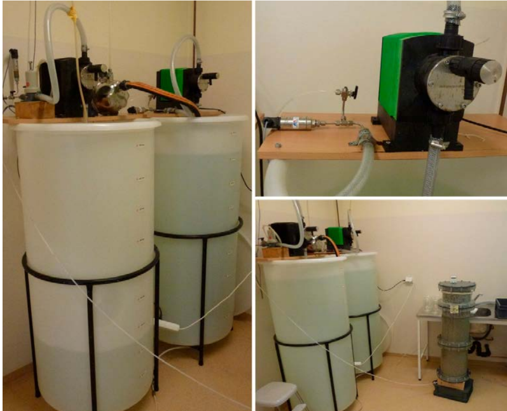
Figure 3-95. The test equipment of the erosion tests. To the left are the water tanks, to the upper right a Grundfos dosage pump and a Druck-transducer and to the lower right the fully rigged test equipment.
