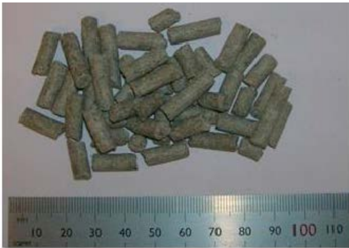
Figure 3-92. MX-80 extruded 6 mm rod-shaped pellets.
