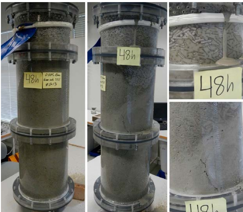
Figure 3-142. Test 13 at 48 hours. The full equipment is shown to the left and the middle. In the upper right, the top section is shown with gel extrusion through the outlet. In the lower right, a small gel-filled pocket in the mid-section is seen.
