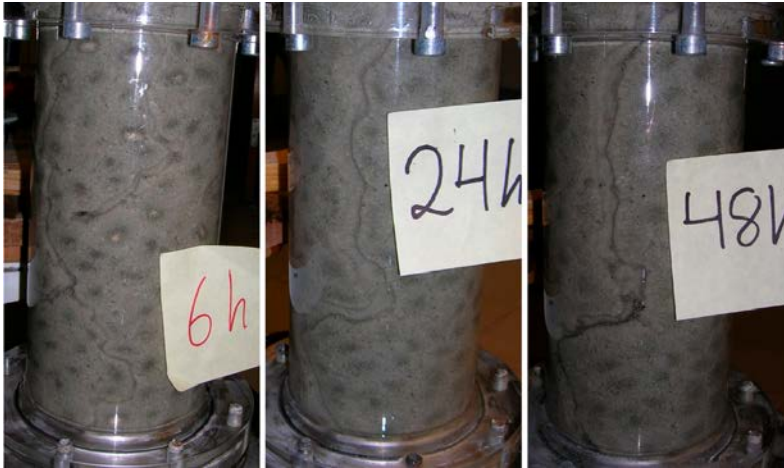
Figure 3-11. Channel forming behaviour in the tube test T1 (Pillow – 0 % salt – 0.1 L/min). Initially, there is a network of several minor channels. After 24 hours, all water runs through a single, larger channel. The smooth edges are typical for non-saline water.
