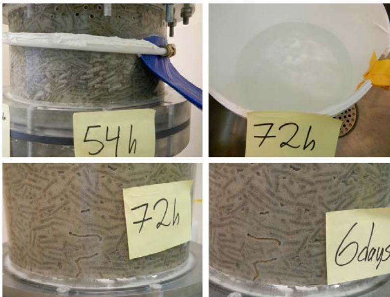
Figure 3-121. Test 8 at 54 hours, 72 hours and 6 days. The top-section was still partly dry after 54 hours. Hardly any eroded material was observed and by 72 hours the sediment trap was almost completely empty. The only visible channel was stable and unchanged for the entire test.
