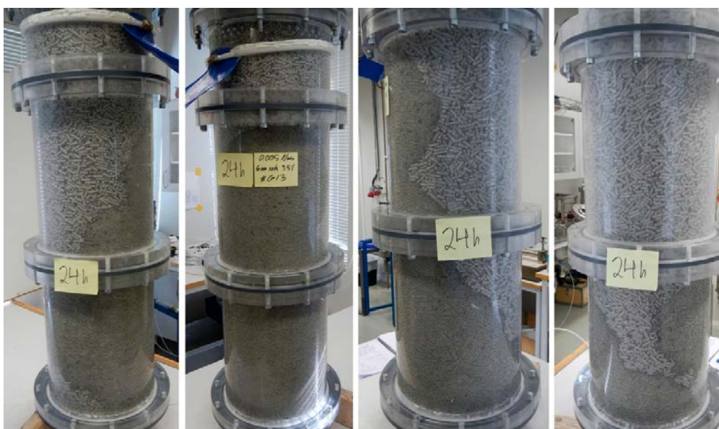
Figure 3-139. Test 13 at 24 hours viewed from all directions. The water has almost reached the top but large parts of the pellets are still dry.
