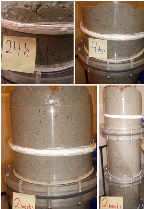
Figure 3-35. Photos from Test SA6 (6 mm rods – 1 % salt – 0.01 L/min). In this test, the flow was running over the top of the pellets and the bentonite was decomposed into bentonite-water slurry. The accumulated water at the top allowed the pellets to decompose. After two weeks, a significant part of the pellets structure had disappeared and was swelling out of the equipment slot.
