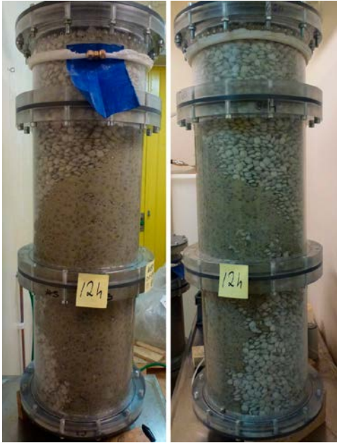
Figure 3-99. Test 2 at 12 hours. By 12 hours runtime the water has almost reached the outlet.
