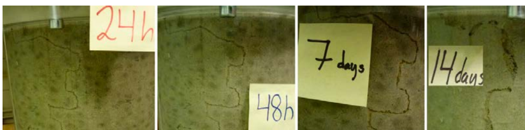
Figure 3-27. The channel formation in Test SA1 (Pillow – 1 meter – 0.01 L/min). The channel seems to widen throughout the entire test and the structure is quite grainy, especially at the end of the test.
