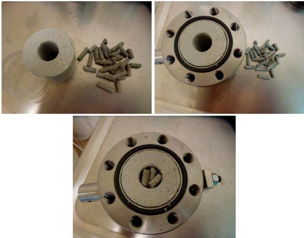
Figure 3-164. Sample preparation in the steel cylinder in set-up 2.
