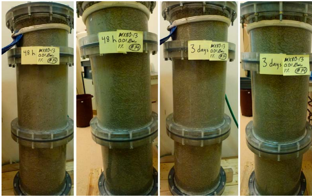
Figure 3-107. Test 4 after 48 and 72 hours. By 48 hours, the visible pellet structure is smeared out against the Plexiglas. By 72 hours, the visible structure is regained.
