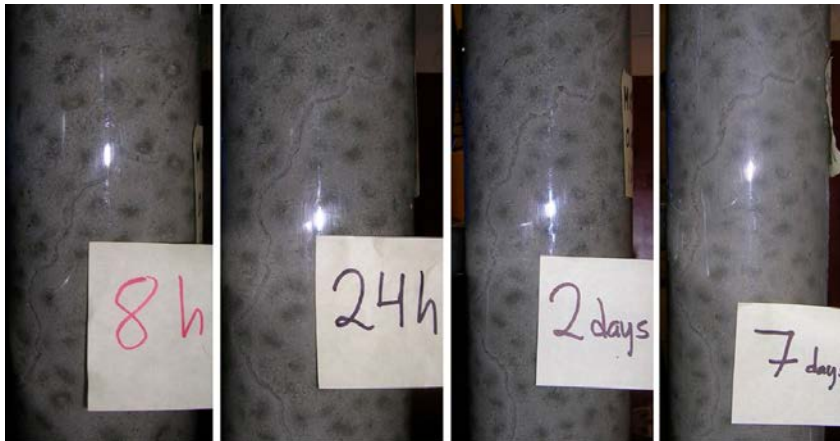
Figure 3-14. Channel forming behaviour in the tube Test T4 (Pillow – 1 % salt – 0.01 L/min). A thin channel is formed early in the test. The channel is stable and does not seem to widen as the test progresses.
