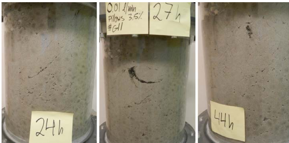
Figure 3-135. The mid-section of test 11 at 24 hours, 27 hours and 44 hours. The outflow is completely sealed from about 24 hours and 30 minutes and a gel- and water-filled pocket is formed. By 44 hours, the flow seems completely sealed and the equipment is increasingly leaking. The test is terminated.
