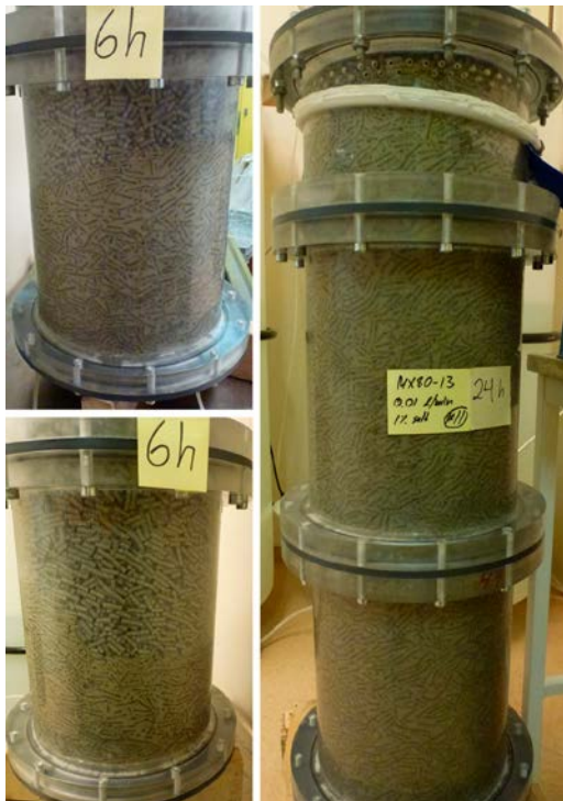
Figure 3-103. Test 3 at 6 hours and 24 hours. At 6 hours, the water front reaches all the way around the circular slot. By 24 hours the water reaches the outflow in the top and the entire amount of pellets is wetted.
