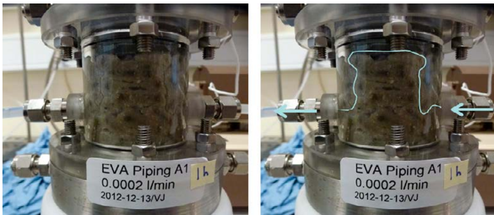
Figure 3-73. Illustration of the pipe developed in test A1. The pipe and the flow direction are elucidated in the right photo.
