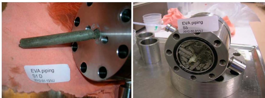
Figure 3-58. Material was punched out through the top hole at the end of tests S1 and S5.
