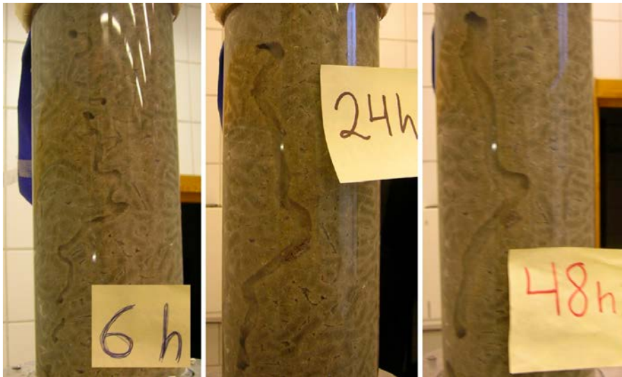
Figure A1-3. Channel formation in Test T1 (6 mm rods – 0 % salt – 0.1 L/min). Initially, there is a network of several minor channels. After 24 hours all water runs through a single larger channel. The smooth edges are typical for 0 % water salinity.
