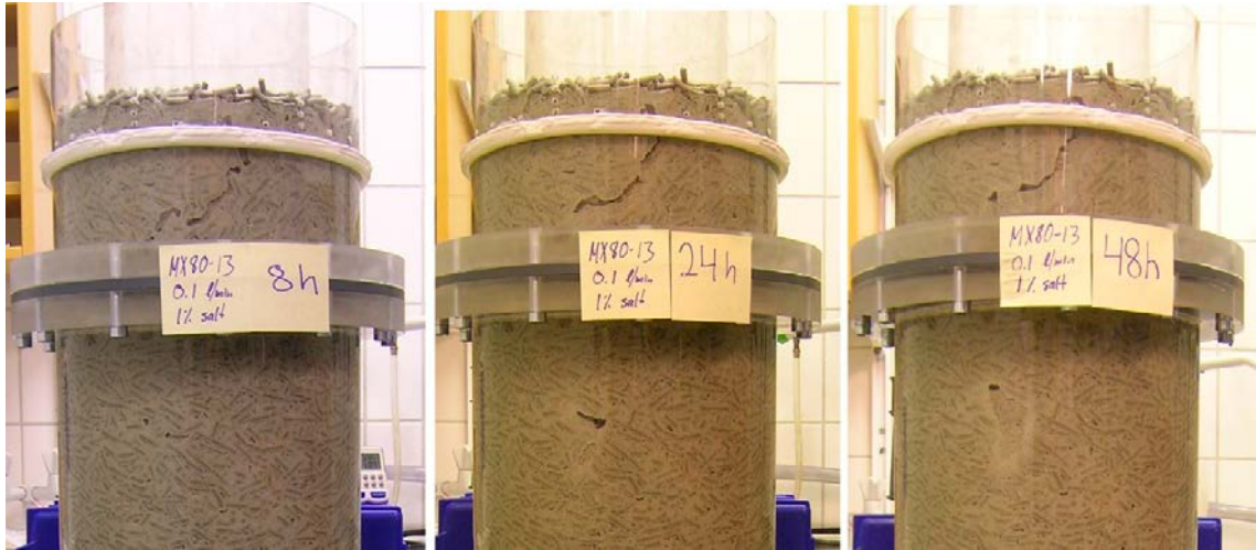
Figure A1-13. Channel forming in Test SA7 (6 mm rods – 1 % salt – 0.1 L/min). A thin channel is formed early in the test. The channel is widening throughout the entire test. It is also seen how a pocket seem to form with loose aggregates swirling in the flow.
