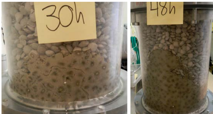
Figure 3-131. Test 10 at 30 hours and 48 hours. The visible channel that appeared to the left has clogged and sealed by 48 hours.
