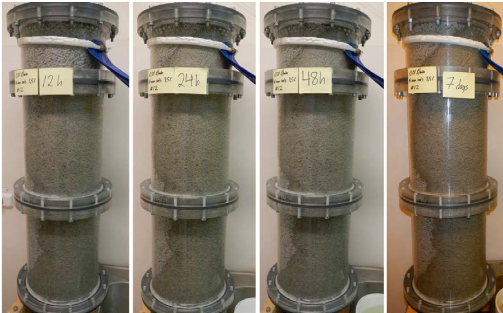
Figure 3-137. Test 12 at 12 hours, 24 hours, 48 hours and 7 days. The water front has moved mainly upwards and the outflow starts sometime shortly after 12 hours. After 24 hours, about 2/3 of the pellets are wetted and no more changes are observed. The test is terminated after 7 days.
