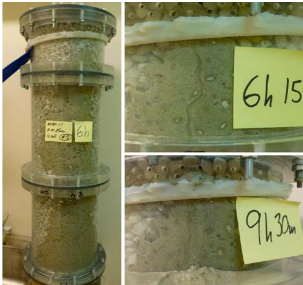
Figure 3-96. In test 1 the wetting was directly oriented upwards and after 6 hours of test run time the water had reached the top section of the equipment. By 6 hours and 15 minutes, loose material was seen in the channel at the top section and by 9 hours and 15 minutes gel extrusion through the outlet had occurred.
