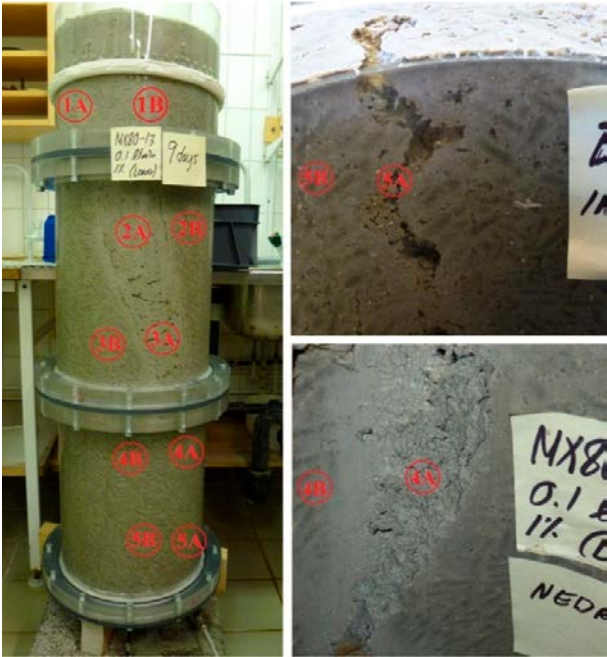
Figure 3-32. Sampling positions for the grain size distribution analysis for Test SA8 (6 mm rod – 1 meter – 0.1 L/min – long term). Note that the equipment is placed upside-down in the photos on the right of the figure.
