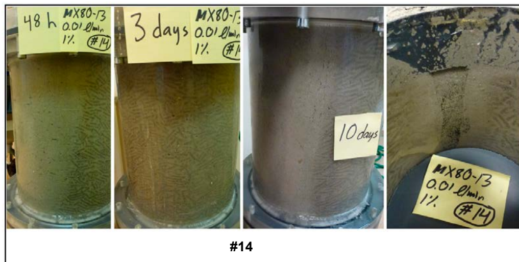
Figure 3-49. Test SB14. On day two, there was a disturbance in the surface between the pellets and the Plexiglas. By day three the disturbance seemed to have healed, but by day ten the pellets started to disperse into a several centimetre wide channel, which caused gel extrusion. At dismantling, a wide channel was clearly seen inside the slot.
