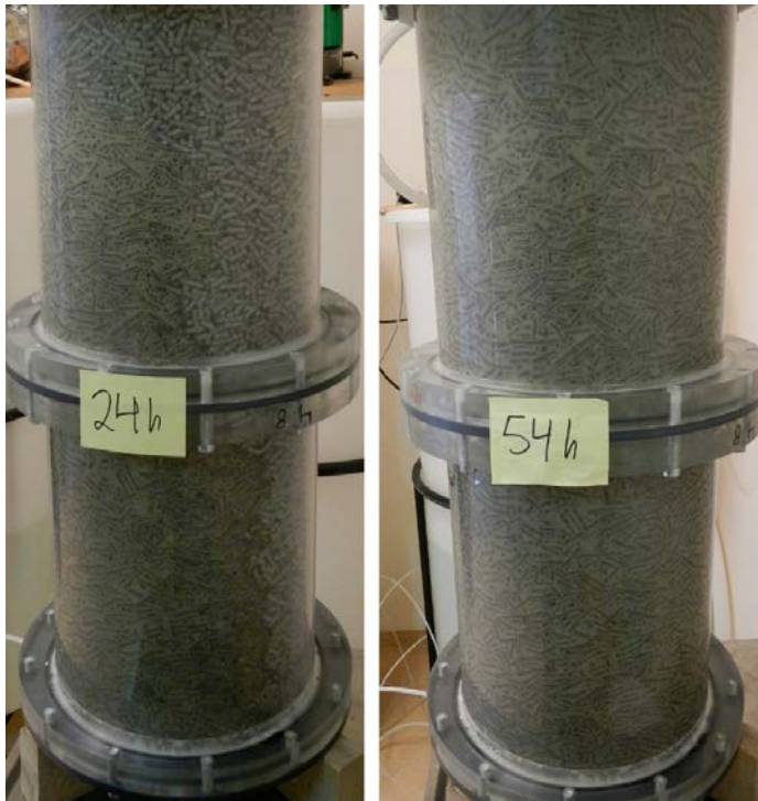
Figure 3-120. Test 8 at 24 hours and 54 hours. By 24 hours, the water front was oriented upwards and only a part of the pellets were wetted. By 54 hours, all pellets in the bottom- and mid-section were wetted.
