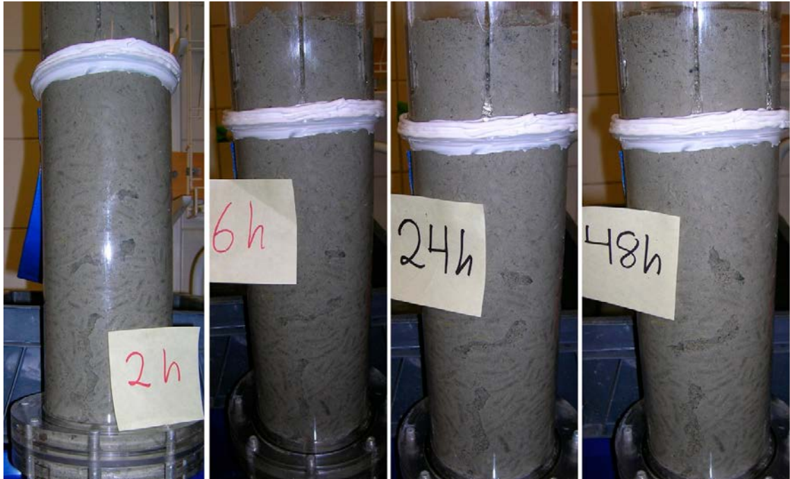
Figure A1-5. Channel-forming behaviour in Test T3 (6 mm rods – 3.5 % salt – 0.1 L/min). A wide channel with a lot of loose material is quickly formed. The channel seems rather unstable and has a very grainy structure.
