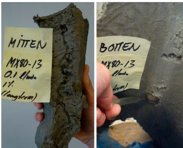
Figure 3-7. Photo documentation of sampled material at test dismantling.
