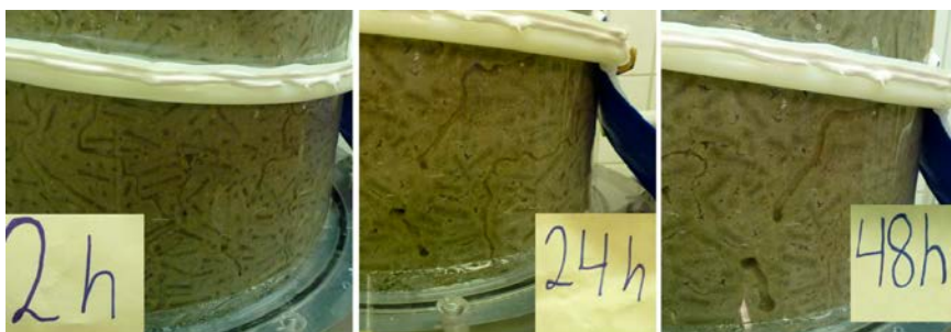
Figure 3-19. Channel formation in Test SA10 (6 mm rod – 0.4 meter – 0.1 L/min – NaCl). Initially, there is a network of smaller channels, but at the end of the test, all water flows through one major channel. The channel structure has smooth edges.
