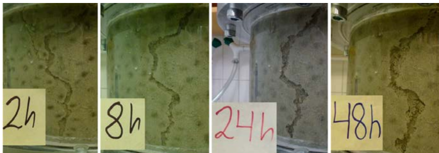
Figure 3-22. Channel formation in Test SA5 (Pillow – 0.4 meter – 0.1 L/min – CaCl 2 ). The channel is formed early and widens throughout the entire test. A lot of loose material is present in the channels and the edges look grainy and fragile.
