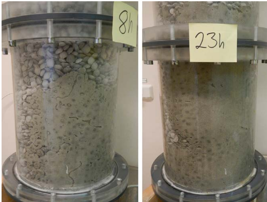
Figure 3-144. Test 14 at 8 hours and 23 hours. By 8 hours, the water has mainly moved upwards and a channel is clearly seen. By 23 hours, most of the bottom-section and the lower part of the mid-section is wetted. By 23 hours, the channel has clogged and the pellets start to disperse.
