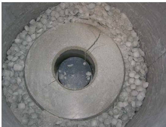
Figure 3-78. Pictures taken during excavation of tests with very low inflow rates. The total volume of macro pores in the pellet filling was 18 L.
