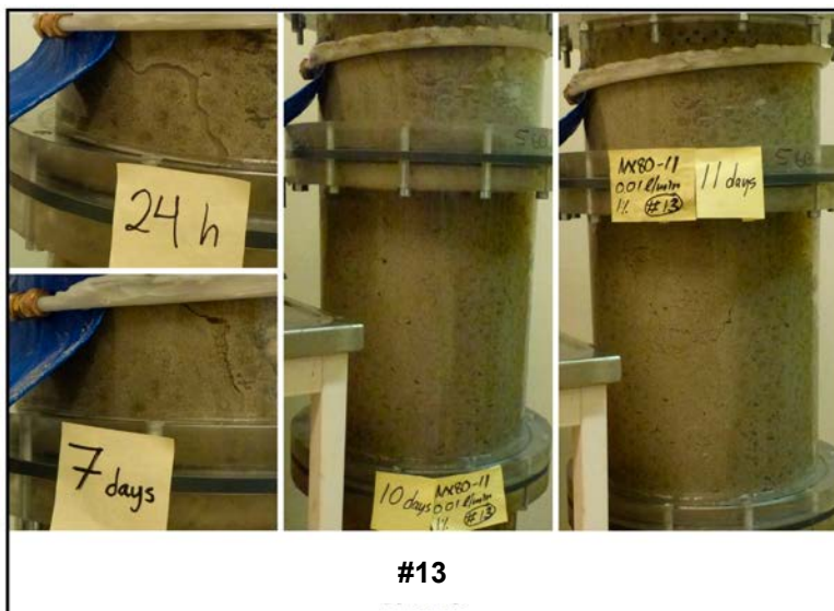
Figure 3-51. Test SB13 had a stable channel for the first seven days. By day ten, the pellets had started to disperse into a wide channel and a gel- and water filled pocket was observed. Gel extrusion occurred through the outlet and on day eleven the test was terminated.
