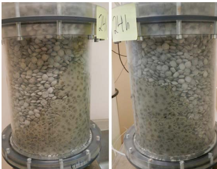
Figure 3-129. Test 10 at 24 hours. The wetting mainly progresses upwards.
