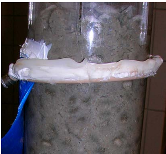
Figure 3-15. The top of the tube equipment. The outflow runs through a number of 2–3 mm slits. The photo is taken from Test T1.
