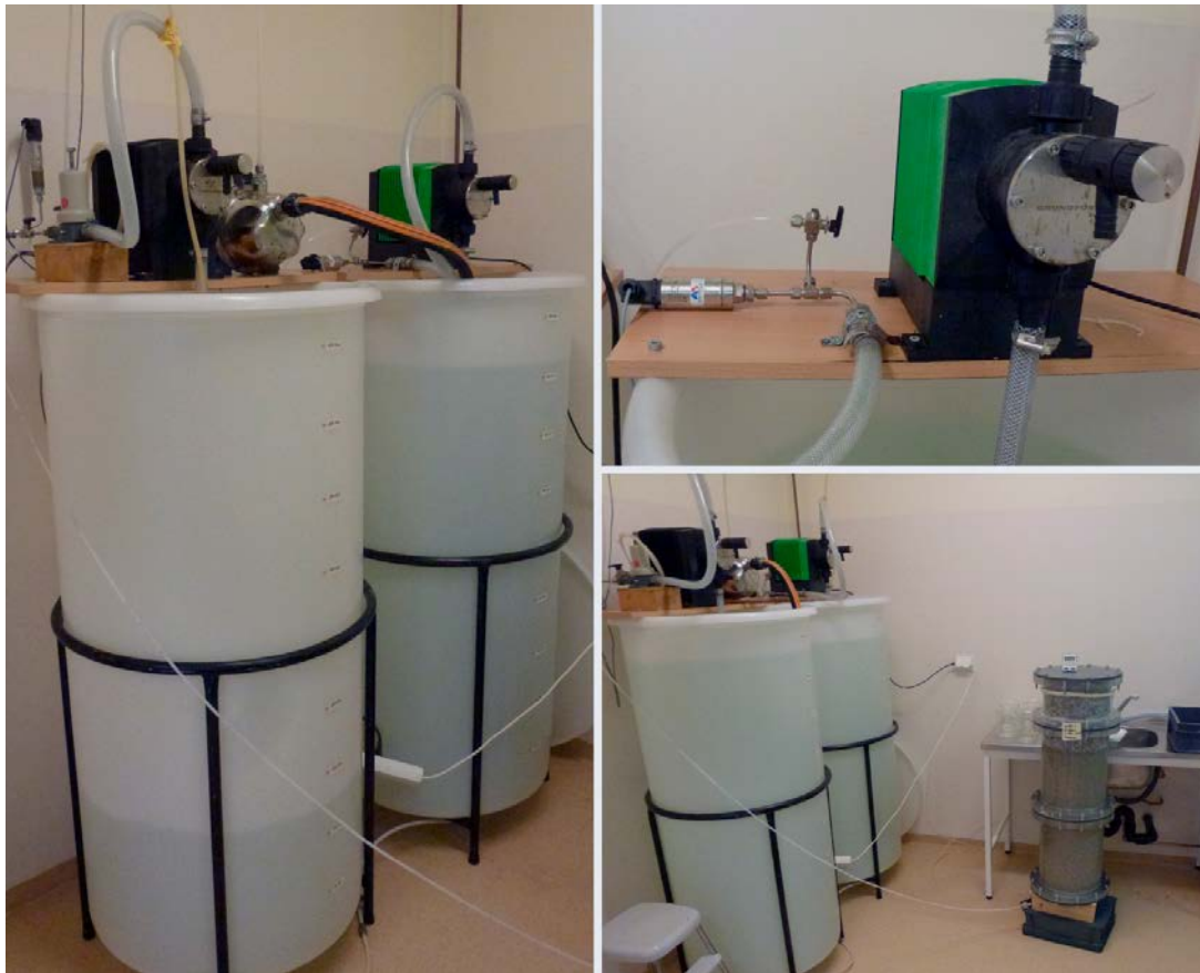
Figure 3-6. The test equipment of the erosion tests. To the left the water tanks, to the upper right a Grundfos dosage pump and a Druck-transducer and to the lower right the fully rigged test equipment are shown.
