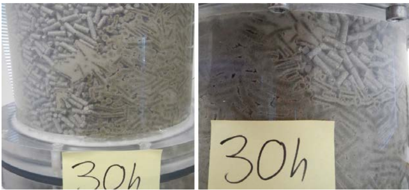
Figure 3-141. Test 13 at 30 hours. Piping with water containing dispersed bentonite occurs in several places between 24 hours and 30 hours.
