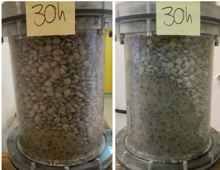
Figure 3-130. Test 10 by 30 hours. A new wet section with a visible channel has occurred to the left.
