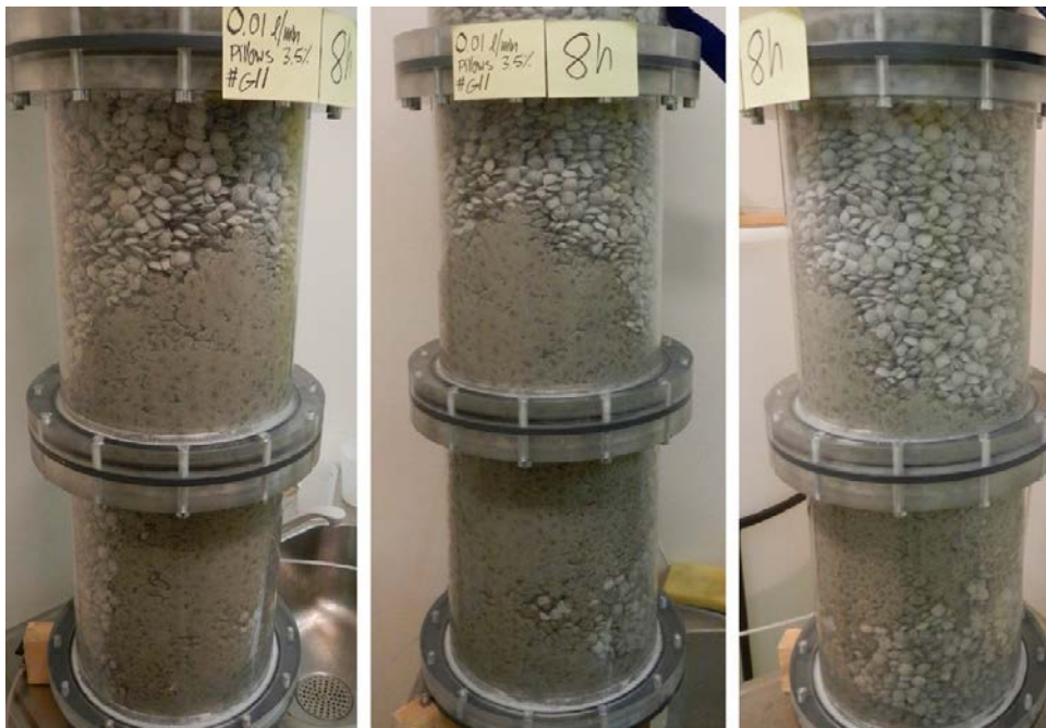
Figure 3-133. Test 11 at 8 hours. The water front has mainly moved upwards.
