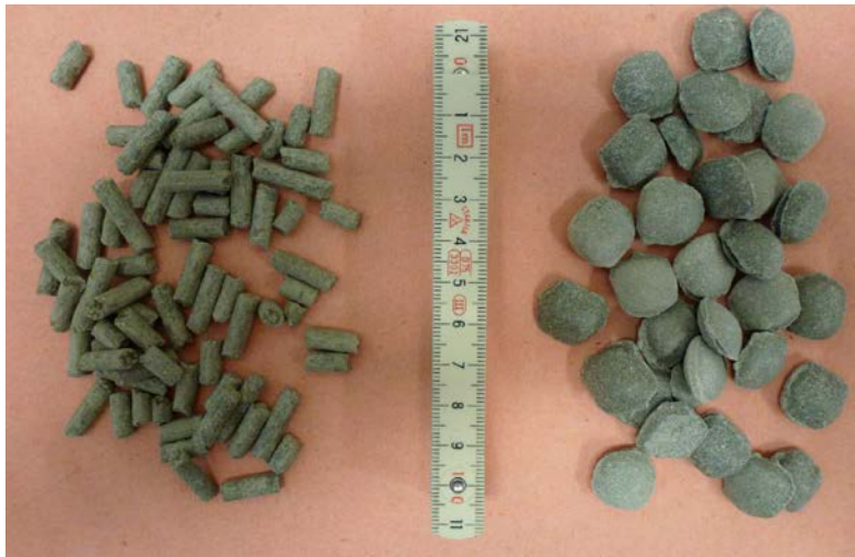
Figure 3-149. Pictures of the two pellet types used for the tests. The left type is extruded 6 mm rods and the right type is roller-compacted, pillow-shaped pellets (see also Section 3.2.2).
