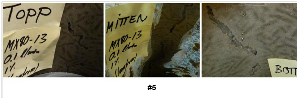
Figure 3-41. At the dismantling of Test SB5, a second channel was found inside the circular slot.
