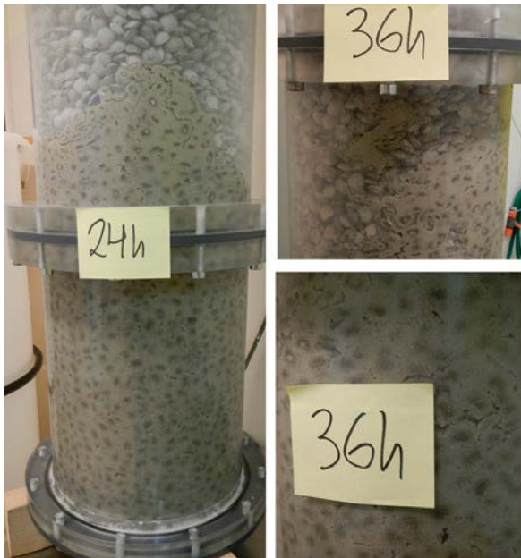
Figure 3-113. Test 6 by 24 hours and 36 hours. A short part of the channel is visible in the upper part of the wetted pellets. By 36 hours, wetting occurs in patches and loose material is visible in the channel.
