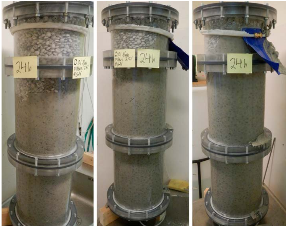
Figure 3-134. The test at 24 hours. A wide channel with dispersed material is observed in the mid-section. The outflow started around 23 hours 30 minutes and mainly consisted of gel.
