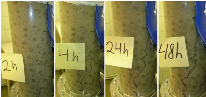
Figure 3-12. Channel forming behaviour in the tube Test T2 (Pillow – 1 % salt – 0.1 L/min). The flow is concentrated to one channel quite early. The channel seems to widen as the test progresses and the structure is grainier than when using non-saline water.
