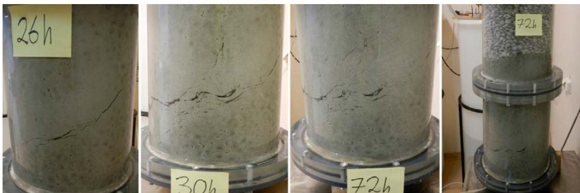
Figure 3-145. Test 14 at 26 hours, 30 hours and 72 hours. By 26 hours the channel has widened and the pellets start to disperse and separate. By 30 hours it looks like a water- and gel filled pocket is forming. No more changes are observed and the test is terminated by 72 hours.
