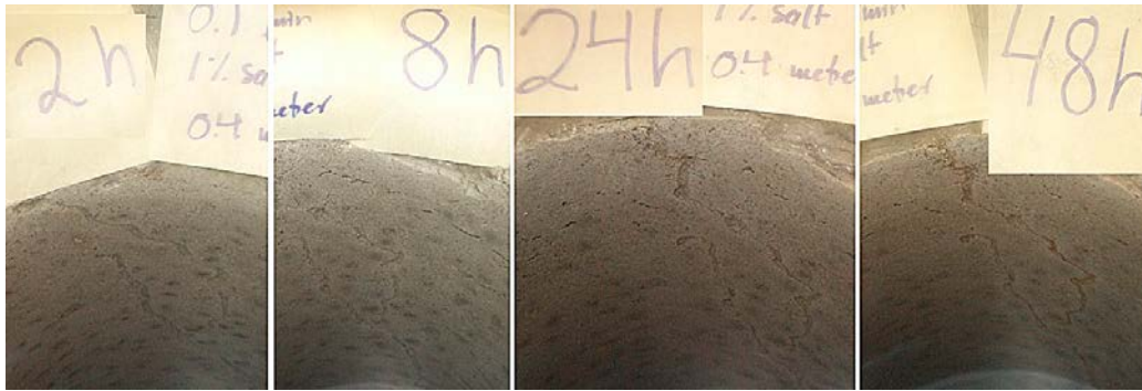
Figure 3-25. Channel formation in Test SA3 (Pillow – 0.4 meter – 0.1 L/min). The channel branches out early and persists throughout the whole test. The structure is slightly grainy and the channel is somewhat wider than in the 6 mm rod test.
