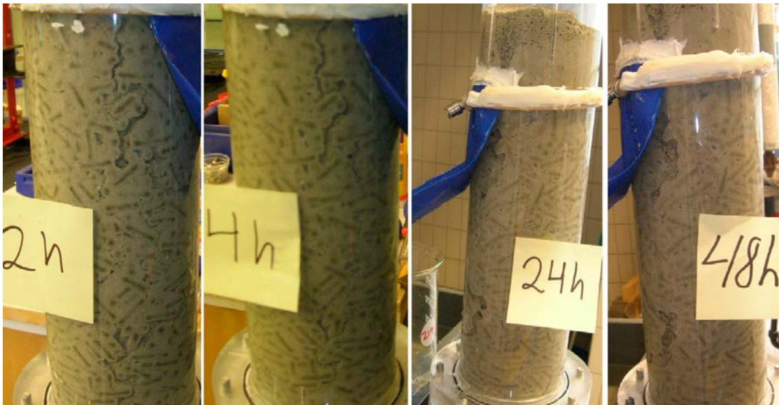
Figure A1-4. Channel-forming behaviour in Test T2 (6 mm rods – 1 % salt – 0.1 L/min). The flow is concentrated to one channel quite early, but at some point after 4 hours the flow path way is changed to the other side of the tube. The channel seems to widen as the test progresses and the structure is grainier than when using water with 0 % salinity.
