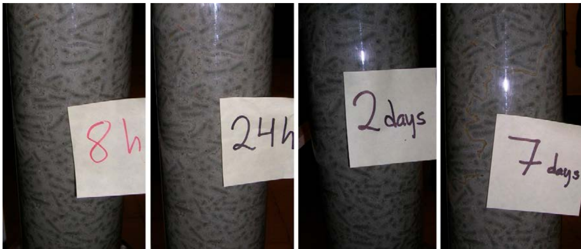
Figure A1-6. Channel-forming behaviour in Test T4 (6 mm rods – 1 % salt – 0.01 L/min). A thin channel is formed early in the test. The channel is stable and does not seem to widen as the test progresses.
