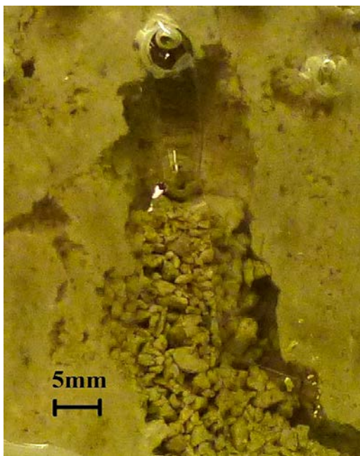
Figure 3-23. Aggregates are formed in the tests with calcium chloride water. The water velocity is normally insufficient to lift the aggregates out of the channel. The photo is taken from Test SA11 (6 mm rod – 0.4 meter – 0.1 L/min – CaCl 2 ).
