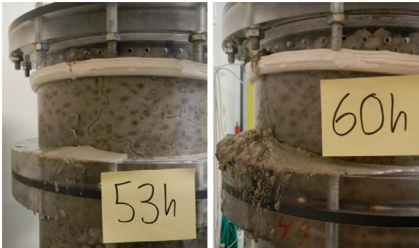
Figure 3-115. Test 6 photos from 53 hours and 60 hours. By 53 hours, gel extrusion starts to occur again and by 60 hours the test is terminated.
