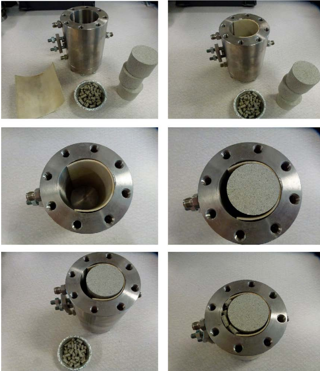
Figure 3-81. Set-up and mounting of specimen in the study of the ability of the bentonite to stop piping (process 4A).
