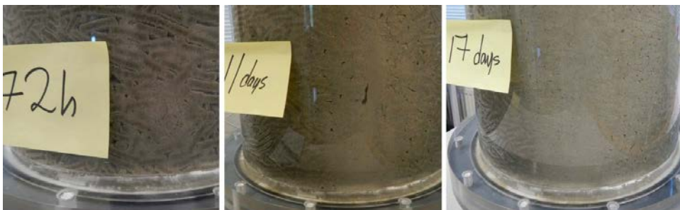
Figure 3-126. Photos of the inlet taken at 72 hours, 11 days and 17 days. It is seen how the pellets just above the inlet are dissolving as the test progresses.
