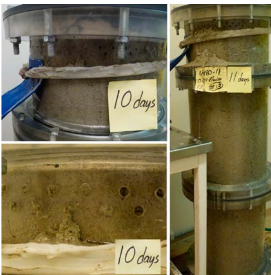
Figure 3-101. After 10 days, gel extrusion is observed through the test outlet and by day 11 a large part of the pellets in the top- and mid-section are dispersed and squeezed out of the equipment.
