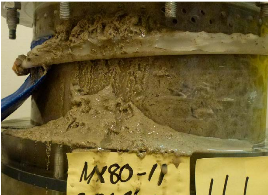
Figure 3-54. Both tests with pillow-shaped pellets at the flow rate 0.01 L/min were stopped due to gel extrusion. Test SB13 is seen in the picture and was terminated on day 11 since it was no longer possible to sample the outflow.
