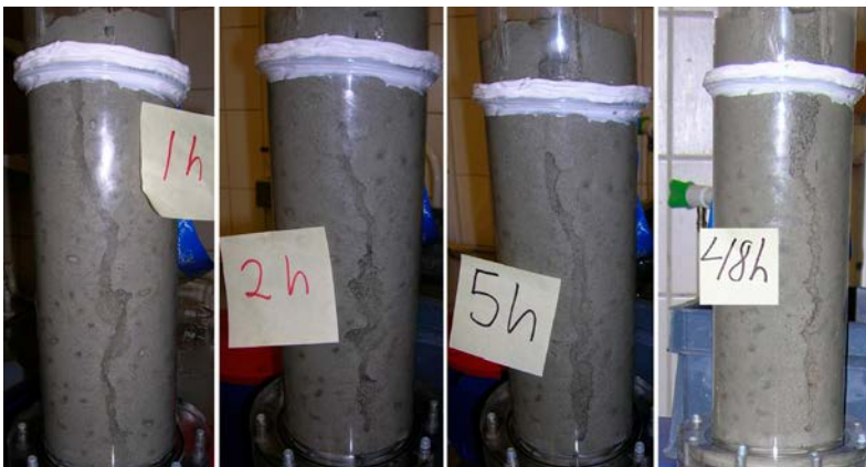
Figure 3-13. Channel forming behaviour in the tube Test T3 (Pillow – 3.5 % salt – 0.1 L/min). A wide channel with a lot of loose material is quickly formed. The channel seems rather unstable and has a very grainy structure.
