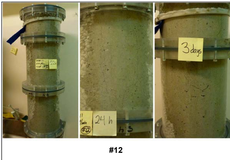
Figure 3-50. In Test SB12, the water moved almost straight upwards and left large parts of the pellets dry. Within 24 hours, the pellets in the flow path started to disperse into a wide channel. After about three days, gel-extrusion occurred through the equipment outlet and the test was terminated.
