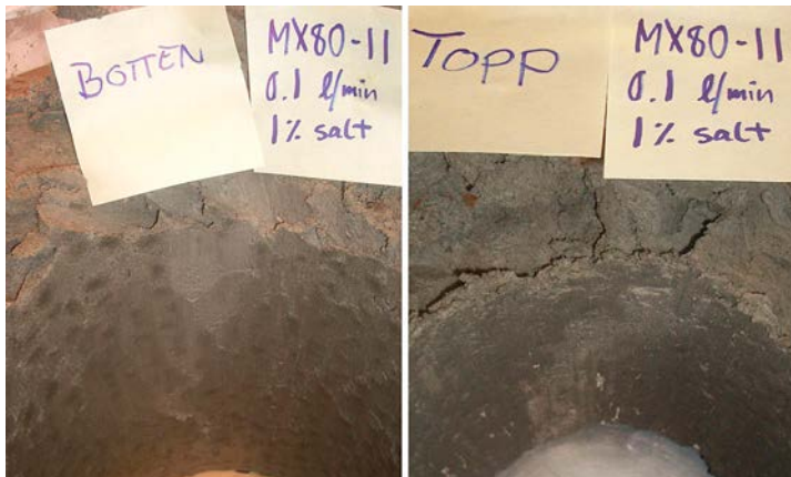
Figure 3-26. The channel in Test SA2 (Pillow – 1 meter – 0.1 L/min) was located inside the equipment. To the left is the inflow point and to the right is the top. Note that the equipment is placed upside down. Although it is hard to evaluate, the channel seems somewhat wider at the inflow point and the top.
