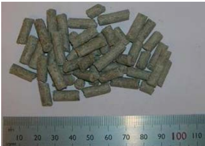
Figure 3-1. Extruded 6 mm rod-shaped pellets (MX-80-13).
