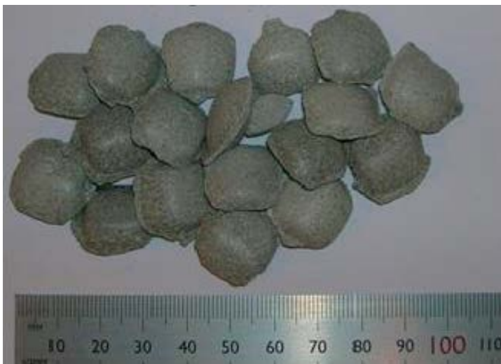
Figure 3-2. Compacted pillow-shaped pellets (MX-80-11).
