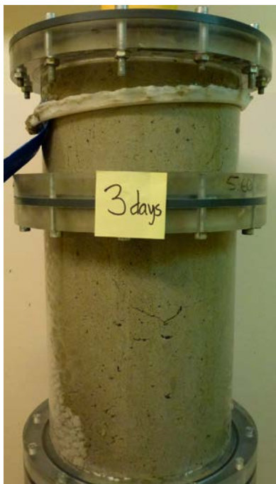
Figure 3-97. Test 1 after 72 hours. A very large amount of the pellets in the mid- and top section is dispersed and being squeezed out of the equipment outlet. A part of the mid- and top-section is considered a gel-filled pocket. The test was terminated after about 72 hours.
