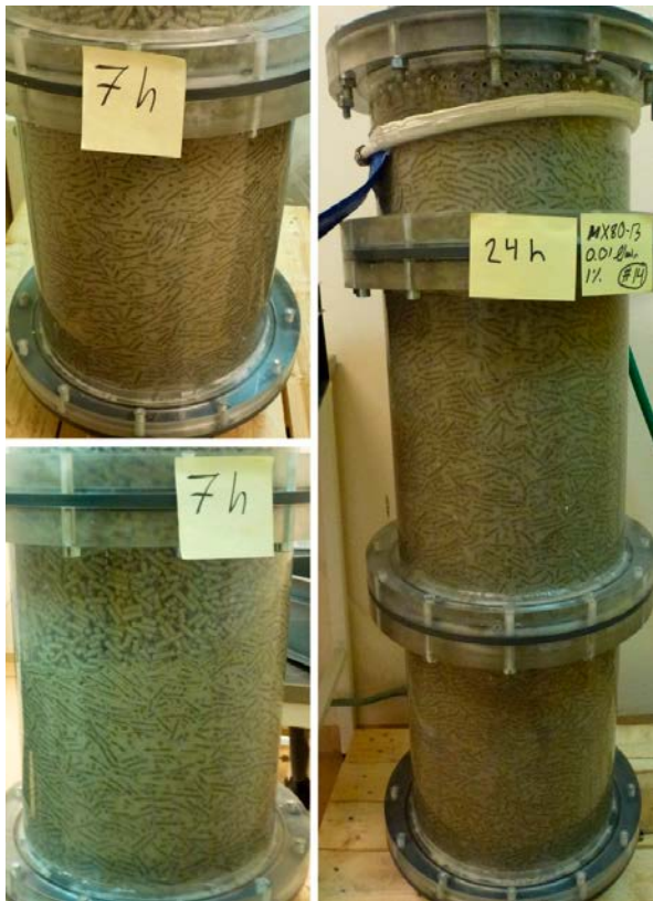
Figure 3-106. Test 4 after 7 and 24 hours. By 24 hours, the equipment is filled and the water reaches the outlet.
