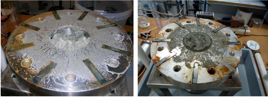
Figure 3-155. Pictures taken from finished tests after removal of the upper lid of the artificial fracture of tests 12 (left) and 16 (right).
