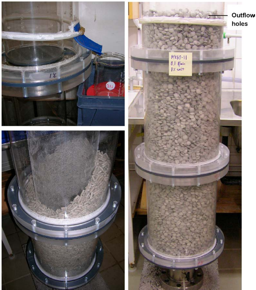
Figure 3-4. Circular slot test: type-A equipment. The upper left shows the top of the equipment, the lower left a half filled equipment and the right a fully prepared test.
