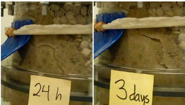
Figure 3-100. Test 2 after 24 hours and after 3 days. A stable channel is seen in the top section after about 24 hours. By 72 hours, the channel has widened somewhat and some loose material can be seen.
