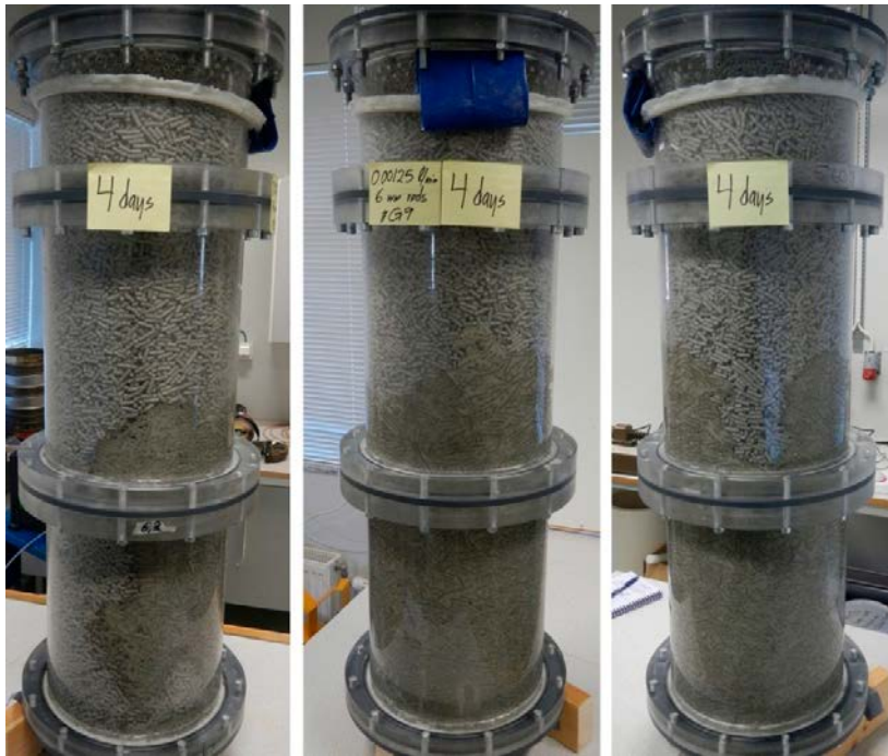
Figure 3-123. Test 9 at day 4. The water has reached half way up the mid-section. A large part of the pellets are still dry in the bottom section.
