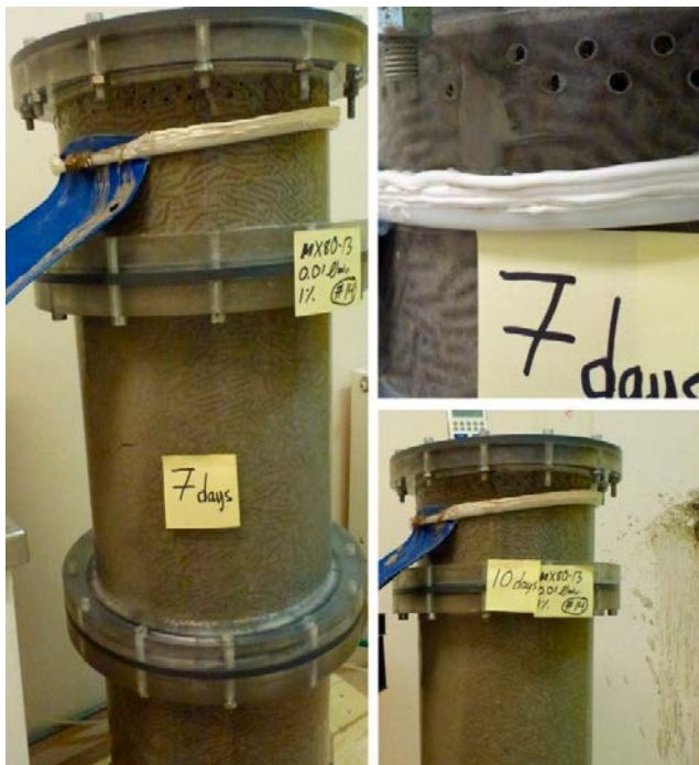
Figure 3-108. Test 4 on day 7 and 10. By day 7, a channel is visible and the surrounding material is starting to disperse. Material is clearly seen in the outflow. By day 10, gel extrusion starts to occur when bentonite gel is splashed out through a new outlet hole.
