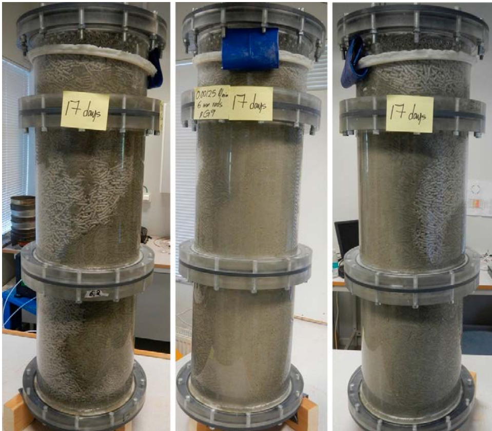
Figure 3-125. Test 9 at day 17. By day 17 it looks like a large part of the pellets have started to disperse.
