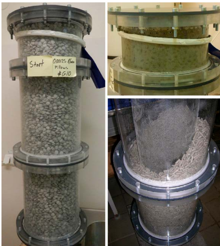
Figure 3-94. Circular slot type-B equipment. The entire equipment filled with pillow-shaped pellets is seen to the left. To the upper right is the top with the lid, to the lower right is the slot half-filled with 6 mm rod-shaped pellets.
