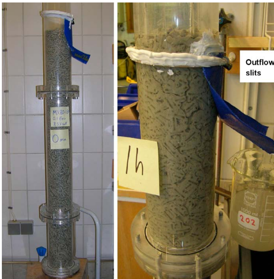
Figure 3-3. The tube test equipment. The left picture shows the full tube and the right picture shows the top part. The right photo is taken during a sampling procedure.
