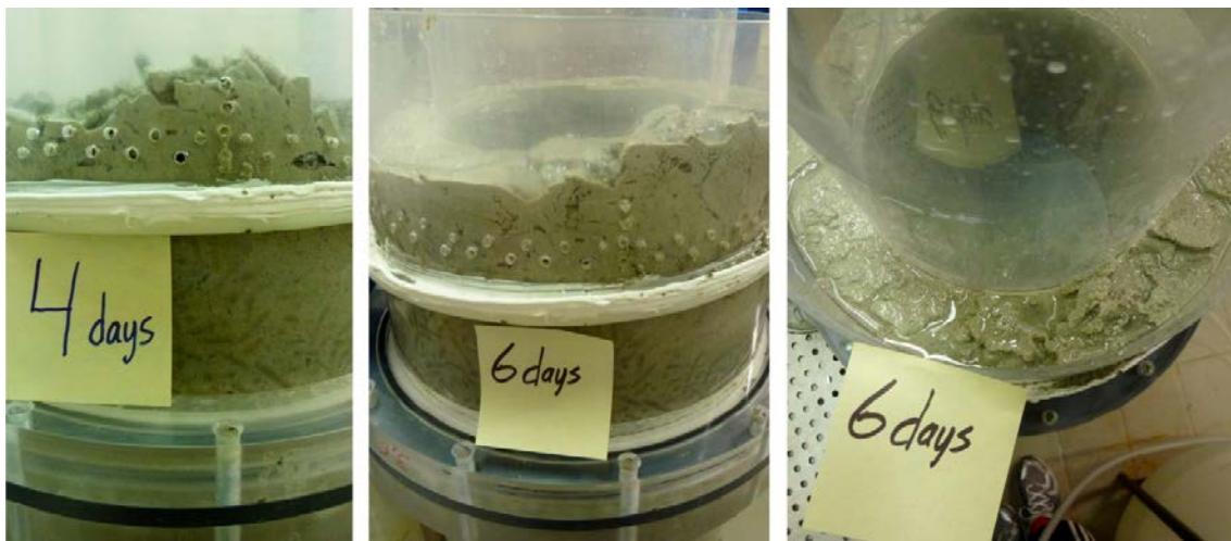
Figure 3-29. Test SA8 (6 mm rod – 1 meter – 0.1 L/min – long term). Decomposed bentonite pellets are accumulating at the top of the equipment.
