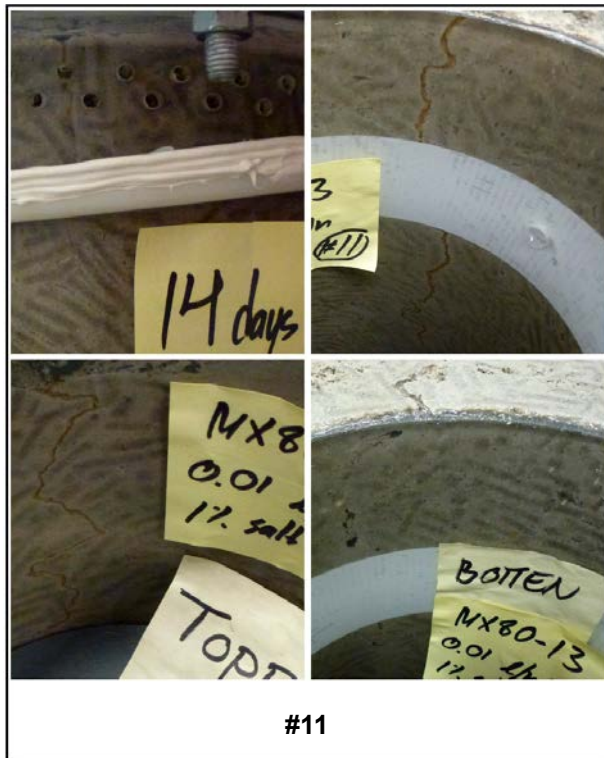
Figure 3-48. The only visible channel during Test SB11 was at the outlet. A thin channel was found inside the slot during test dismantling.
