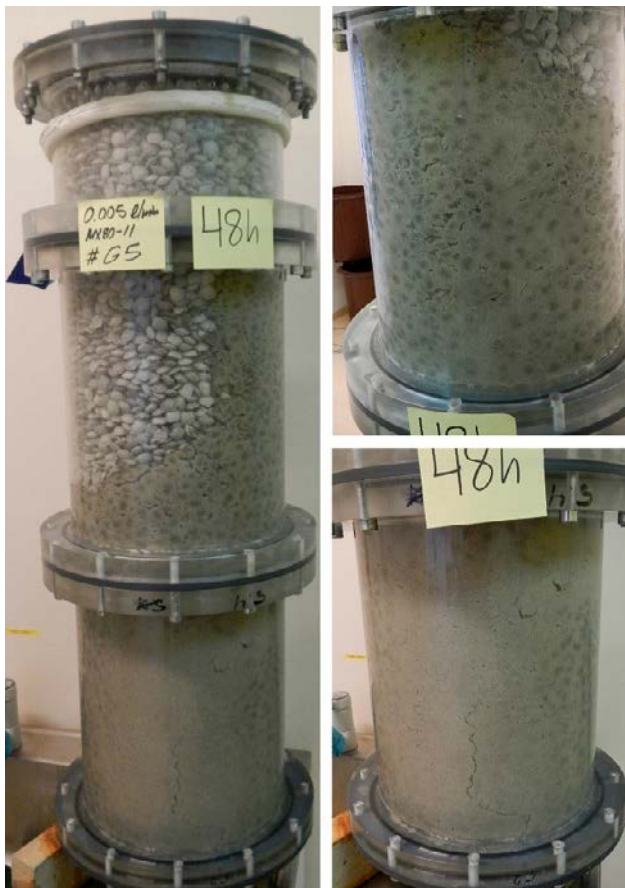
Figure 3-111. Test 5 after 48 hours. The channel in the bottom-section has widened significantly and large amounts of dispersed bentonite are seen. At this time, the channel has sealed in the mid-section and the test is terminated.
