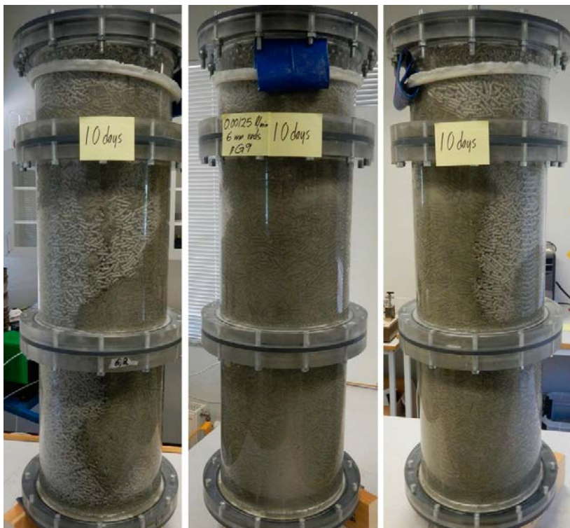
Figure 3-124. Test 9 at day 10. The water has reached the top and large parts of the pellets are still dry. No outflow has started yet.
