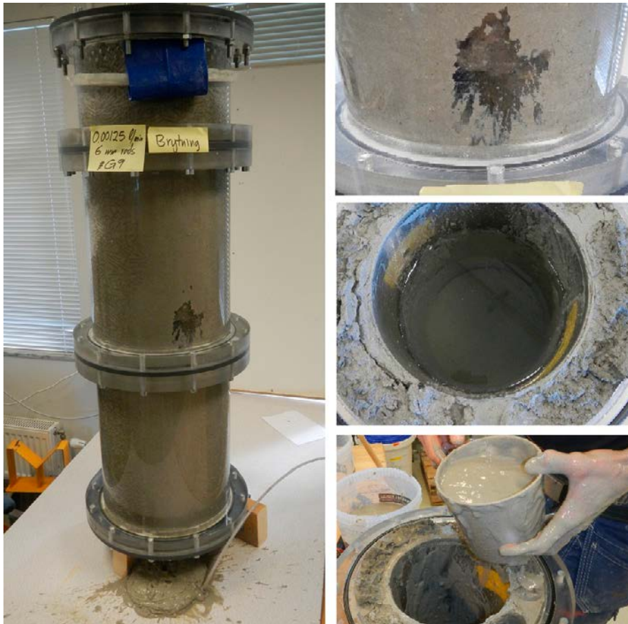
Figure 3-127. Test 9 at test termination. To the left it is seen how a large amount of gel poured out through the inlet at test dismantling. An empty visible part of the gel pocket is seen to the upper right. The mid- and lower right photos show the water and gel that had leaked into the centre tube.
