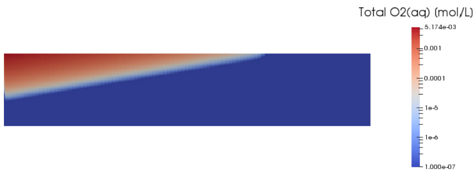
Figure 4-17. Oxygen concentration computed using iDP after 200 days of simulation time. The domain is magnified by a factor of 400 in the direction perpendicular to the fracture.
