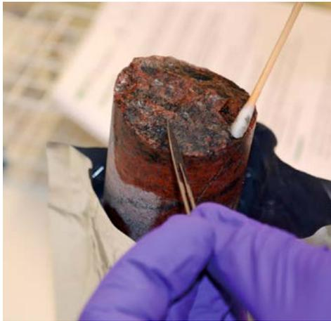
*Figure 2-2. Sampling of one of the KA3065A01 fracture surfaces showing scalpel and a viscose swab.*
