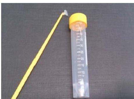
*Figure A-3. Sampling equipment for collecting loose material of mud and sand.*
