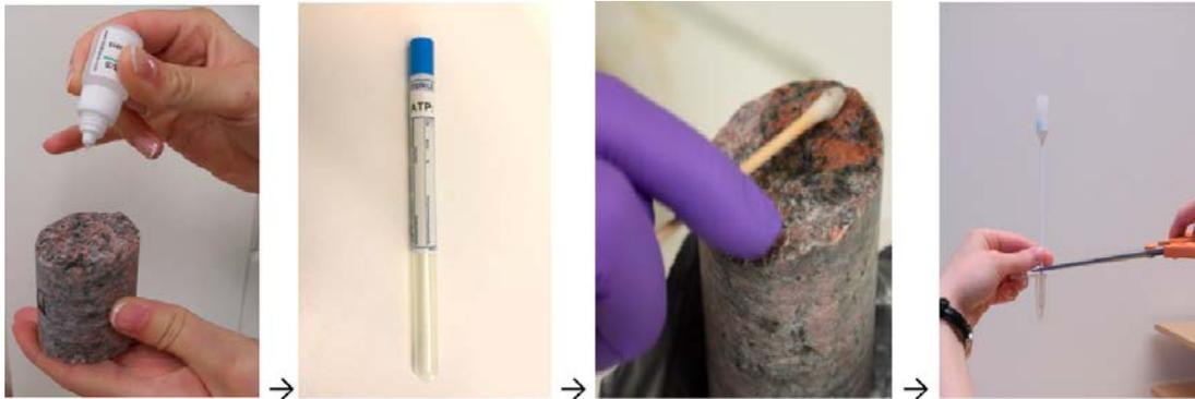
**Figure 2-3.** Sampling procedure for ATP: Add 2–3 drops from the bottle containing Extractant B/S on the surface. Rub thoroughly all over the surface with the swab marked ATP. Place the swab in the provided 1,5 mL Eppendorf tube. Cut off the swab at 2 cm from the tip and close the cap on the tube. Store the ATP samples in freezer.
