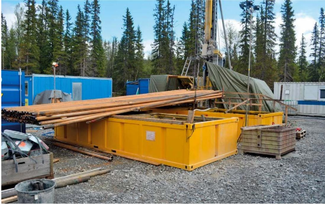
**Figure 2-1.** The COSC-1 drill site with the drill mud reservoirs in front, drill strings on top and the drill rig in the background. The blue “bugs-lab” is visible in the left background.
