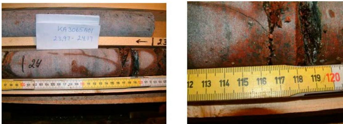
*Figure A-1. Detection and localisation of water conducting fractures in a drill core.*
