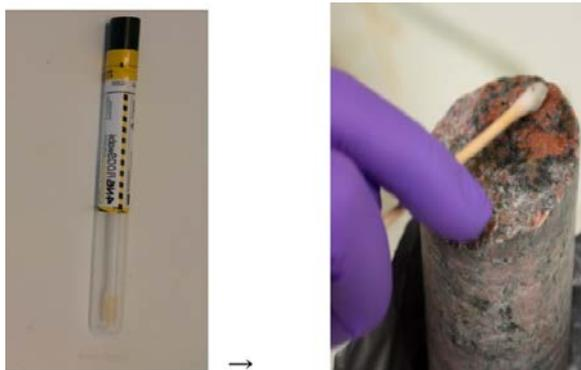
**Figure 2-4.** Sampling procedure for DNA: Sample the opposite fracture surface with the black swab for DNA. Put the swab back into the provided tube. Note the sample number on the tube and on the sampling list. Store the DNA samples in room temperature.
