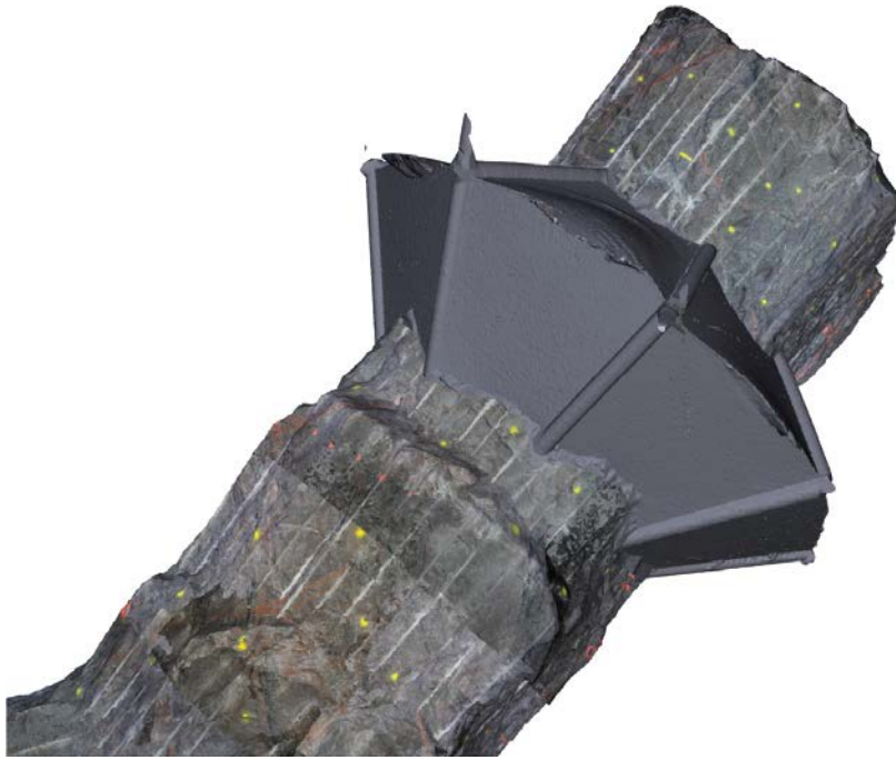
Figure 4-33. Illustrative model structured of data from laser scanning of TAS01 as well as of the excavated slot abutment (seen from above).
