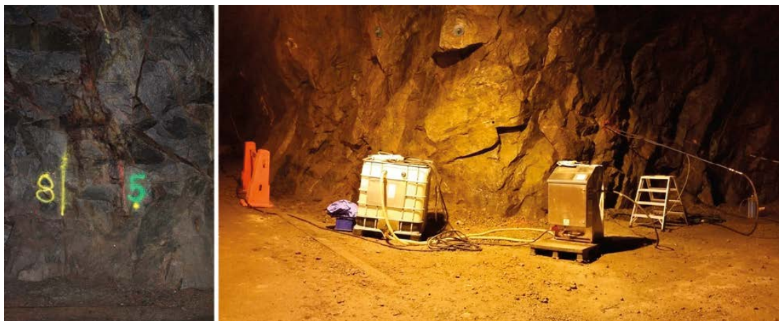
Figure 7-9. Transmissivity measurements in field (Äspölaboratoriet).
