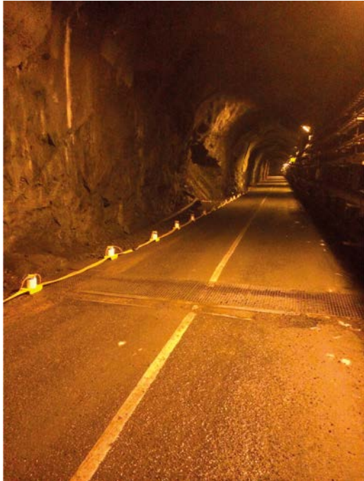
Figure 7-5. A segment of the seismic landstreamer placed on the tunnel floor in the proximity of the NE1 fracture system. The streamer uses digital-3C sensors and proved in this experiment to be free of electrical noise when compared with planted geophones on its either side in the tunnel.
