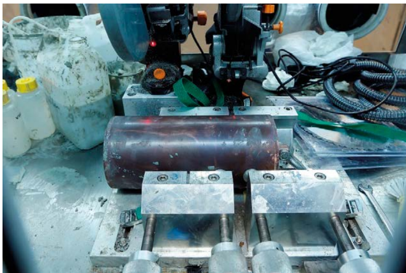
Figure 4-17. Canister before being sliced for preparation of metallographic examination.
