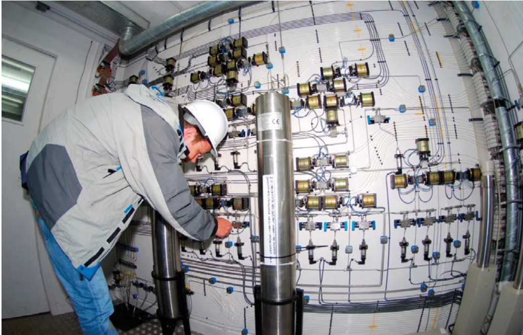
Figure 4-9. Photo of the laboratory area for the large-scale gas injection test 420 m below ground at Äspö HRL.
