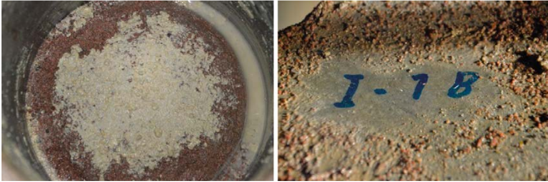
Figure 4-19. After removing the topmost layer of sand and the bentonite used to seal the deposition hole from intruding surface water the concrete cylinder is exposed. Please note that the sand-filled slit is saturated with ground water. The right figure shows the label of the concrete cylinder ensuring that the correct concrete cylinder is retrieved.
