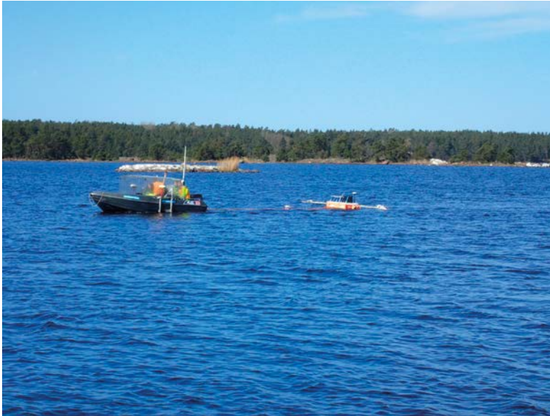
Figure 7-6. Boat-towed RMT data acquisition over the southern part of the Äspö tunnel. The system was recently modified to make the acquisition faster and more reliable using a DGPS mounted recording system. In less than 3 hours more than 5 km/line RMT data were collected.
