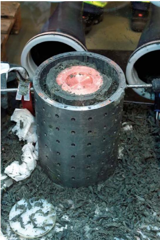
Figure 4-16. Canister of MiniCan 4 sees daylight after nearly nine years in the borehole.
