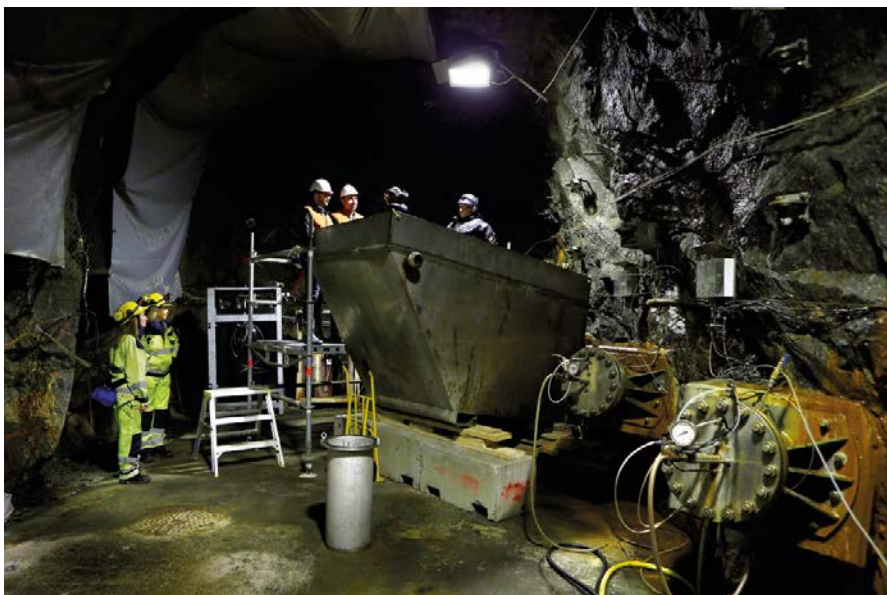
Figure 4-12. Ground water filled container docked to the borehole of MiniCan 4. The experimental package was taken out and placed in a transport flask under nitrogen saturated water in order to avoid exposure to the atmosphere.
