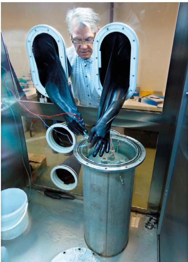
Figure 4-14. Claes Taxén from Swerea-KIMAB controlling the potential of reference electrode.
