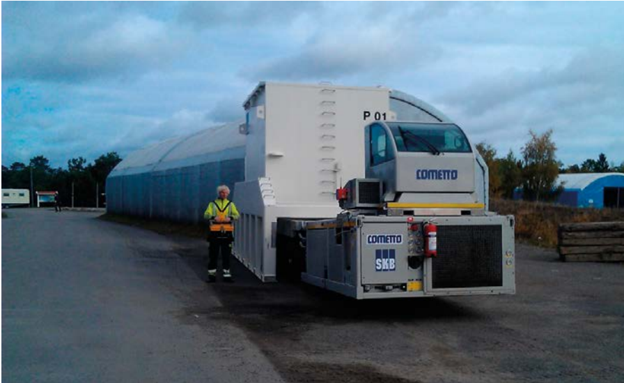
Figure 5-6. Ramp Vehicle carrying the modified ATB.
