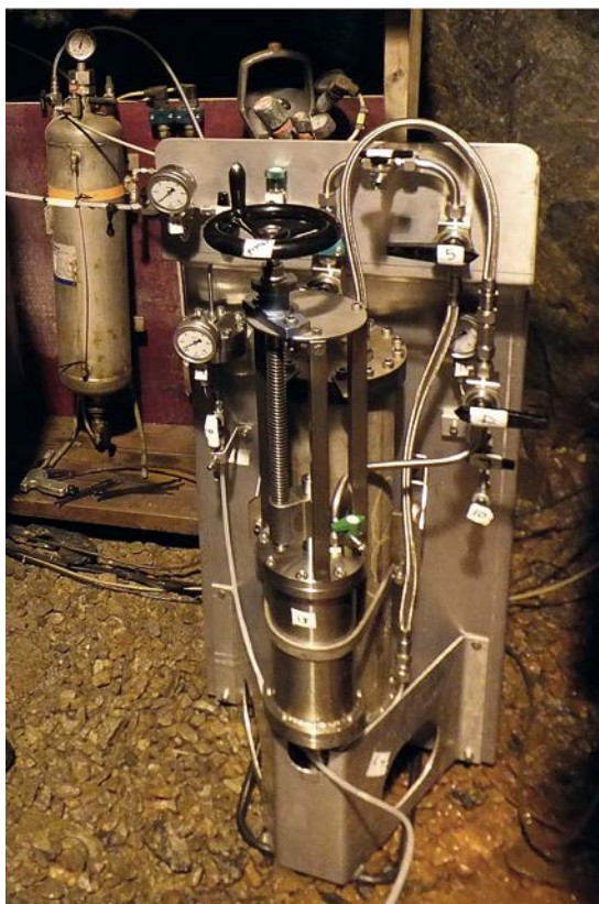
Figure 7-29. Sampling vessel for preservation of RNA from borehole water maintained under in situ conditions.
