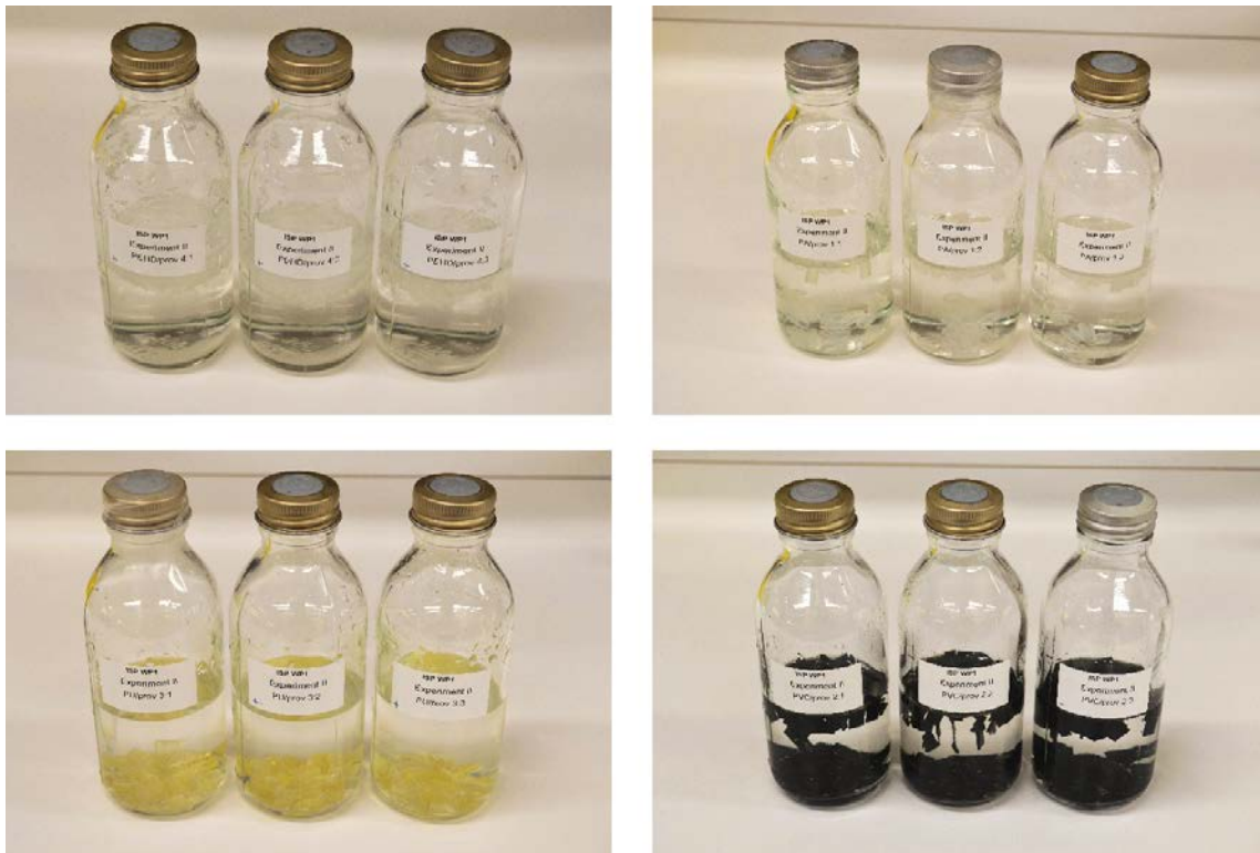
Figure 2-3. Release experiments with polymeric materials used to construct stationary borehole equipment in groundwater. Upper left, high density polyethylene; lower left, polyuretan Slitan 80A-71; upper right polyamide tubing; lower right, PVC tape.
