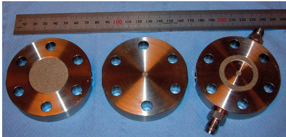
Figure 1-3. The types of fluid injection geometry adopted. A) Filter in full bottom area B) Small injection filter C) Small injection filter + circumferential outflow filter. The circumferential outflow channel is isolated from the top outflow channel.
