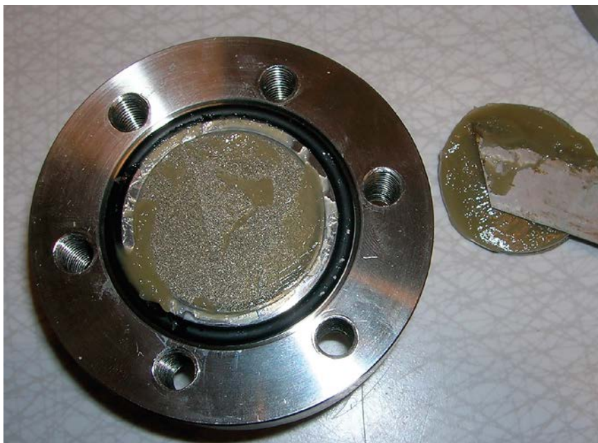
Figure 2-3. Sample GenCh02 at termination. The sample (right) is covered by the knife used to cut it from the injection filter (left). The loose – almost slurry-like – structure is clearly seen.
