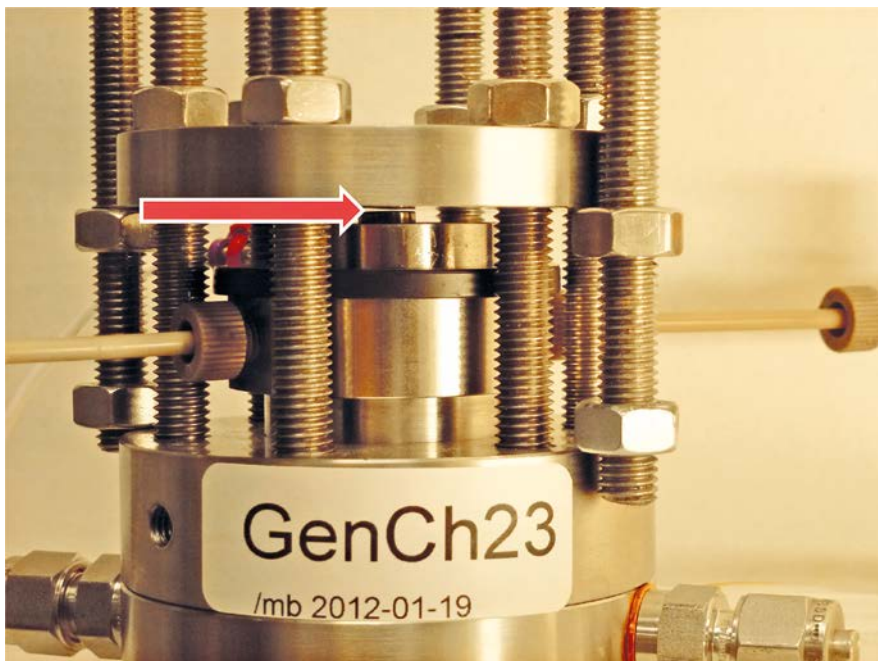
Figure 3-11. After being pressurized with air at 0.2 MPa on the injection side, the piston of the test cell could be pushed down, opening a slit between the force sensor and the top of the cell in sample GenCh23. This is a visual demonstration that air has the ability to (macroscopically) consolidate bentonite clay.
