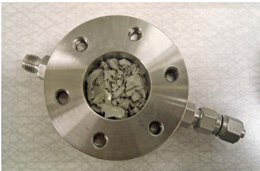
Figure 3-7. The dry Ca-montmorillonite grains used in the preparation of sample GenCh22. These were placed directly in the test cell, as shown in the picture, during preparation of the sample.
