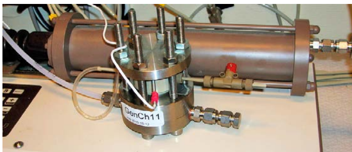
Figure 1-2. A test cell connected to a pressure controlling unit (white tube in the bottom).
