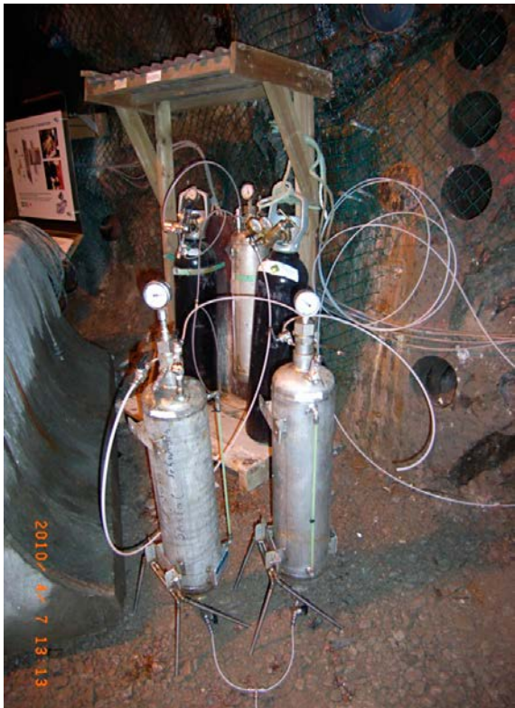
Figure 3-6. Pressurized tracer tanks and gas tube ( N_2 ) used during tracer injection.
