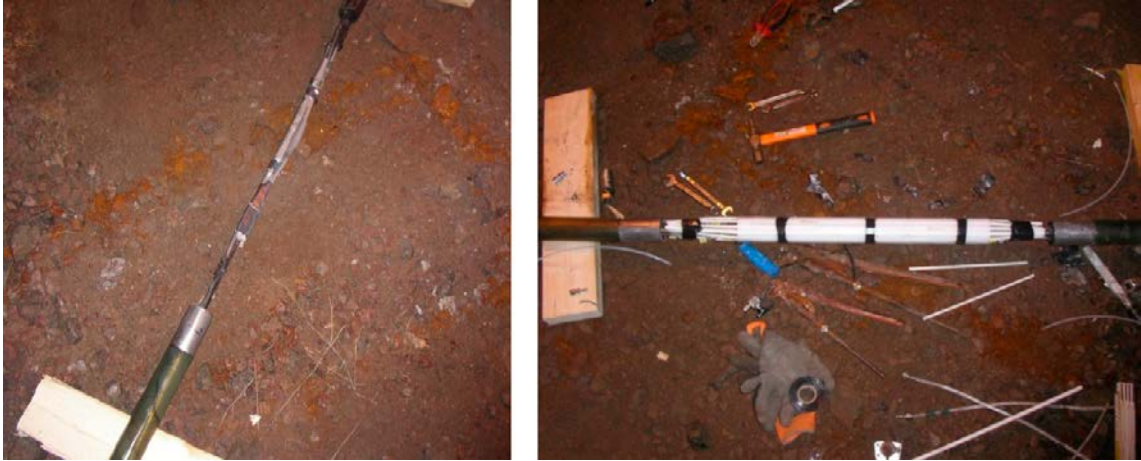
Figure 3-2. The left photograph shows the section between the packers a few minutes after the equipment was removed from the borehole and prior to the dummy installation. The right photograph shows the same section with the dummy installed.
