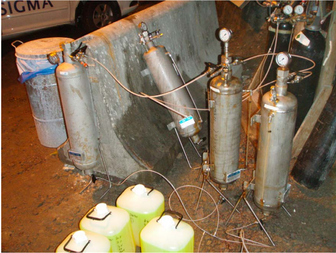
Figure 3-15. Pressurized tracer storage tanks and gas tube ( N_2 ) used for injection of synthetic groundwater during the main SWIW tests (SWIW 4 and SWIW 5).
