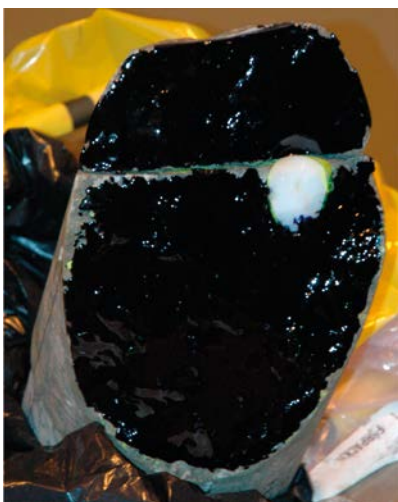
Figure A1-13. KXTT4, Feature A, core piece 1 (Figure A1-11) with core piece 2 (Figure A1-12) on top, as these pieces fit together. The surfaces are in this picture reinforced with a layer of dark blue epoxy. This is made before further cutting to keep the surfaces intact.
