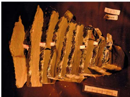
Figure A2-9. Core piece 33. Slices 33.1 to 33.9 and on the upper picture a broken corner also is shown. Slices 33.1 to 33.6 has been cut into rods for Cs analysis.
