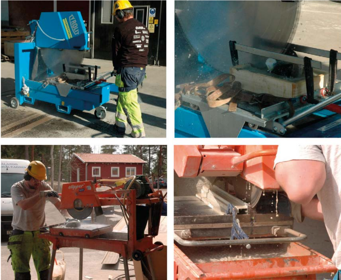
Figure 3-2. The cutting of core pieces from KXTT3 into slices and rods.
