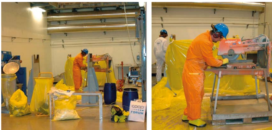
Figure 3-4. The cutting of core pieces in KXTT4 into slices and rods. This was made in a controlled area at CLAB (intermediate storage for radioactive waste) since the drill core displayed a radiation level above the criteria for free handling.
