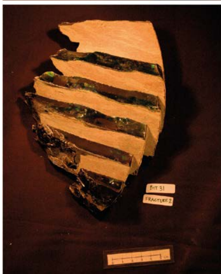
Figure A2-7. Core piece and fracture plane 31 Fracture 2. Slices 31.1 to 31.6. Slice 31.5 has been cut into rods for Cs analysis.
