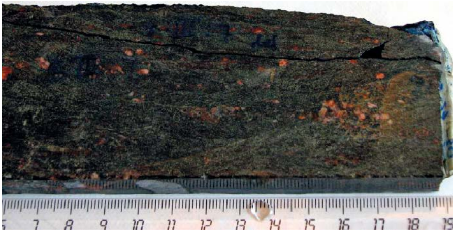
Figure 6-58. Photograph of 8:III:7 (KXTT4), with the open fracture (Feature A') in the upper part of the sample. Black parts are epoxy attached to the fracture surface after drilling.
