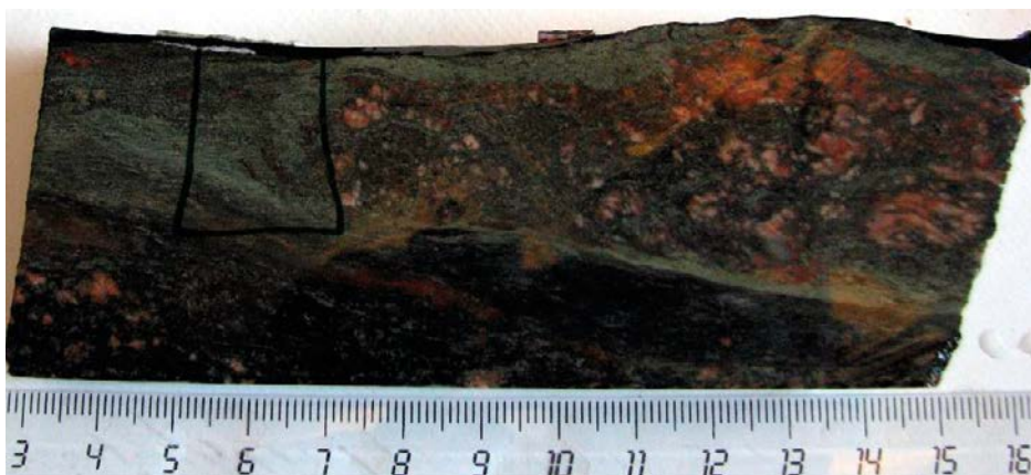
Figure 6-68. Photograph of 11:III:4 (KXTT4), with the open fracture (Feature A') in the upper part of the sample. The location of the thin section is indicated by the markings. Black parts have been epoxy-impregnated after drilling.
