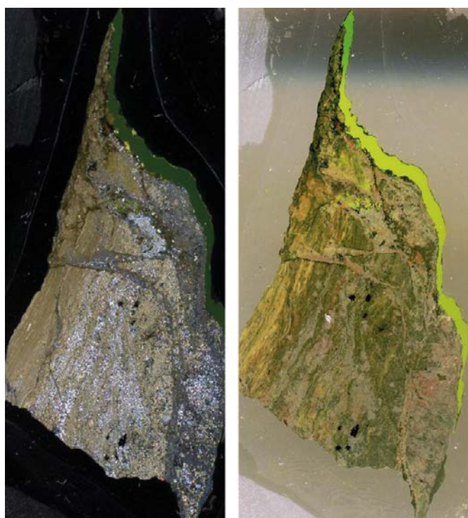
Figure 6-35. Scanned thin section from sample 31-fracture 2, KXTT3 (left: crossed polars; right: plane polarised light). Epoxy (green-yellow) is preferentially found as an outermost layer on the fracture surface in the upper part of the thin section. Width of each image is ~2 cm.
