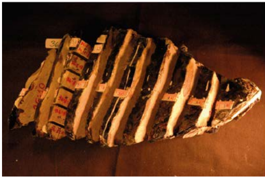
Figure A2-10. Core piece 36. Slices 36.1 to 36.10 and on the upper picture a broken corner also is shown. Slice 36.8 has been cut into rods for Cs analysis.
