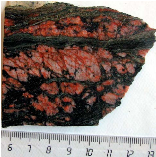
Figure 6-41. Photograph of 1:I:0 (KXTT4), with the open fracture (Feature A) in the upper part of the sample.
