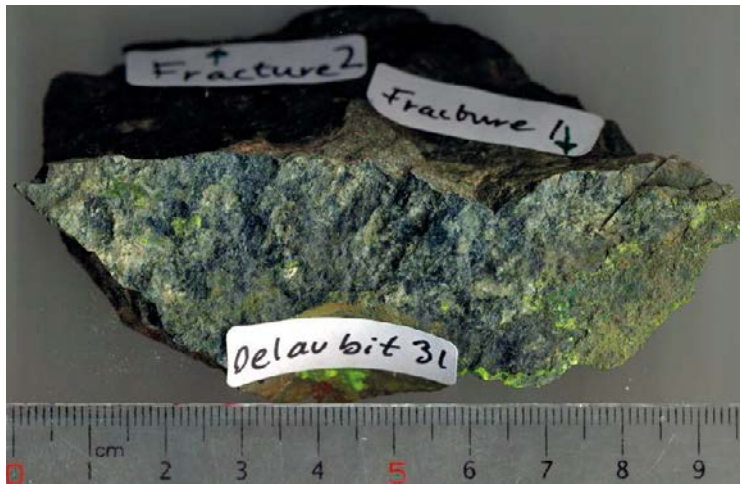
Figure 6-16. Scan of fracture surface of Fracture 1, part of piece 31, KXTT3.
