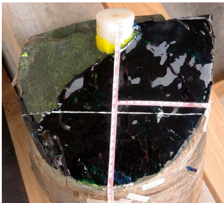
Figure 3-1. KXTT3, core piece 15 with reinforced surface and measurements tapes were added as reference lines before cutting.
