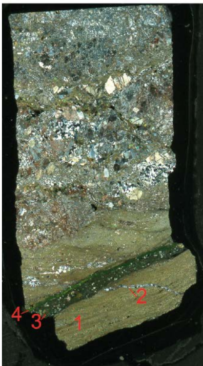
Figure 6-9. Scanned thin section from sample 26, KXTT3 (left: crossed polars; right: plane polarised light). Epoxy (green-yellow) is preferentially found in a fracture in the bottom part of the thin section. Numbers refer to the order of formation (see list below) Width of each image is ~2 cm.
