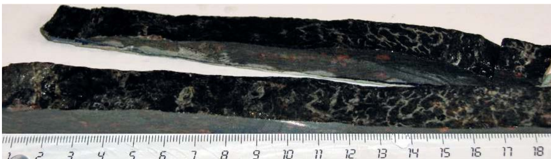
Figure 6-59. Photograph of 8:III:7 (KXTT4), showing both of the fracture surfaces of the fracture parallel to the open Feature A' fracture.
