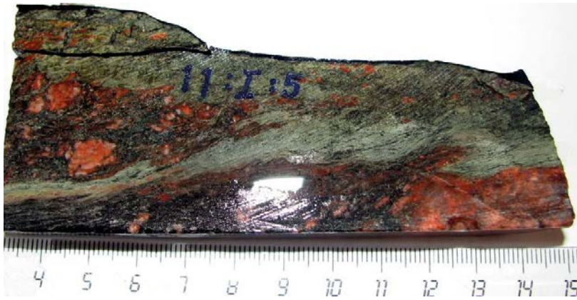
Figure 6-65. Photograph of sample 11:I:5 (KXTT4), with the open fracture (Feature A') in the upper part of the sample. Black parts have been epoxy-impregnated after drilling.
