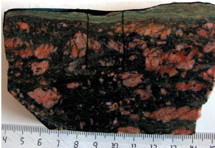
Figure 6-48. Photograph of 2:5 (KXTT4), with the open fracture (Feature A) in the upper part of the sample. The location of the thin section is indicated by the markings.
