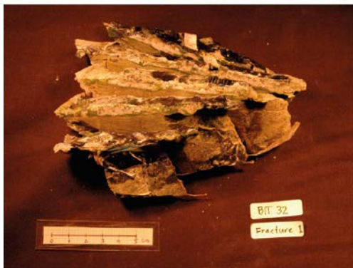
Figure A2-8. Core piece 32. Slices 32.1 to 32.5, Slice 32.3 has been cut into rods for Cs analysis.
