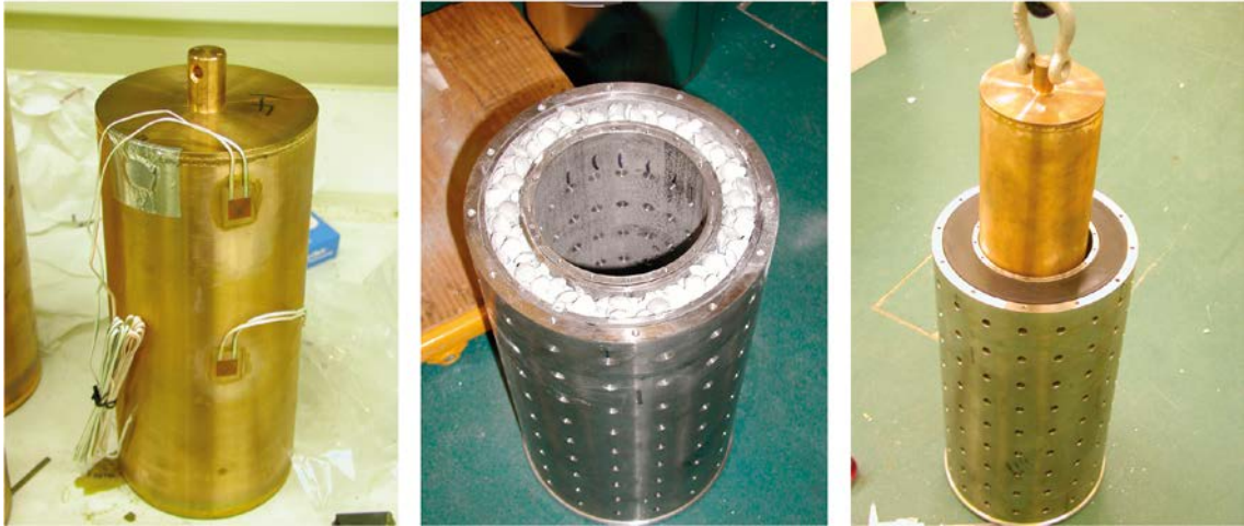
Figure 2-3. Left: Strain gauges mounted on model canister; Centre: Positioning of bentonite pellets inside annulus of support cage; Right: insertion of model canister assembly into support cage.
