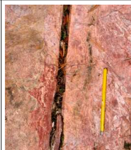
Reddish pink protocataclasite at PFM007095, transected by fractures and a 2 cm thick ultracataclasite (eroded) with orientation 320/88 sub-parallel to the orientation of the Eckarfjärden deformation zone (after SKB P-06-212).
