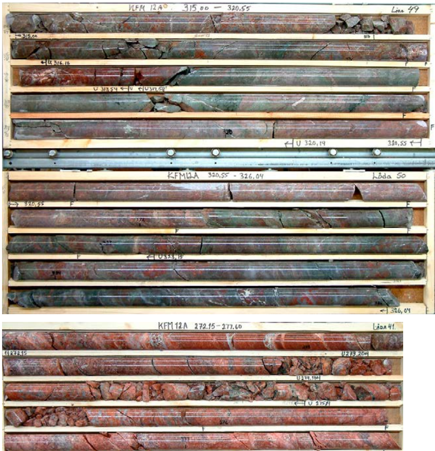
Photographs showing cataclastic rock (upper) and crush rock (lower) along separate fault core intervals. Cohesive fault breccia is also present in the lower photograph (after SKB P-07-111)
