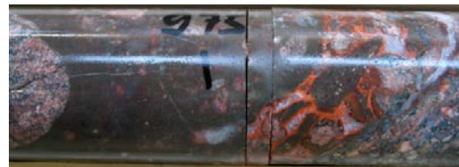
Cataclasite along strong tectonic foliation. The cataclasite is post-dated in its footwall (to the right) by a network of quartz-, laumontite- and calcite-filled fractures. Picture provides evidence for multiple reactivation along the ductile fabric (after P-06-212)
