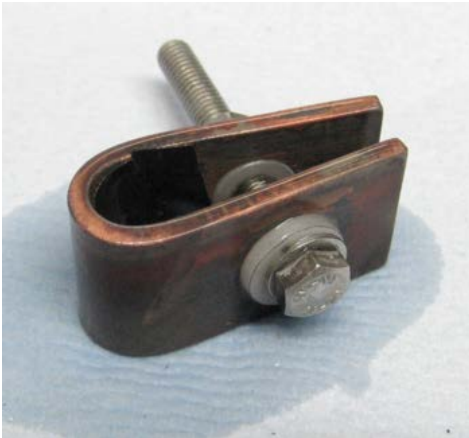
Figure 3-39. U-bend specimen 94UG immediately after removal from the water-filled transfer flask when the specimens were transported to the UK for analysis (Smart et al. 2012).
