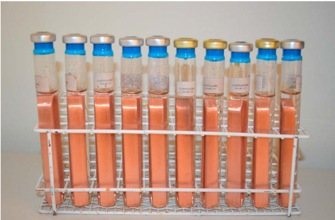
*Figure 4-11. Image of N2 vials after 846 days. N2:1 to N2:10 are shown from left to right.*
