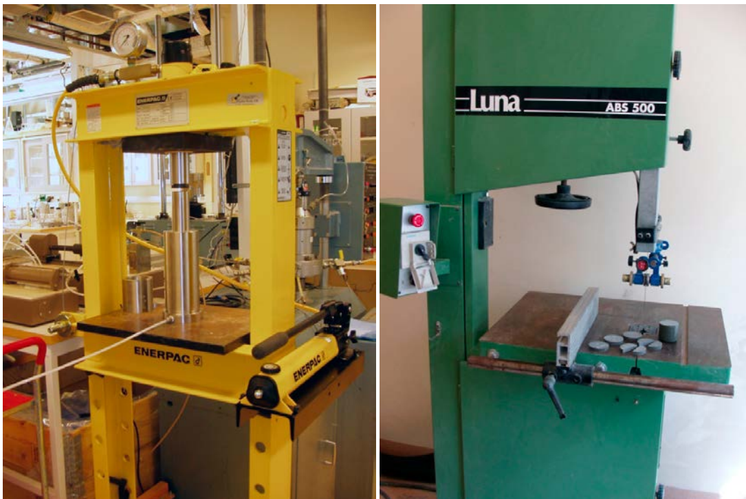
Figure 7-2. The Enerpac VLP256 P392 ram (left) and the Luna ABS 500 band saw with a partly cut sample (right).
