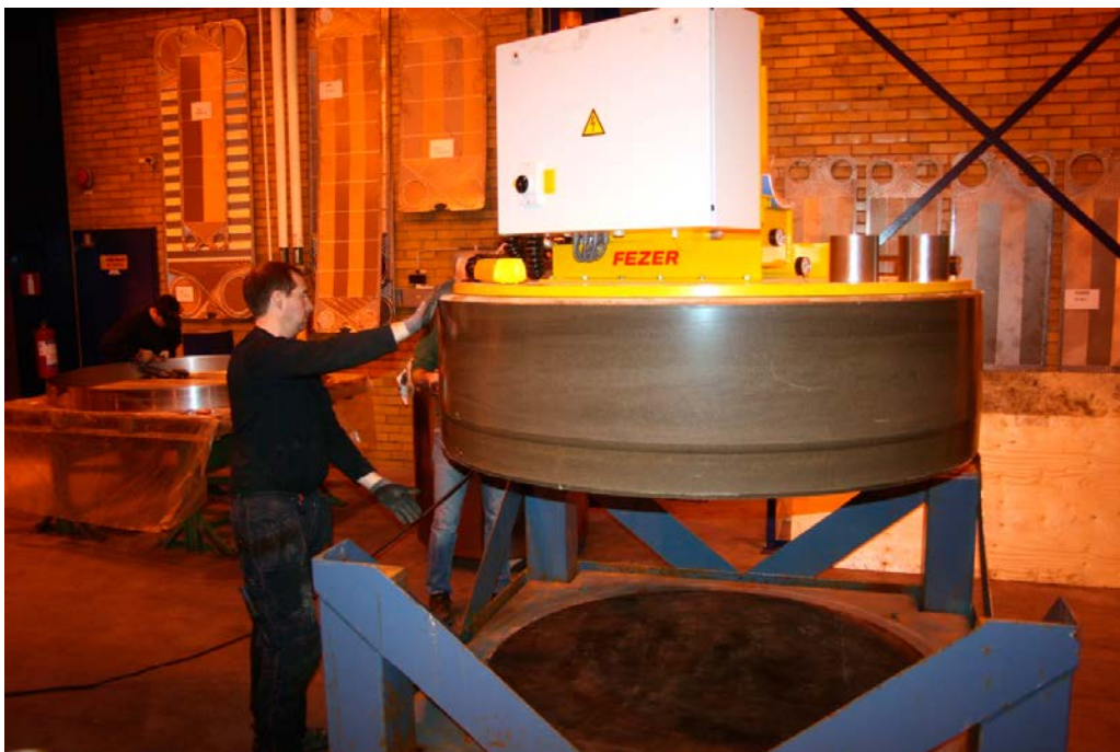
Figure 5-5. Vacuum lifting tool during test production of buffer blocks.
