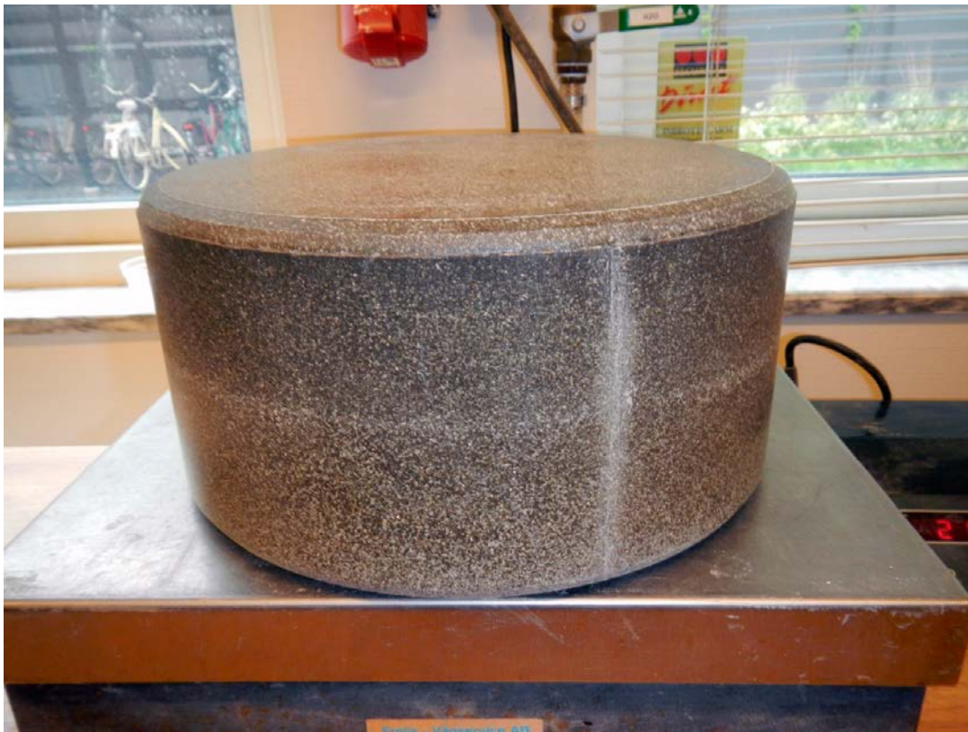
Figure 7-17. Scale block with 300mm in diameter produced with prototype cylindrical mould and no lubricants.
