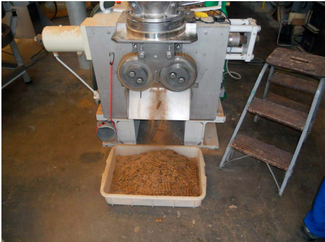
Figure 5-9. Roller compaction of bentonite in a Hosakawa GS-25.
