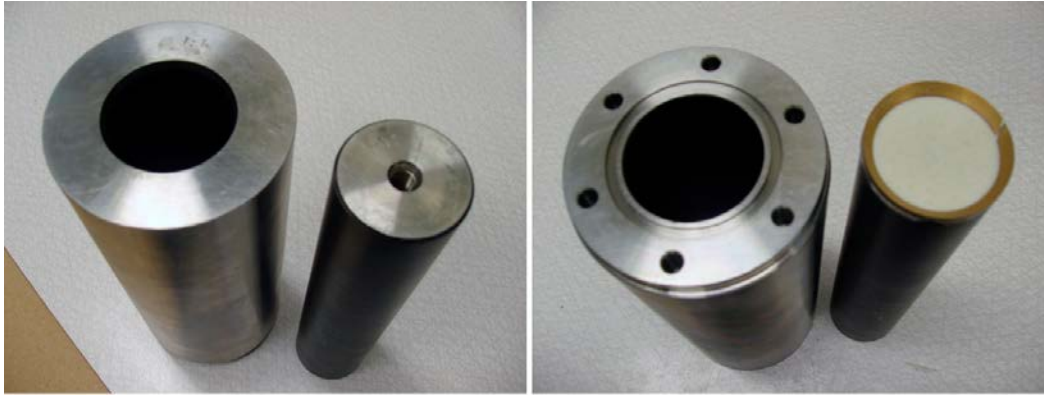
Figure 7-1. The mould and piston (left), and the same mould upside-down together with the filter and copper sealing ring on top of the piston (right).
