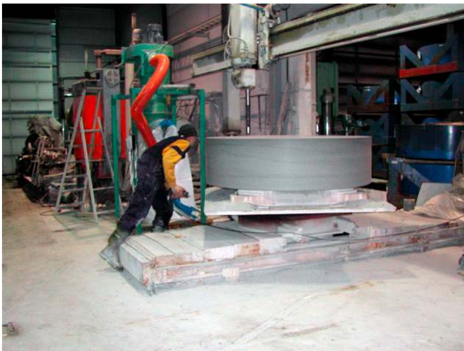
Figure 5-8. Milling of blocks during test production. In the real production the machine needs to be encapsulated and the relative humidity in the encapsulation controlled.
