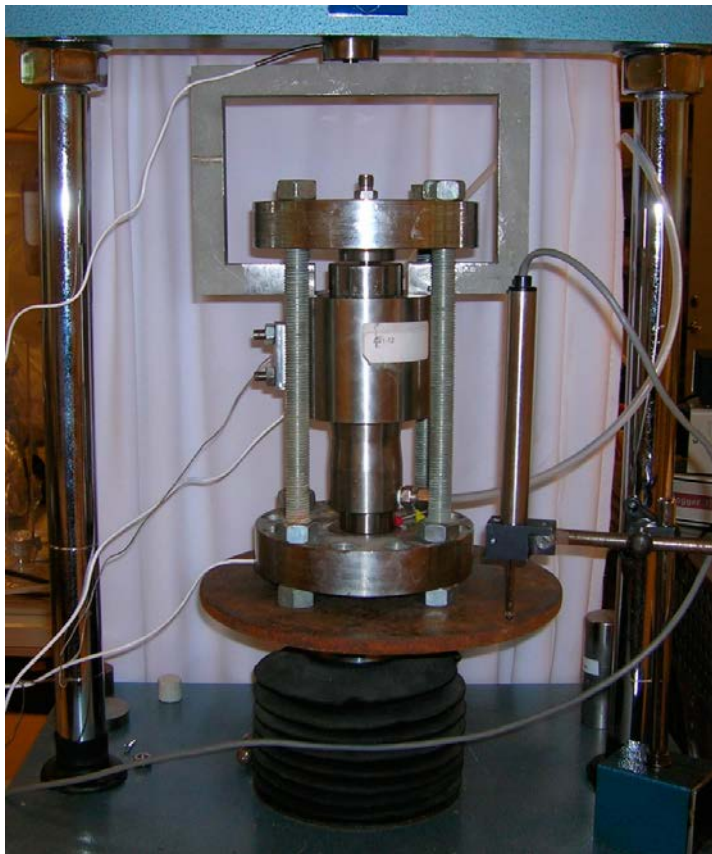
Figure 4-9. Photo of the set-up during the shearing phase of the test.
