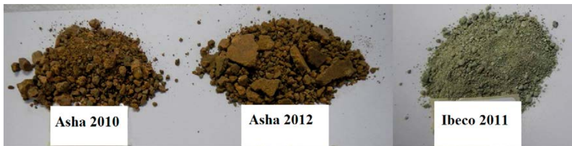
Figure 3-1. Photo showing the different bentonite materials tested.
