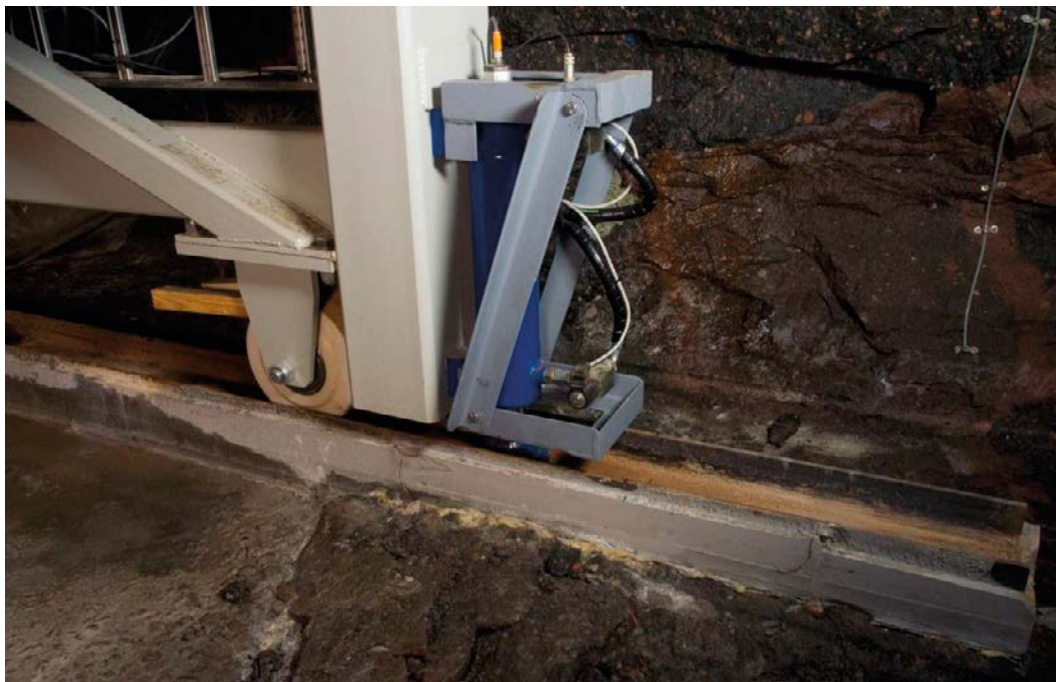
Figure 8-2. The robot platform was operated and moved using temporary guide rails.
