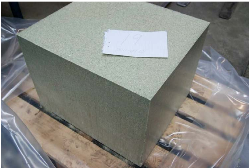
Figure 5-2. Photo showing one of the best Ibeco blocks manufactured.
