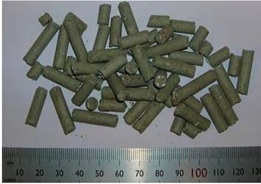
Figure 4-1. 6 mm extruded pellets of Ibeco material.
