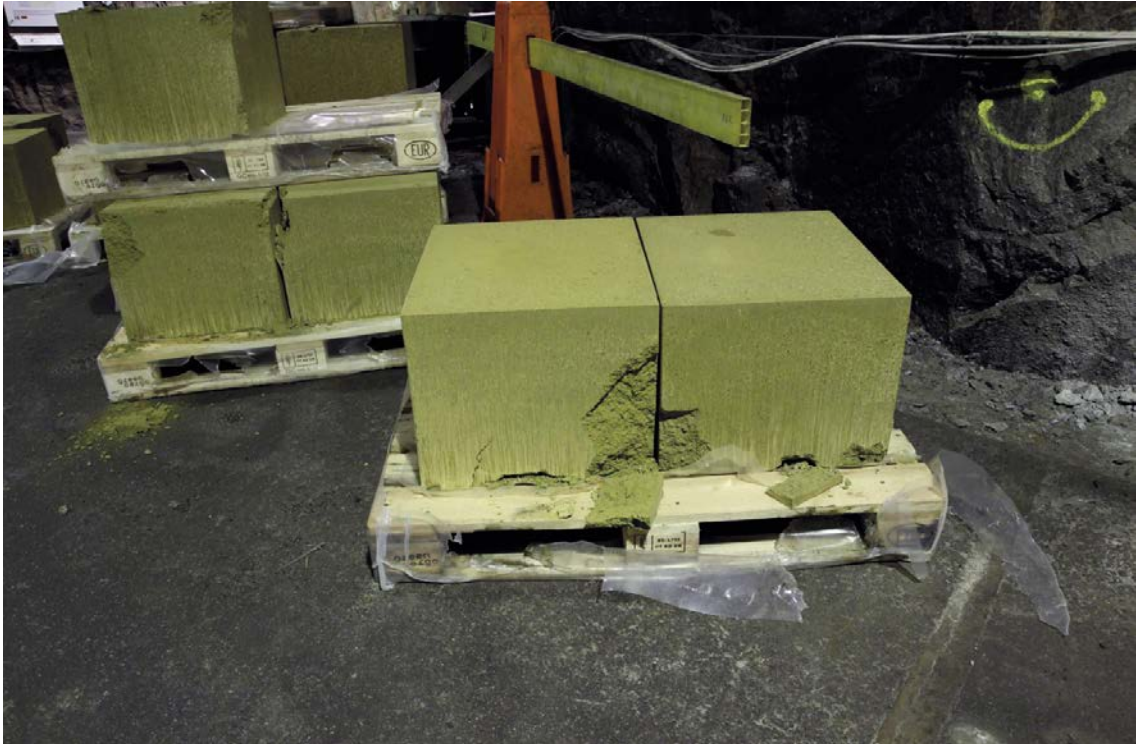
Figure 8-8. Examples of backfill blocks rejected due to cracks and missing pieces.
