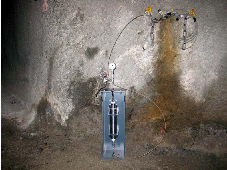
Figure 2-2. A flowcell connected to borehole ONK-PVA8, for biofilm enrichment in the ONKALO tunnel, Finland.
