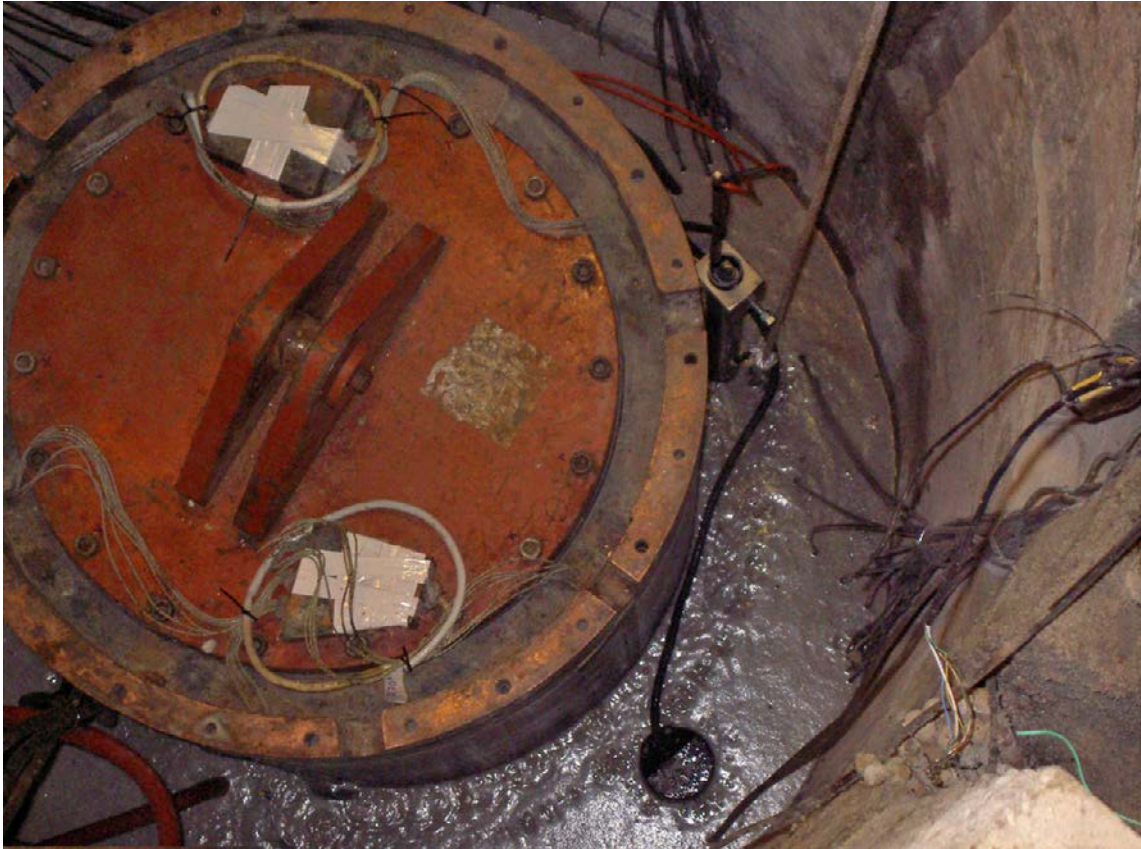
Figure 5-5. The buffer disintegration system in operation. The canister is visible to the left.
