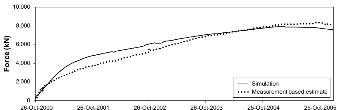
Figure 4-9. Simulated and measurement based estimate of vertical force on the plug.
