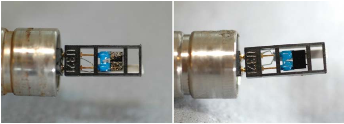
Figure D-1. Vaisala Sensor membrane, exposed W204 and new.
