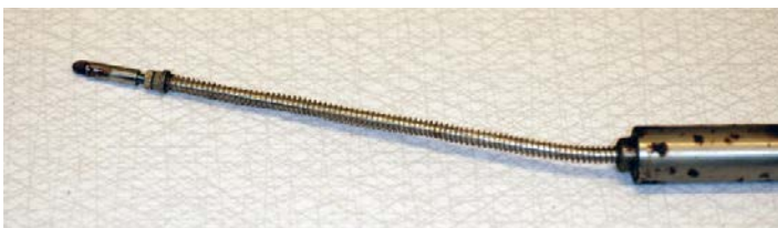
Figure D-5. Bent displacement sensor 3.
