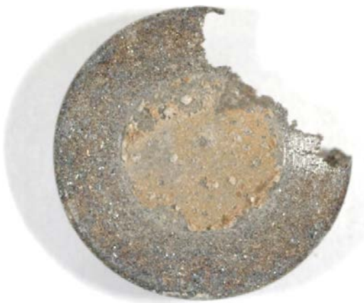
Figure D-2. Wescor filter (W214), the damage on the rim occurred when the filter was removed from the holder.
