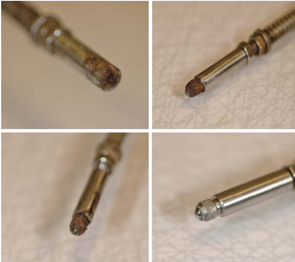
Figure D-3. Top row, tip of sensor 1 and 2, Bottom row tip of sensor 3 and a new tip.
