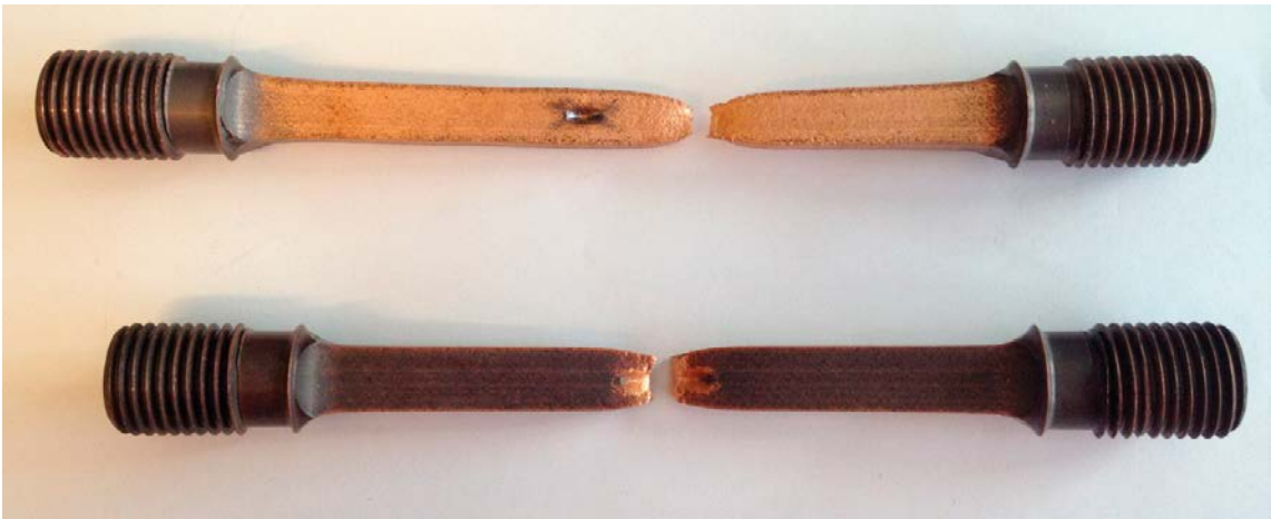
Figure 3-16. Image showing the distance from fracture to indentation. Over: SKB 2-4, under: SKB 2A-4.
