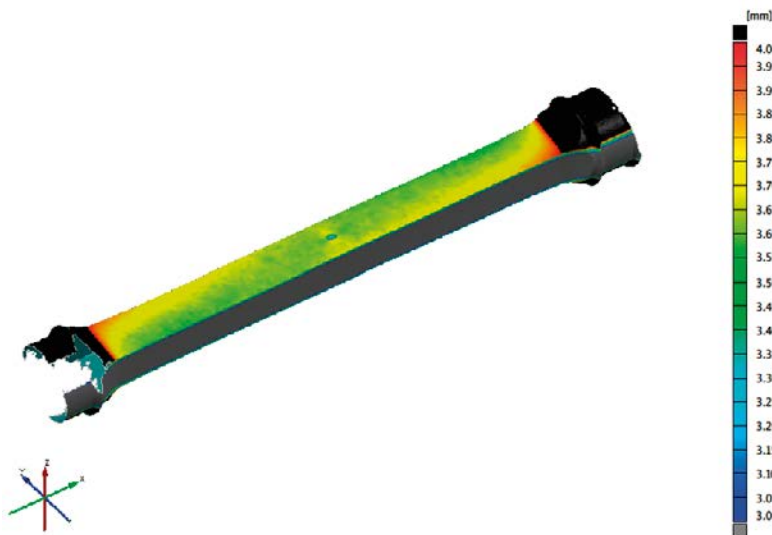
Figure 3-19. SKB 2A-1, annealed 2 mm indentation then annealed again.
