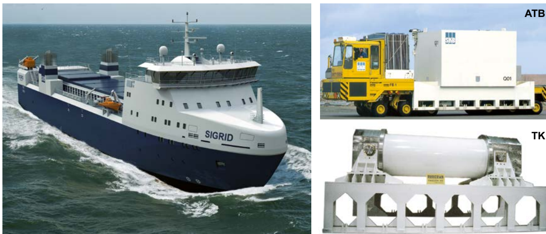
Figure 3-6. M/S Sigrid and transport casks for short-lived radioactive waste (ATB) and for core components (TK).
