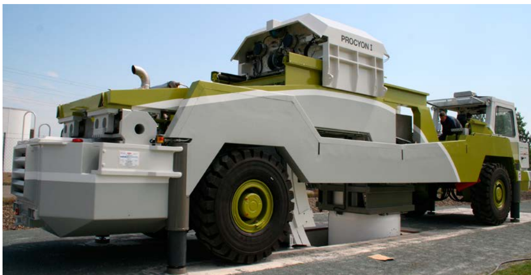
Figure 3-8. Deposition machine for handling canisters in the repository
