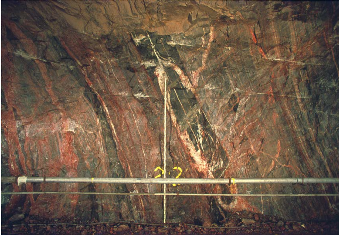
Figure A-2. Brecciated metagranite within the Singö Deformation Zone with numerous veins of quartz and calcite, Forsmark 1 and 2 tunnel (Carlsson and Olsson 1977, Carlsson and Christiansson 2007, Figure 4-4).
