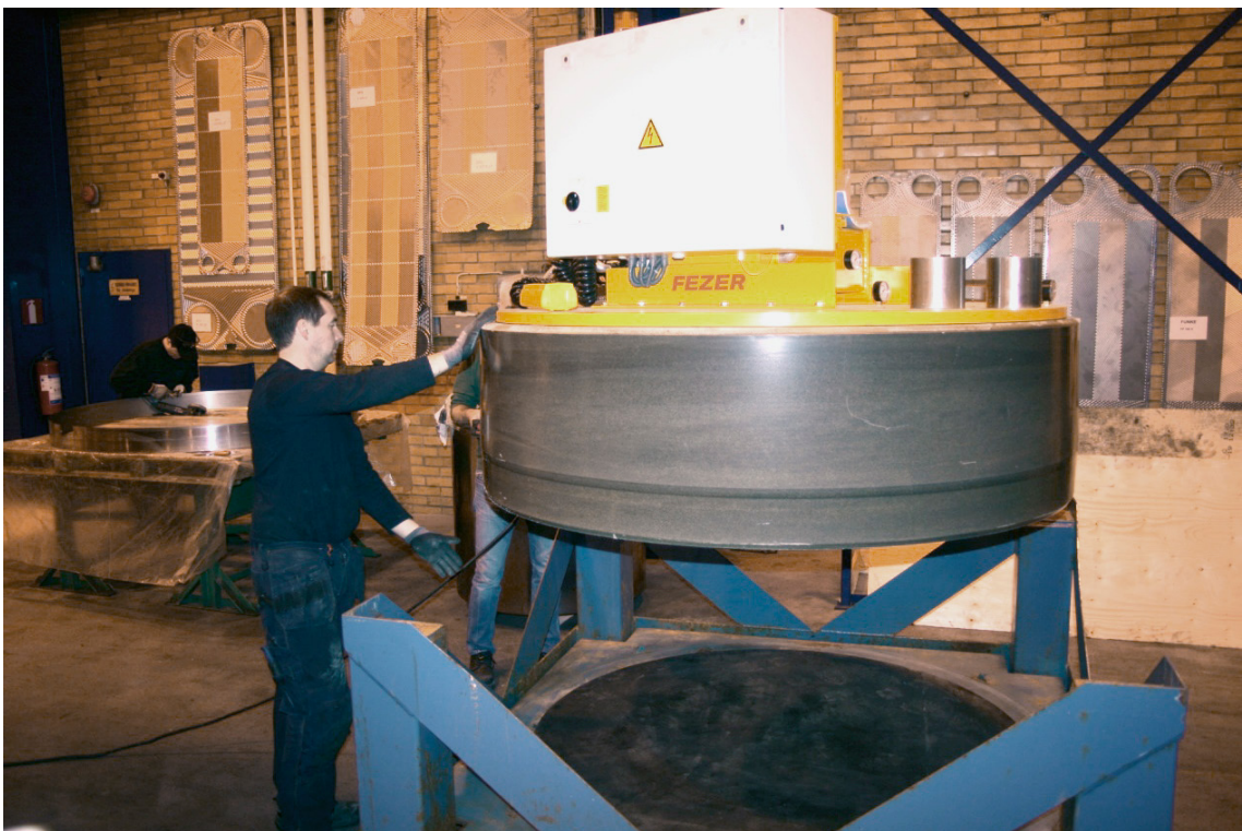
Figure 4-4. The bentonite block lifted with the vacuum oak and placed on the special designed pallet.
