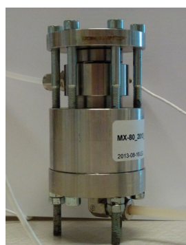
Figure 2-8. A picture and a schematic drawing of the swelling pressure device.
