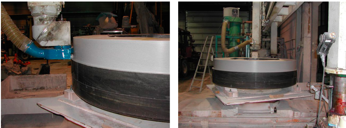
Figure 6-1. The bentonite block machined with a milling machine.
