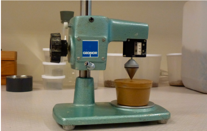
Figure 2-4. The cone apparatus used for determining the liquid limit of the bentonite.
