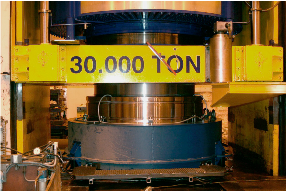
Figure 4-2. The mould placed in the press.
