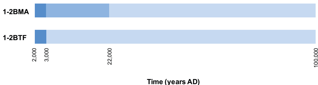
Figure 7-14. Illustration of succession of the hydraulic conductivity of the concrete in the accelerated concrete degradation scenario where the three colours represents the degradation from moderately via severely to completely degraded concrete. Only the waste vaults where the concrete constitutes a main flow barrier are shown. The corresponding figure for the main scenario is Figure 7-8.
